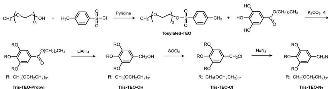
**Figure S2.** Synthesis of azide-terminated hydrophilic dendron (tris-TEO-N<sub>3</sub>).
