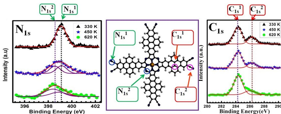
**Figure S2:** XPS core-level measurements of the C and N of HTTN/Au (111) experience a hierarchical on-surface reaction driven by thermal treatments.
