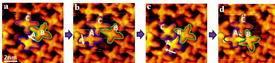
**Figure S1:** The cross-like supramolecular structure can be rotated and moved around on the surface as a whole by STM manipulation. Scanning parameters:  $V_s=1.0\text{V}$  and  $I_s=0.03\text{nA}$ .
