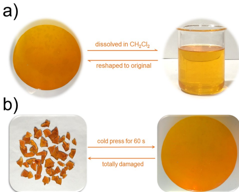
Fig. S18 (a) Recycling procedure of BTA-PDMS-25000 polymer films by dissolving the sample in DCM. (b) Reprocessing of the totally damaged pieces through compression molding at 25 °C and 10 MPa for 60 s.
