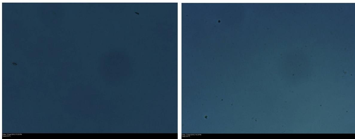
**Fig. S6** Optical microscopic images for the blend surfaces of **W8** (P3HT left and PTB7 right) showing fairly flat surfaces corroborating TEM and XRD analyses.
