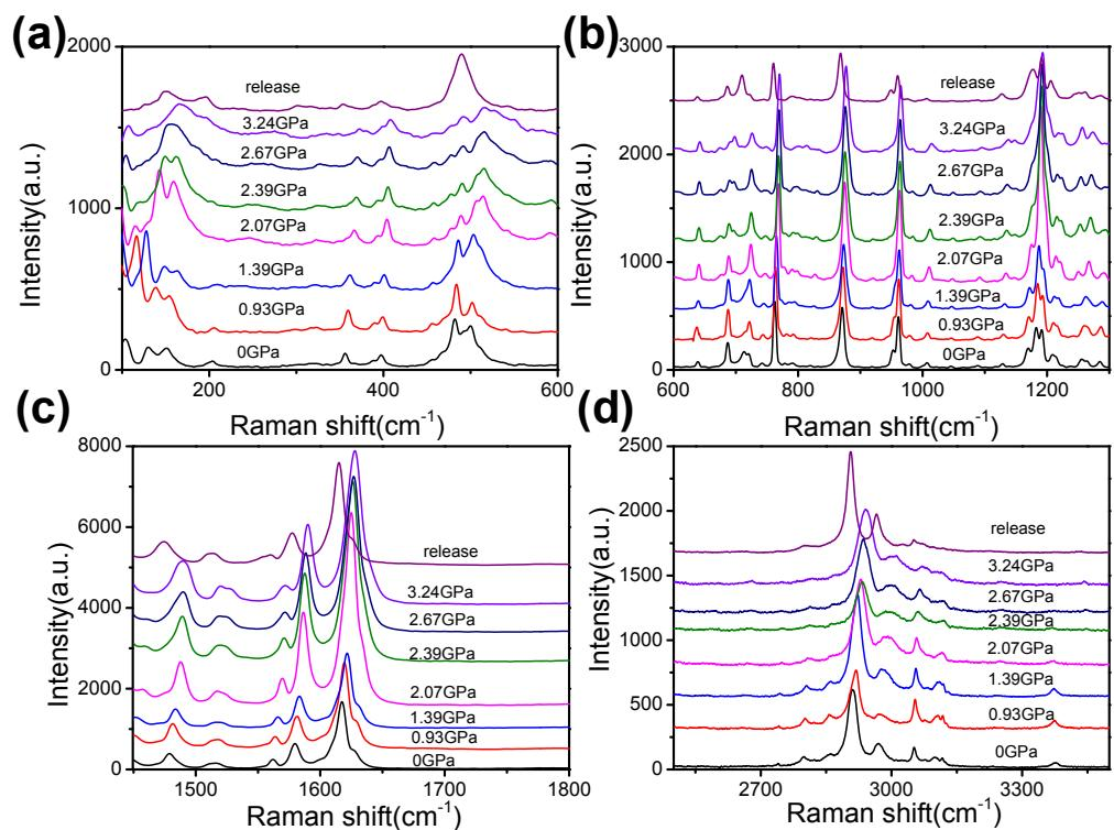
Figure S5. Raman spectra of GC at different pressure values *via* DAC. The excitation wavelength was 633 nm. (a)-(d) 100-600, 600-1320, 1400-1800, and 2400-3500  $\text{cm}^{-1}$ , respectively.
