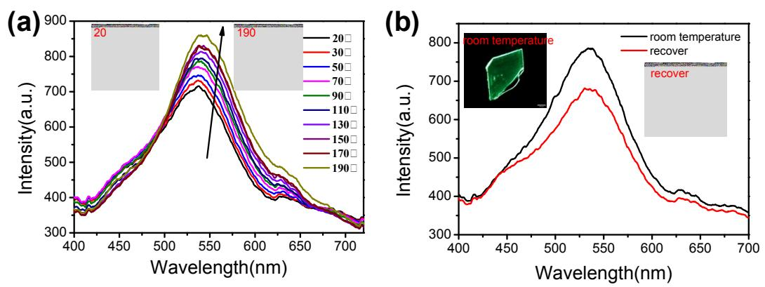
Figure S13. Temperature-dependent fluorescent spectra of GC during 20 °C-190 °C (a) and reversible fluorescence switching with temperature (b).  $\lambda_{\text{ex}} = 375$  nm.
