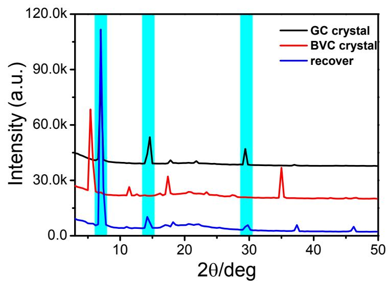
Figure S15. XRD patterns of GC, BVC and the crystal that recovers to room temperature.
