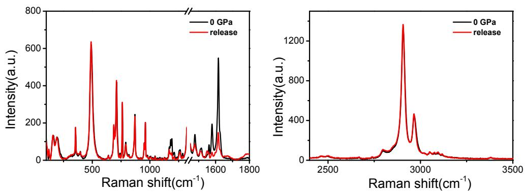
Figure S6. The recovery of the Raman spectra of GC under the excitation of 633 nm. Left panel; 100-1800 cm<sup>-1</sup>. Right panel: 2400-3500 cm<sup>-1</sup>.
