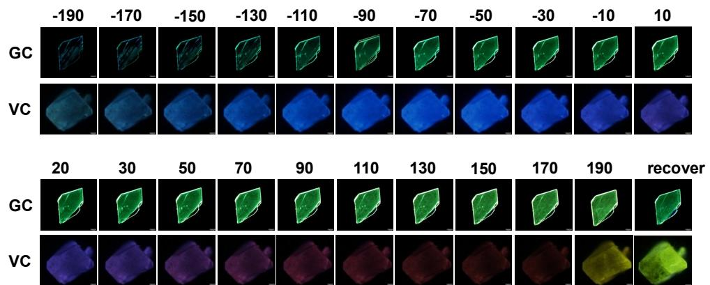
Figure S12. Temperature-dependent fluorescent photos of GC and BVC during -190°C-190 °C.  $\lambda_{\text{ex}} = 375 \text{ nm}$ .
