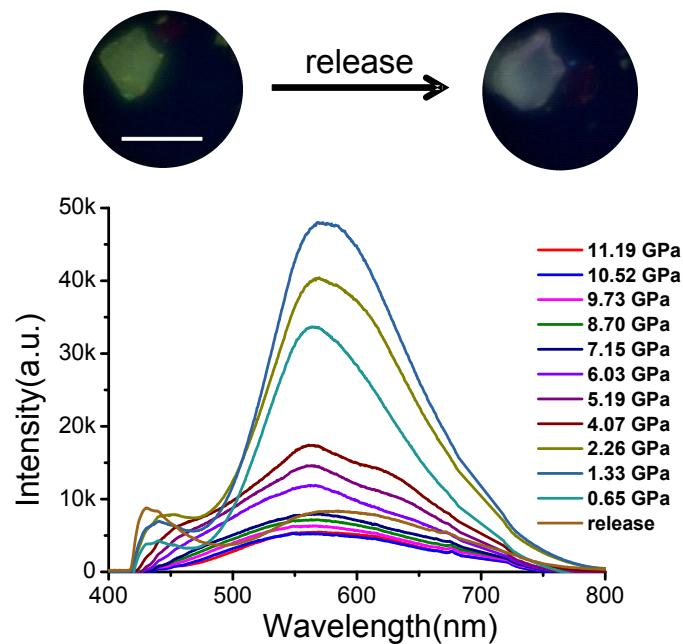
Figure S3. Fluorescent spectra of BVC at different pressure values *via* DAC (a) and the corresponding fluorescent photos (b) during the depressurizing process. Excitation wavelength was 365 nm. The scale is 100  $\mu\text{m}$ .
