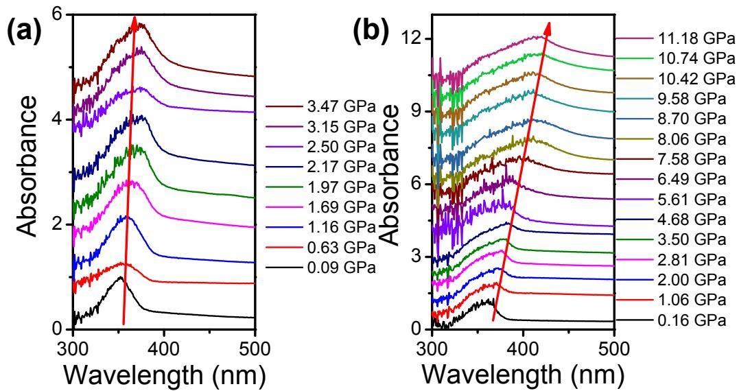
Figure S2. UV-visible absorption spectra of GC (a) and BVC (b) with increasing pressure.
