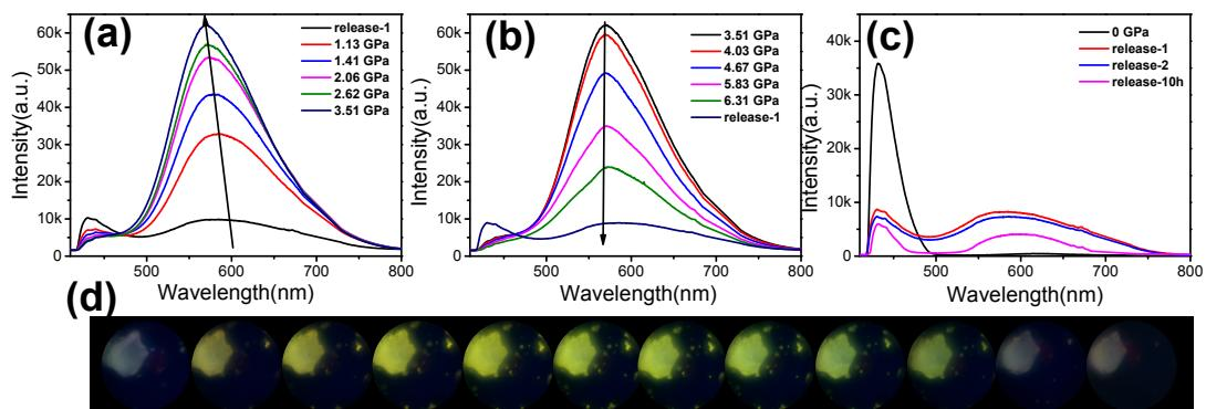
Figure S4. Fluorescent spectra of BVC crystal under the pressure from 0 to 3.61 GPa (a), from 3.61 to 6.31 GPa (b) and recovery (c). (d) Left to right; the photos during the compression under the excitation of 365 nm.
