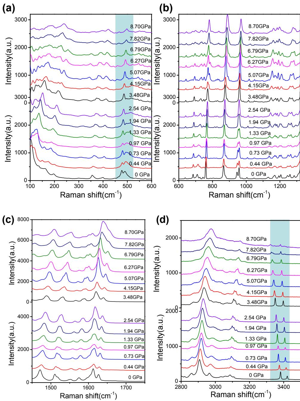
Figure S7. Raman spectra of BVC at different pressure values *via* DAC. Excitation wavelength was 633 nm. (a)-(d) 100-600, 600-1320, 1400-1800, and 2400-3500  $\text{cm}^{-1}$ , respectively.
