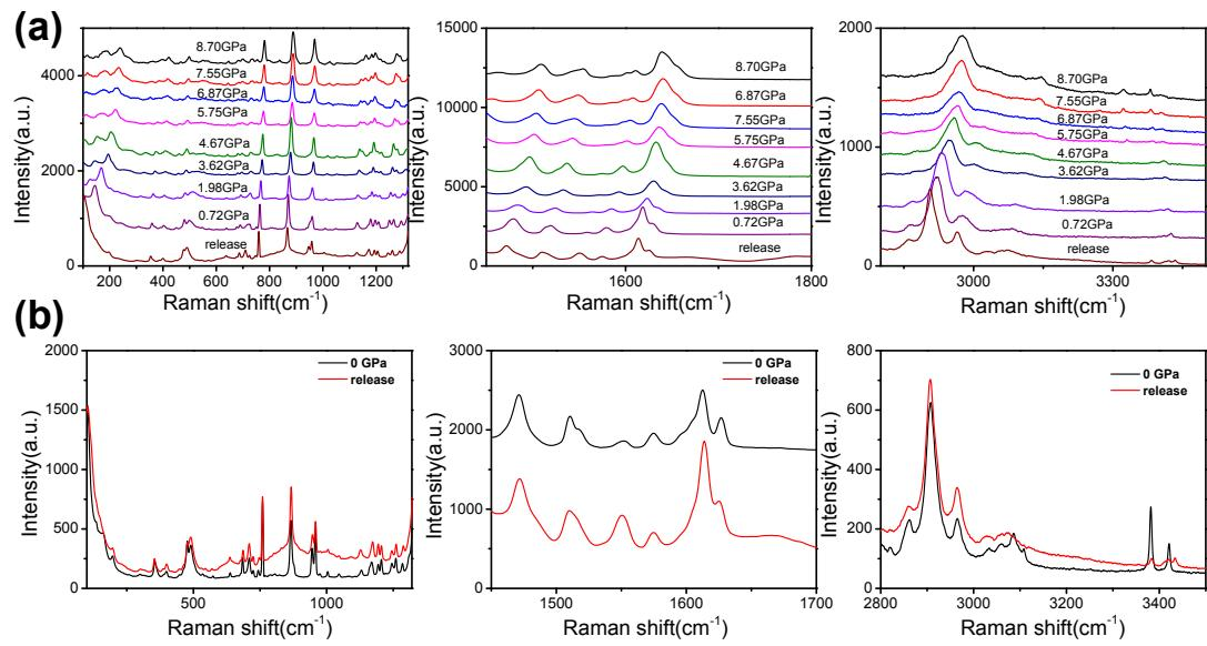
Figure S8. Raman spectra of BVC during the decompression (a) and the recovery properties (b). Excitation wavelength was 633 nm.
