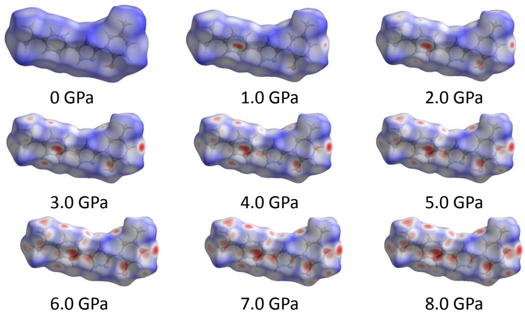
Figure S9. Hirshfeld surfaces of a 4MPP molecule based on a twisted conformation in BVC under different pressures.
