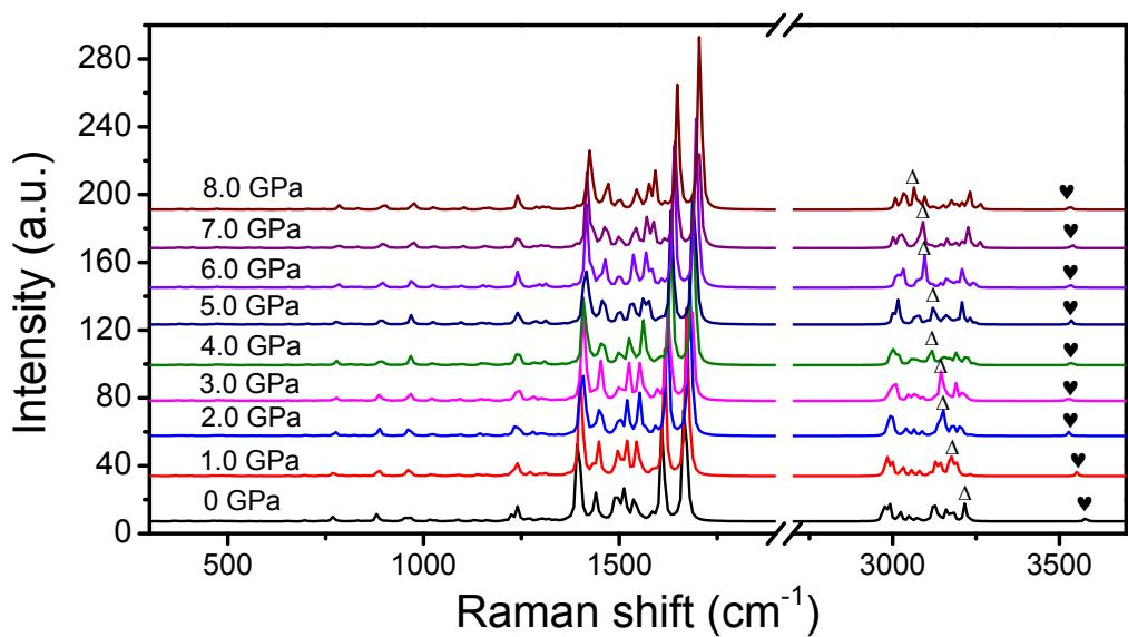
Figure S11. The calculated Raman spectra of a 4MPP molecule based on a twisted conformation in BVC under the external stress of 0, 1.0, 2.0, 3.0, 4.0, 5.0, 6.0, 7.0 and 8.0 Gpa. The symbol “Δ” and “♥” represents the O-H and the N-H stretching vibrational modes, respectively.
