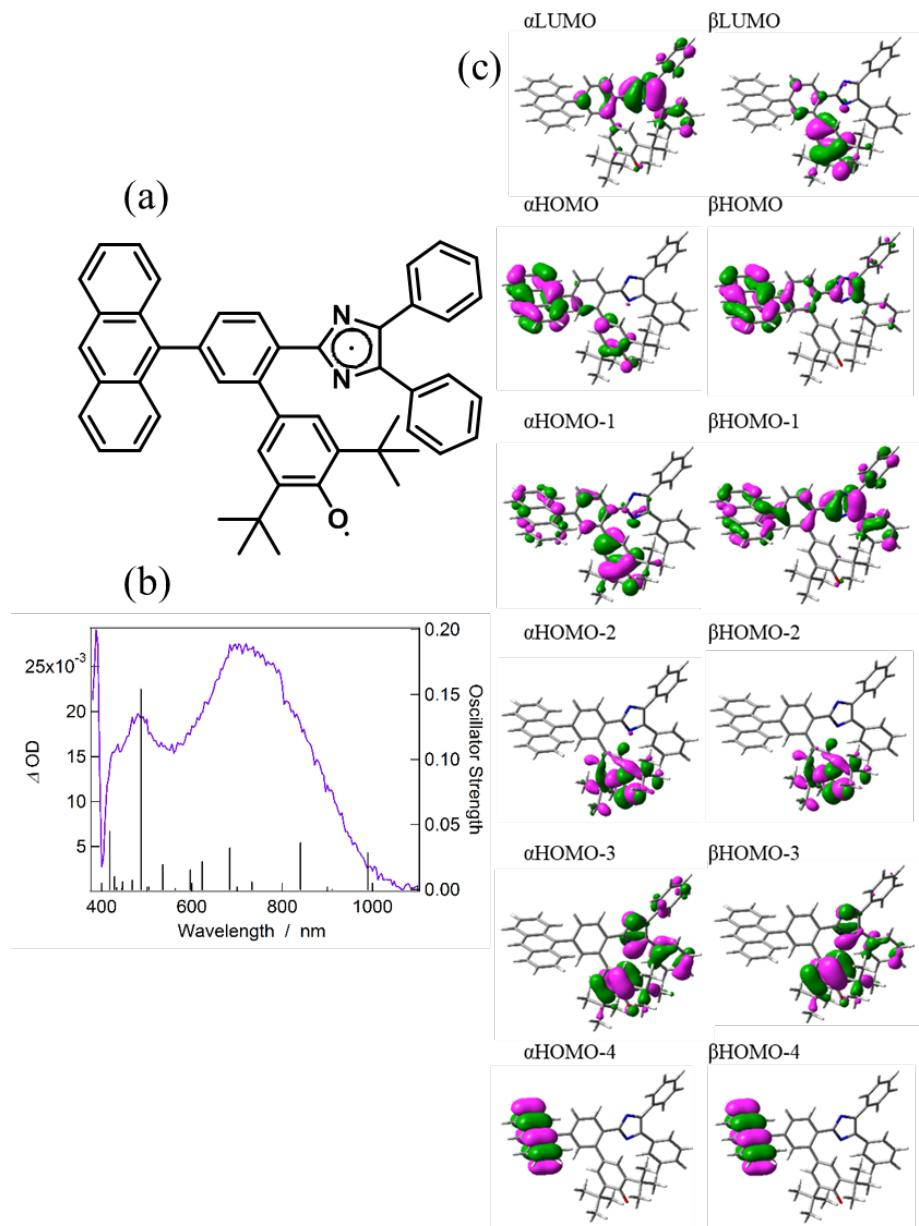
**Figure S42.** (a) Molecular structure of compound **An-PICR**; (b) UV–vis absorption spectrum of **An-PICR**. The calculated spectra are shown by the perpendicular lines. (c) The calculated molecular orbitals of **An-PICR**.
