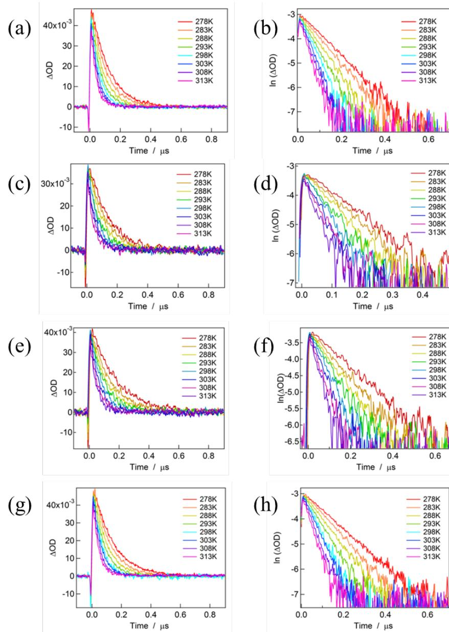
**Figure S44.** (a), (c), (e), (g) Transient absorption spectra and (b), (d), (f), (h) first-order kinetic profiles of the colored species generated from **Ph-PIC**, **Np-PIC**, **An-PIC** and **Py-PIC** in benzene. ( $\lambda_{\text{ex.}} = 355$  nm,  $\lambda_{\text{abs.}} = 700$  nm.  $[\text{Ph-PIC}] = 3.2 \times 10^{-5}$  M,  $[\text{Np-PIC}] = 3.5 \times 10^{-5}$  M,  $[\text{An-PIC}] = 3.1 \times 10^{-5}$  M,  $[\text{Py-PIC}] = 3.3 \times 10^{-5}$  M, power density 4.2 mJ).
