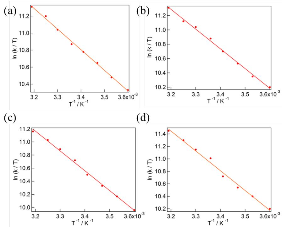
**Figure S45.** Eyring plot for the thermal back-reaction of colored species of **Ph-PIC**, **Np-PIC**, **An-PIC**, **Py-PIC** in benzene.
