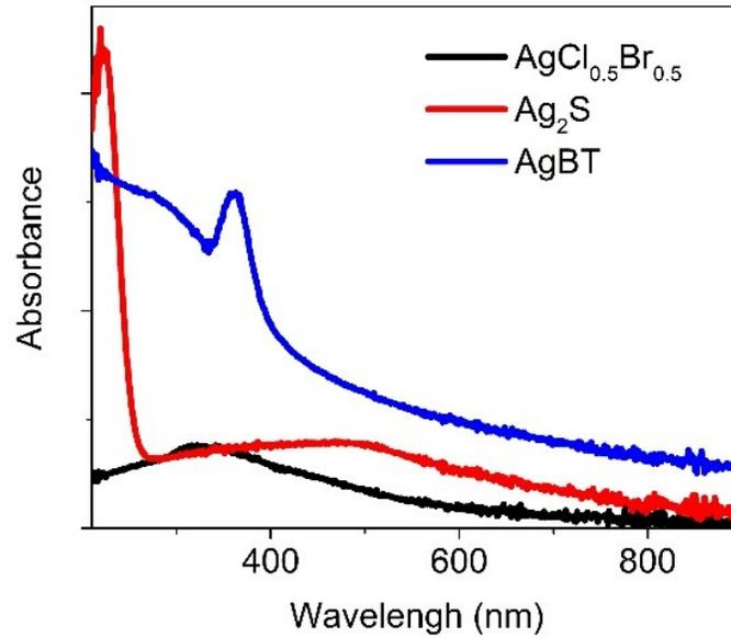
**Fig. S5** UV-visible absorption spectra of dispersions of  $\text{AgCl}_{0.5}\text{Br}_{0.5}$  nanocubes (black), hollow  $\text{Ag}_2\text{S}$  nanoshells (red), and hollow AgBT nanoshells (blue).
