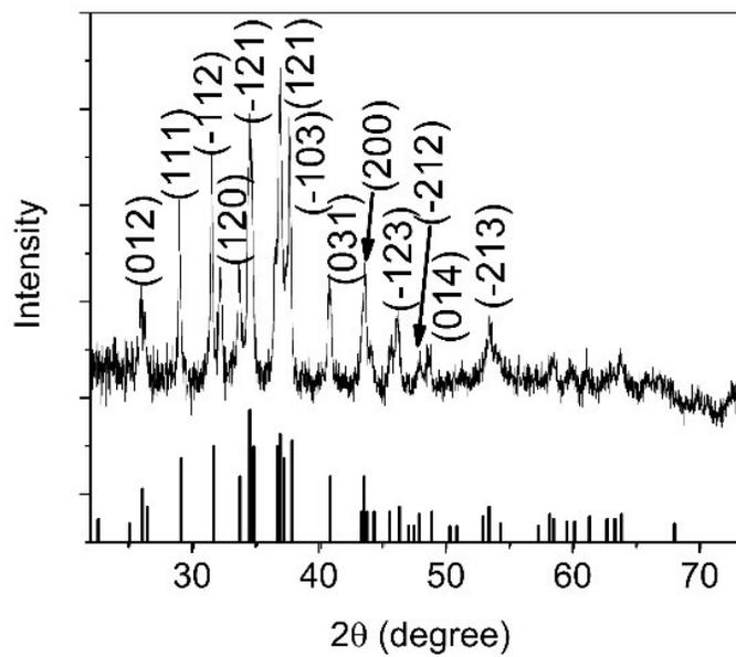
**Fig. S6** XRD pattern of freestanding  $\text{Ag}_2\text{S}$  nanoparticles that were used as control experiment of photocatalysis.
