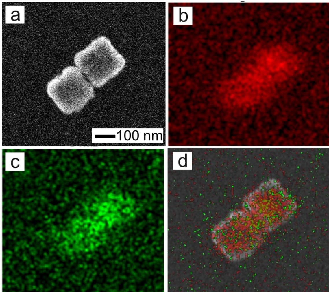
**Fig. S3** (a) SEM image of hollow Ag<sub>2</sub>S nanoshells, EDS element mapping of both (b) Ag (red), (c) S (green), and (d) the overlay of Ag and S spectra on the SEM image.
