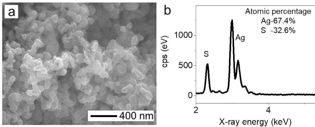
**Fig. S7** (a) SEM image and (b) EDS element analysis of the  $\text{Ag}_2\text{S}$  nanoparticles after the use in photocatalytic reaction. The result of EDS analysis indicates that the atomic ratio of Ag to S still maintained at 2:1, consistent with the stoichiometric composition of  $\text{Ag}_2\text{S}$ .
