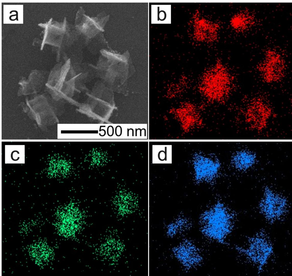
**Fig. S4** (a) SEM image of hollow AgBT nanoshells and the corresponding EDS element mapping of individual elements: (b) Ag, (c) S, and (d) C.
