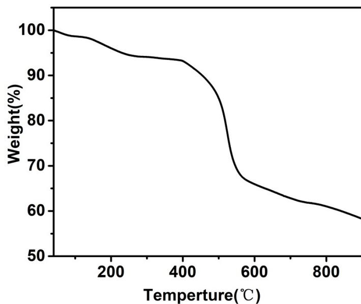
**Figure S3.** The TGA of UPC-50.
