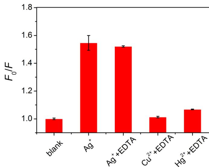
Fig. S7. Fluorescence changes of the probe towards  $Ag^+$ , the mixture of  $Ag^+$  and EDTA, the mixture of  $Cu^{2+}$  and EDTA, the mixture of  $Hg^{2+}$  and EDTA. (The concentration of the N-dots was  $100 \mu\text{g/mL}$ . The concentration of the  $Ag^+$  was  $2 \mu\text{M}$ . The concentrations of  $Cu^{2+}$  and  $Hg^{2+}$  were  $20 \mu\text{M}$ . The concentration of EDTA was  $100 \mu\text{M}$ .)
