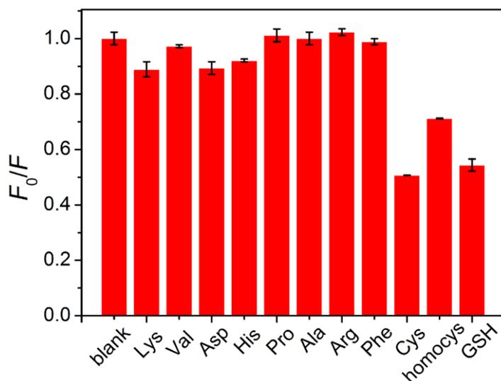
Fig. S10. Selectivity of the N-dots/Ag<sup>+</sup> complex toward Cys. (The concentrations of the N-dots and Ag<sup>+</sup> were 100 μg/mL and 2 μM, respectively. 4 μM for Cys, Hcy and GSH. 100 μM for other cations)
