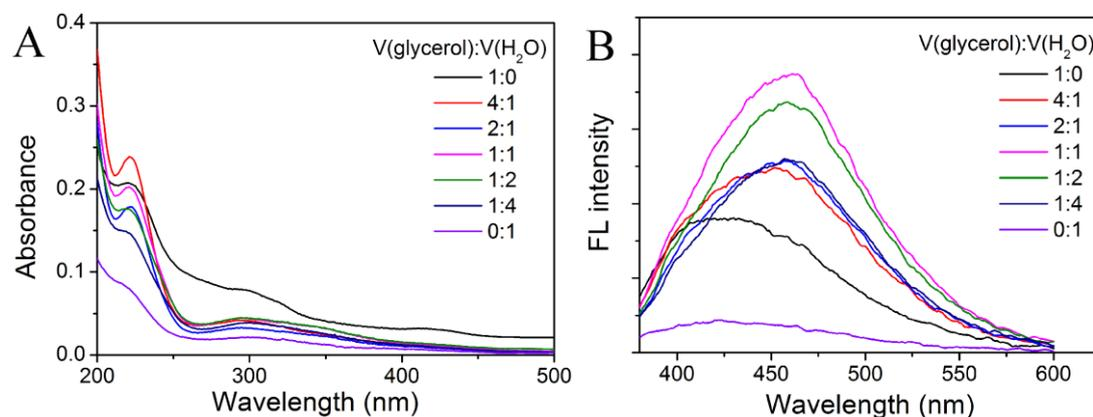
Fig. S2. The UV-vis spectra (A) and fluorescence emission spectra (B) of the N-dots synthesized at different concentrations of glycerol.
