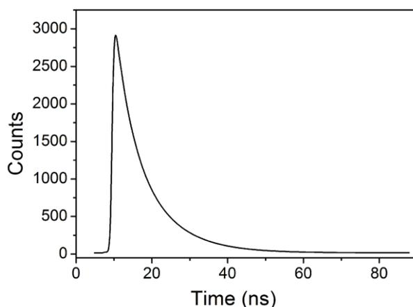
Fig. S5. The fluorescence lifetime spectrum of the N-dots (The concentration of the N-dots was 100  $\mu\text{g/mL}$ ).
