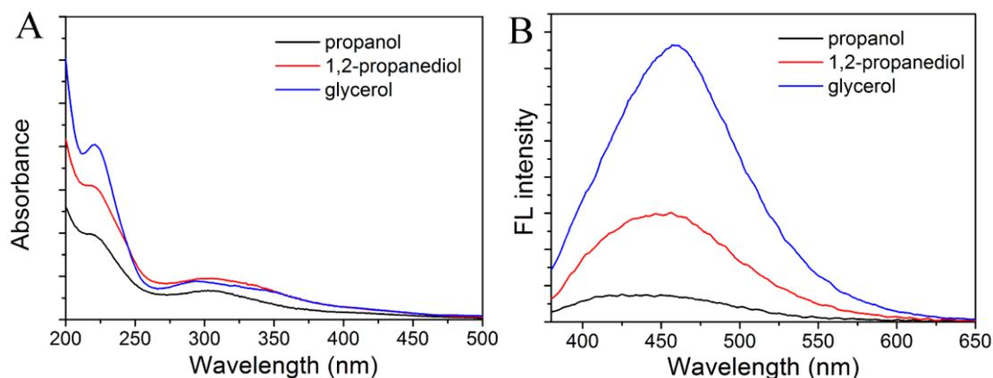
Fig. S1. The UV-vis spectra (A) and fluorescence emission spectra (B) of the nitrogen-rich CDs (N-dots) synthesized with different hydroxyl compounds as additives.
