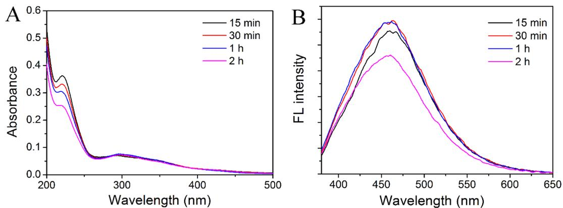
Fig. S4. The UV-vis spectra (A) and fluorescence emission spectra (B) of the N-dots synthesized at different reaction time with glycerol
