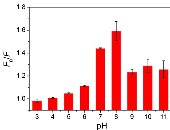
Fig. S6. pH Effect on  $\text{Ag}^+$  detection based on the fluorescence quenching efficiency ( $F_0/F$ ) (The concentrations of the N-dots and  $\text{Ag}^+$  were 100  $\mu\text{g/mL}$  and 2  $\mu\text{M}$ , respectively).
