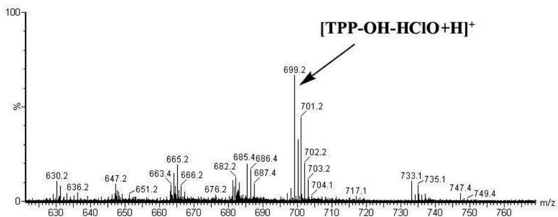
**Figure S14.** The mass spectrum of TPP-OH-HClO (m/z 699.2  $[\text{M}+\text{H}]^+$ ).
