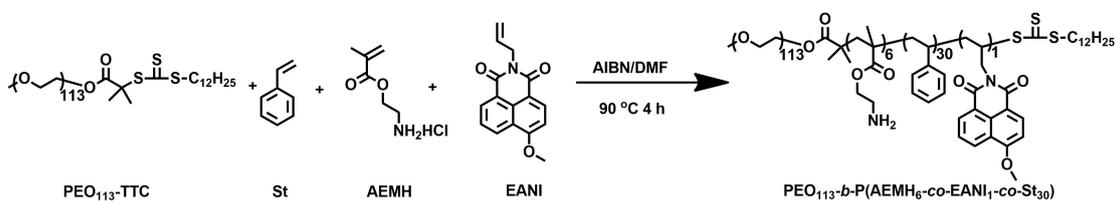
**Scheme S2.** Synthesis route of PEO<sub>113</sub>-*b*-P(AEMH<sub>6</sub>-*co*-EANI<sub>1</sub>-*co*-St<sub>30</sub>).
