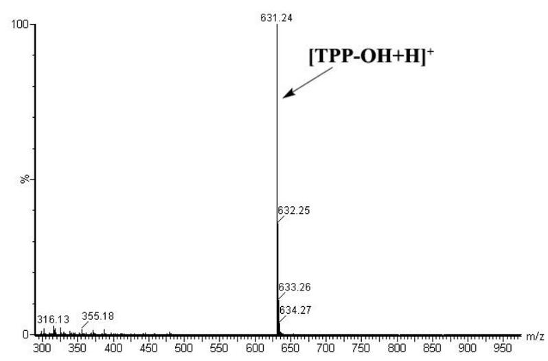
Figure S2. Mass spectrum of TPP-OH ( $m/z$  631.24  $[\text{M}+\text{H}]^+$ ).
