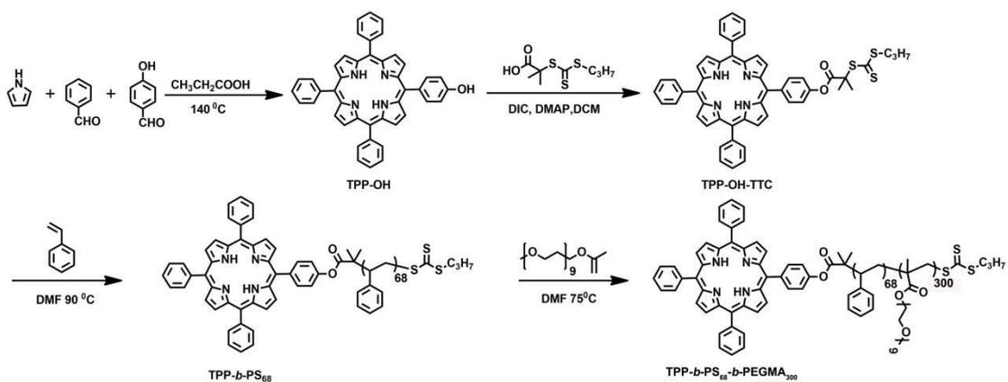
**Scheme S1.** Synthesis route of TPP-*b*-PS<sub>68</sub>-*b*-PEGMA<sub>300</sub>.
