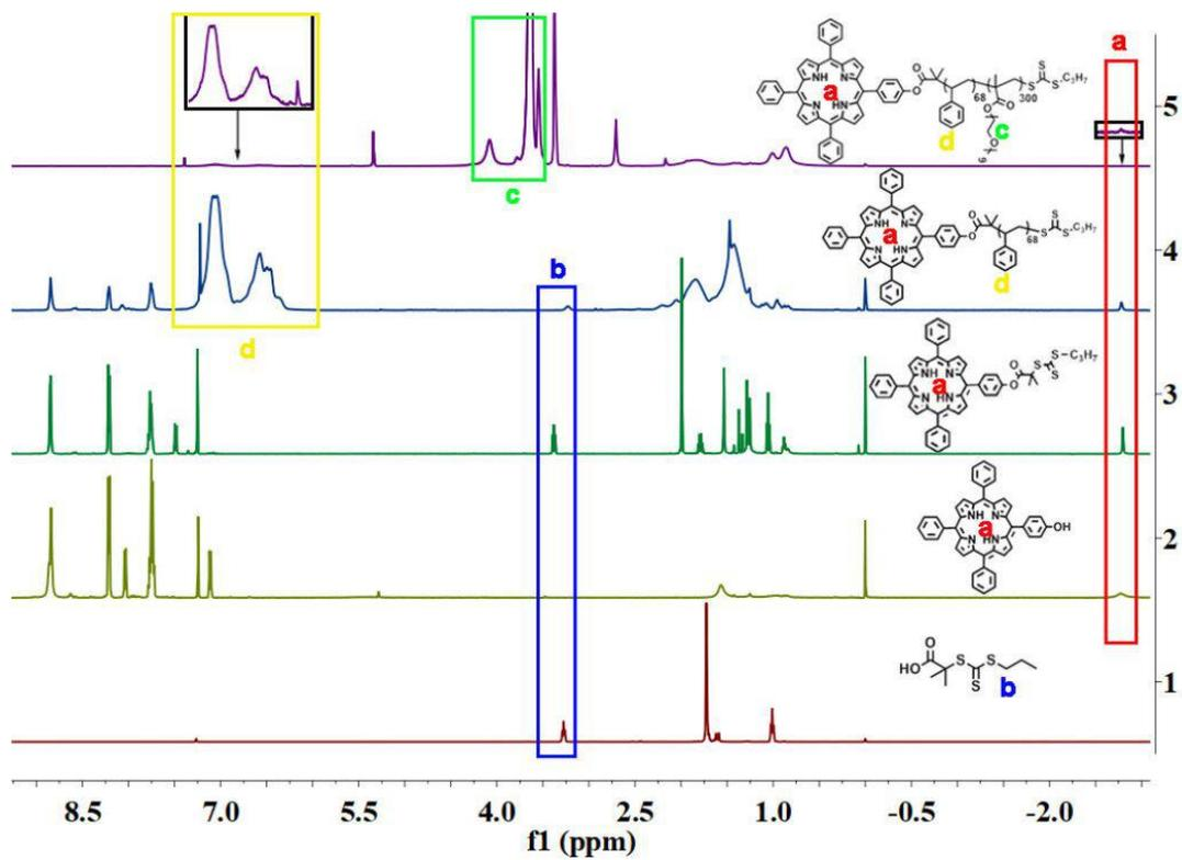
**Figure S4.**  $^1\text{H}$  NMR (in  $\text{CDCl}_3$ ) of TTCA (1), TPP-OH (2), TPP-OH-TTC (3), TPP-*b*-PS<sub>68</sub> (4), TPP-*b*-PS<sub>68</sub>-*b*-PEGMA<sub>300</sub> (5).
