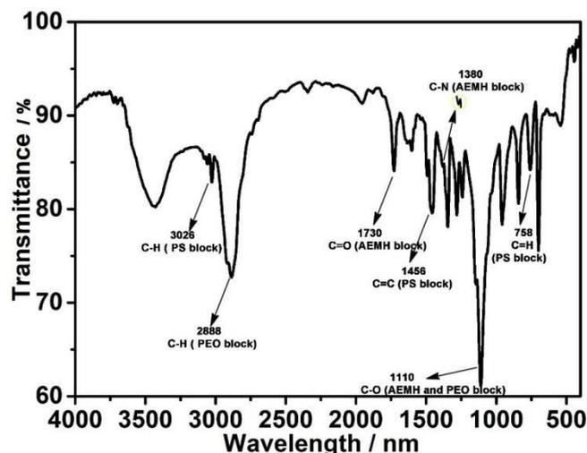
**Figure S9.** IR spectrum of PEO<sub>113</sub>-*b*-P(AEMH<sub>6</sub>-*co*-EANI<sub>1</sub>-*co*-St<sub>30</sub>).
