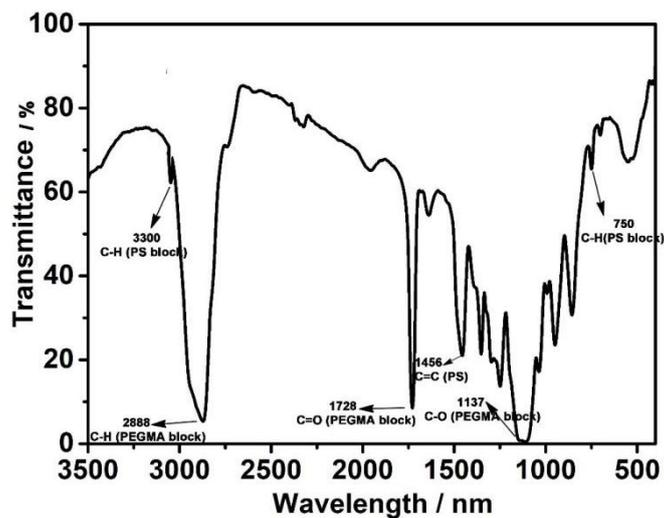
**Figure S6.** IR spectrum of TPP-*b*-PS<sub>68</sub>-*b*-PEGMA<sub>300</sub>.
