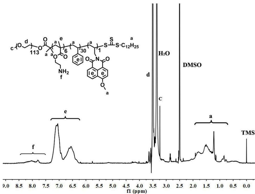
Figure S7.  $^1\text{H}$  NMR of the  $\text{PEO-}b\text{-P(AEMH}_6\text{-co-EANI}_1\text{-co-St}_{30}\text{)}$ .
