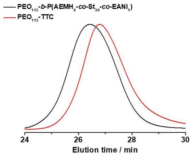
Figure S8. GPC trace of  $\text{PEO}_{113}\text{-}b\text{-P(AEMH}_6\text{-co-EANI}_1\text{-co-St}_{30}\text{)}$  and  $\text{PEO}_{113}\text{-TTC}$ .
