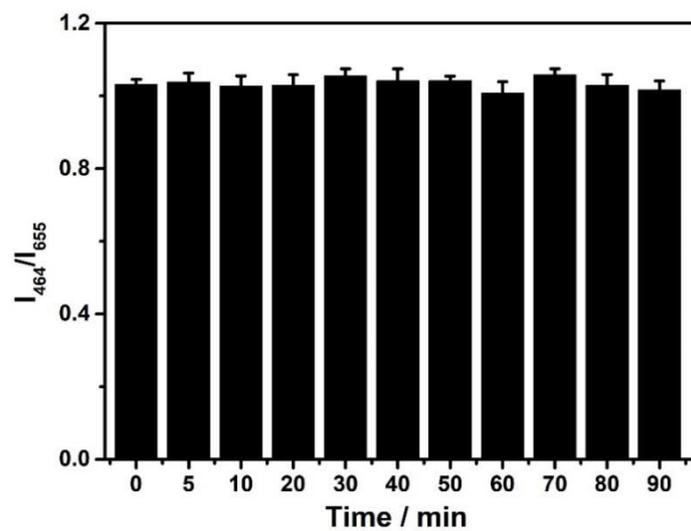
**Figure S16.** Fluorescence intensity changes ( $I_{464}/I_{655}$ ) of ZC-FPN ( $48 \mu\text{g}\cdot\text{mL}^{-1}$ ) under a continuous 365 nm UV lamp irradiation ( $2.8 \text{ mW}\cdot\text{cm}^{-2}$ ).
