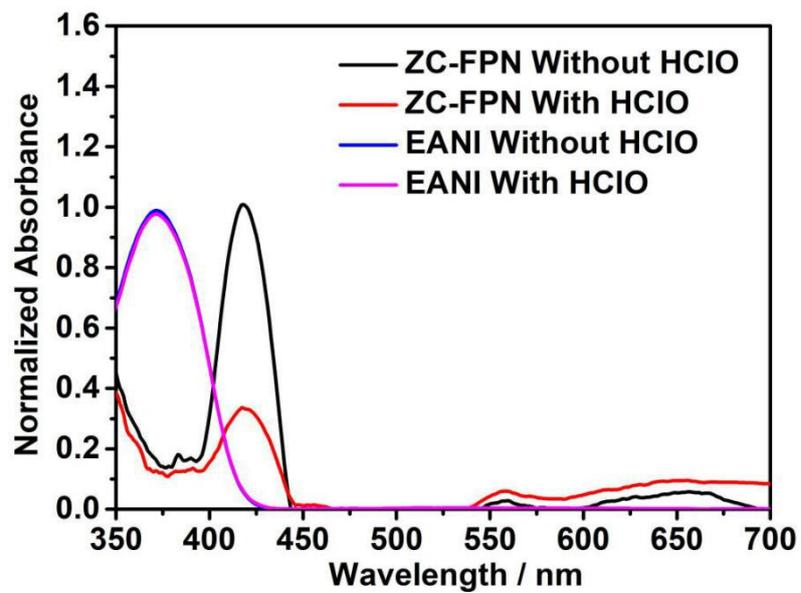
**Figure S10.** The normalized absorbance spectra of ZC-FPN ( $48 \mu\text{g}\cdot\text{mL}^{-1}$ ) and EANI without and with HClO ( $160 \mu\text{M}$ ).
