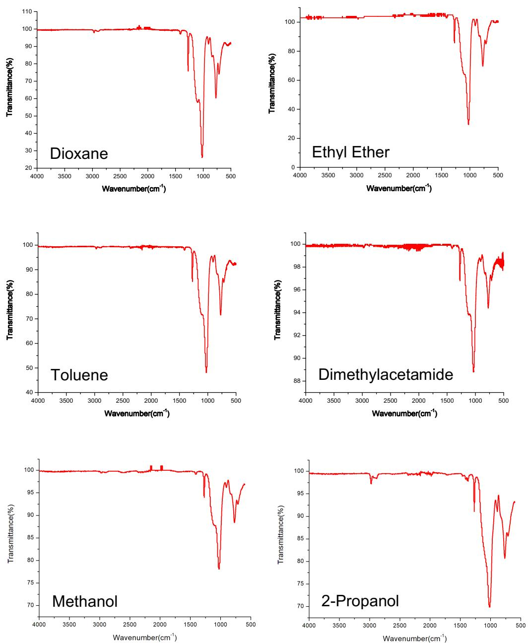
**Figure S31.** FTIR spectra of materials synthesized in different solvent (post-curing)
