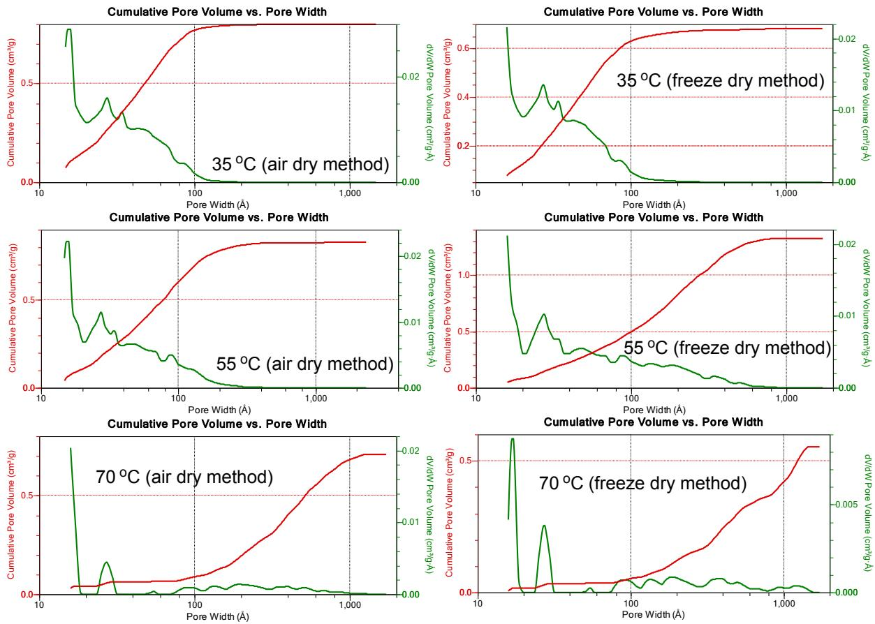
**Figure S19.** DFT pore size distribution graphs of materials synthesized in acetonitrile at different temperatures (gel washed by solvent (left), washed by solvent then freeze dried(right)).
