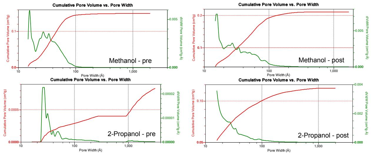
**Figure S4.** DFT pore size distribution graphs in mesopore and macropore region of materials synthesized in different solvents (pre-curing and post-curing).
