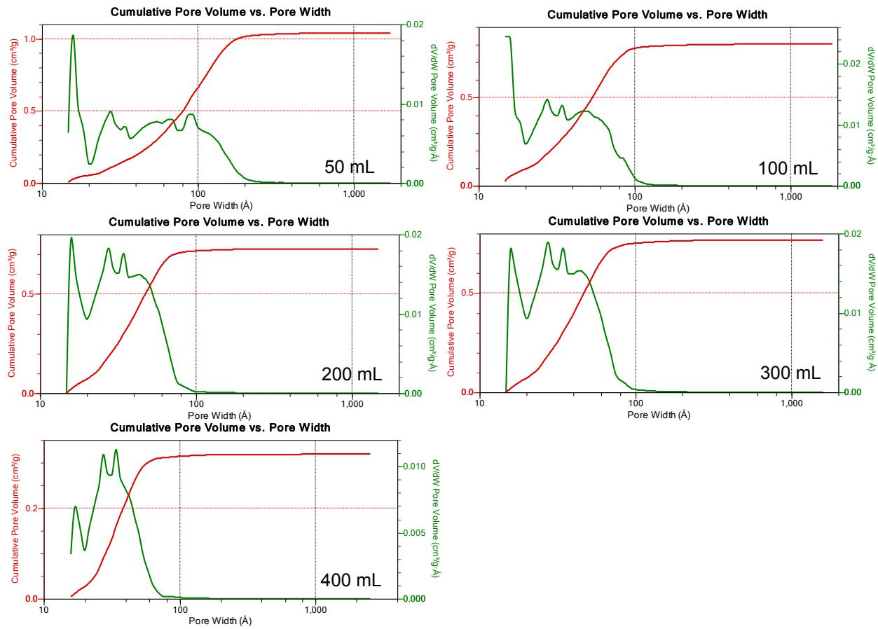
**Figure S8.** DFT pore size distribution graphs of material synthesized in different amounts of acetonitrile.
