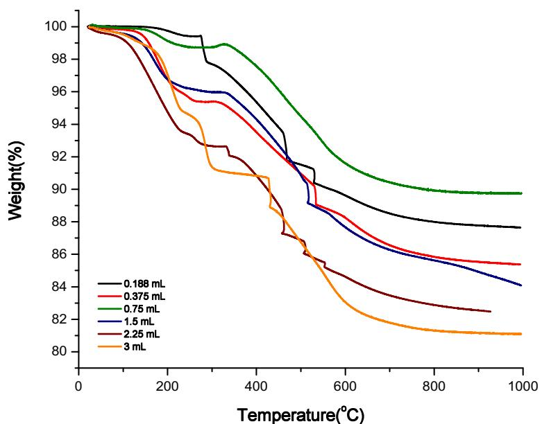
**Figure S9.** TGA graphs of materials synthesized in dichloromethane with different amounts of water.
