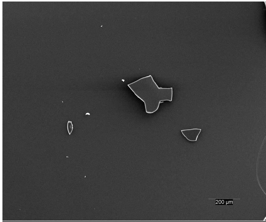
**Figure S23.** SEM images of condensed gel synthesized in acetonitrile at 70 °C with 0.75 mL of water (air dry method).
