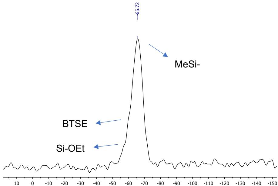
**Figure S27.** Si SSNMR spectra of material synthesized in acetonitrile.
