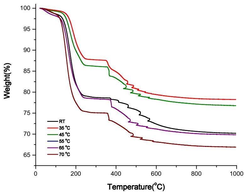
**Figure S15.** TGA graphs of samples from materials synthesized in acetonitrile at different temperatures.
