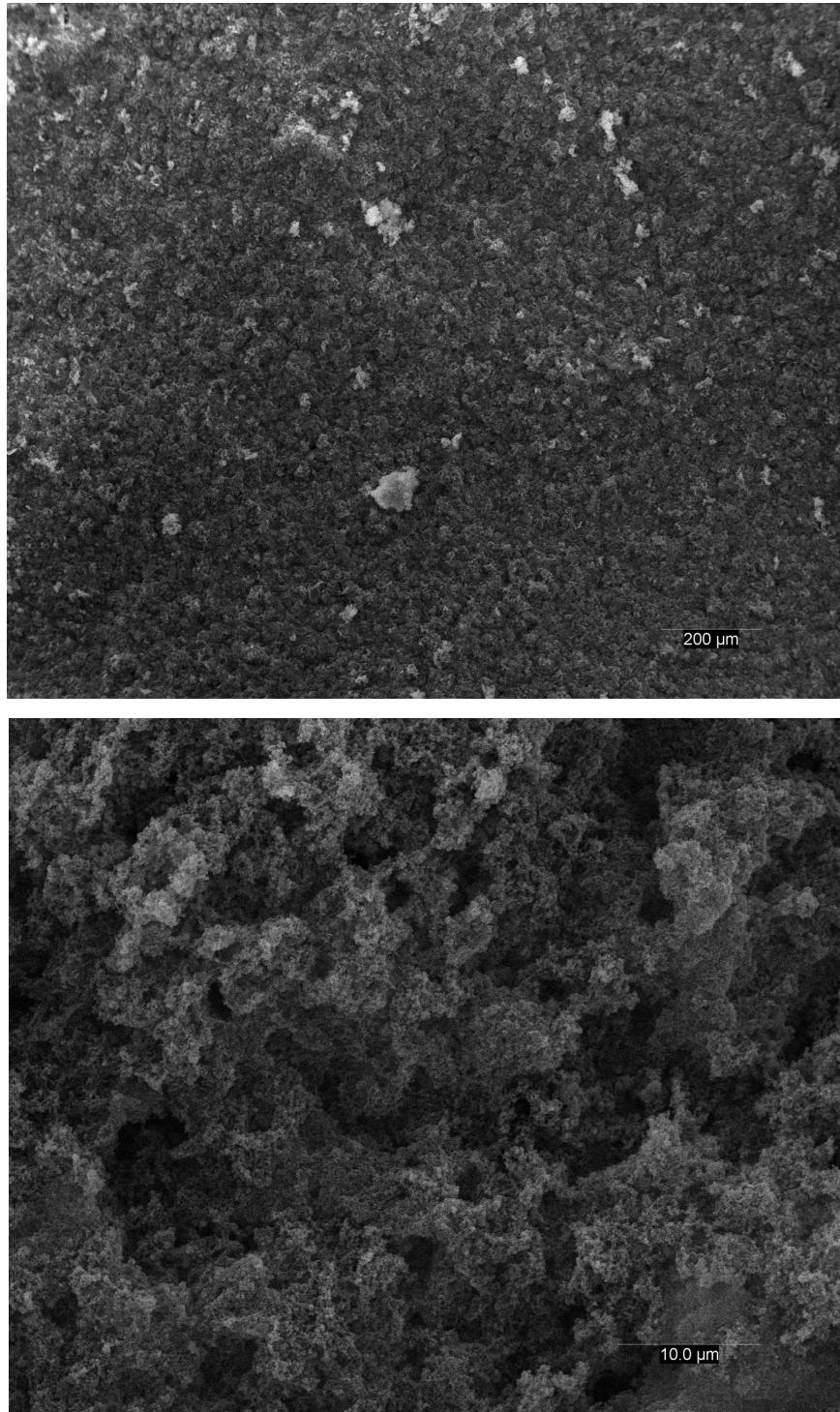
**Figure S20.** SEM images of particle gels synthesized in dichloromethane at room temperature (air dry method).
