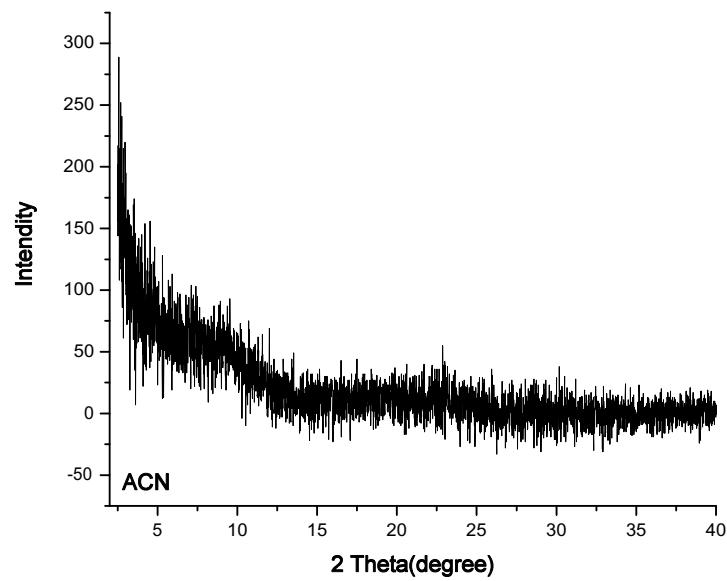
**Figure S25.** XRD spectra of material synthesized in acetonitrile. at room temperature (air dry method).
