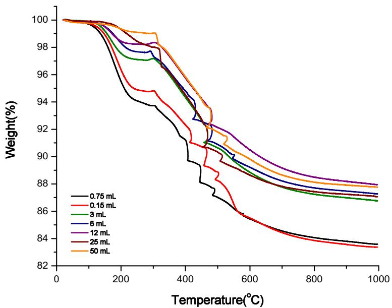
**Figure S11.** TGA graphs of materials synthesized in acetonitrile with different amounts of water.
