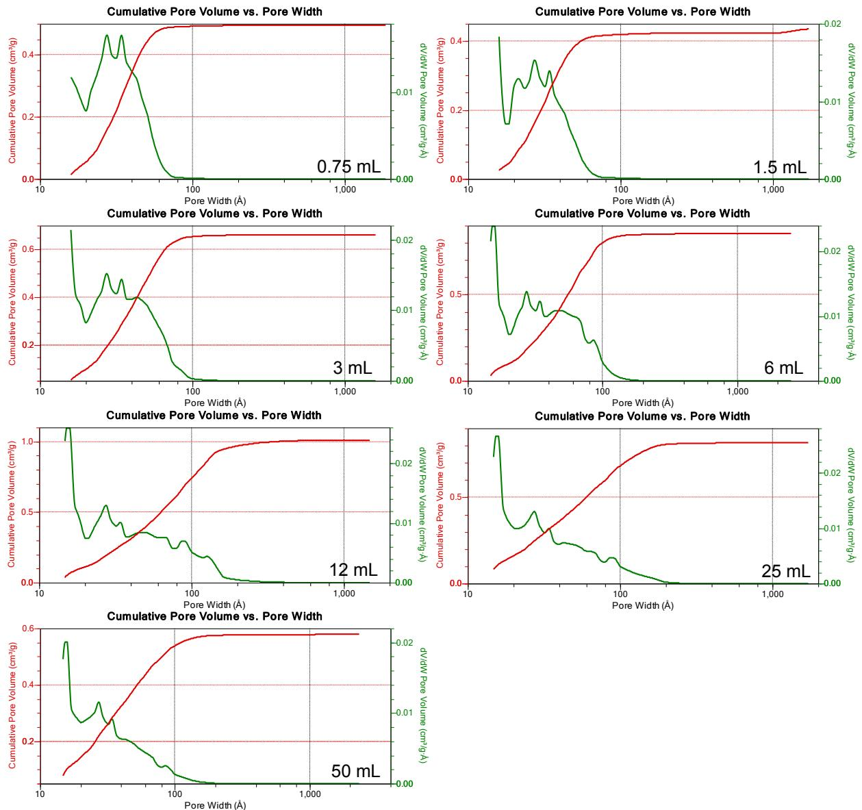
**Figure S12.** DFT pore size distribution graphs of material synthesized in acetonitrile with different amounts of water.
