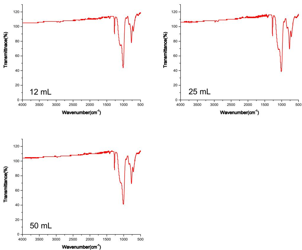
**Figure S35.** FTIR spectra of materials synthesized acetonitrile with different amounts of water.
