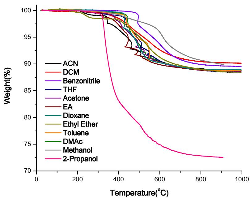
**Figure S2.** TGA graphs of materials synthesized in different solvents (post-curing).
