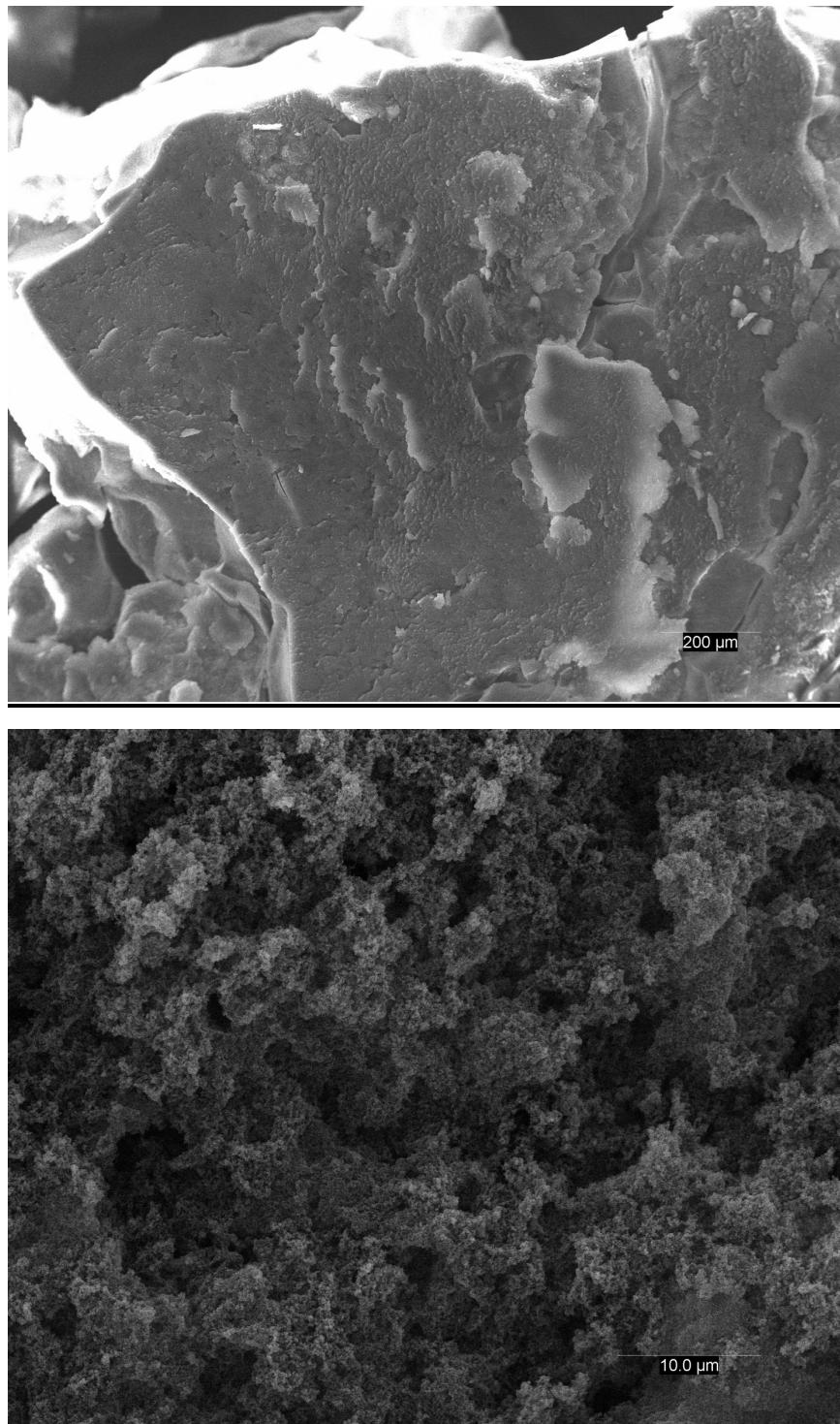
**Figure S22.** SEM images of light gel synthesized in acetonitrile at 70 °C with 25 mL of water (air dry method).
