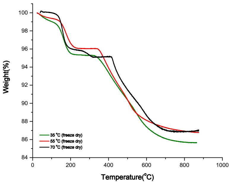
**Figure S17.** TGA graphs from materials synthesized in acetonitrile at different temperatures (gel washed by solvent and freeze dried).
