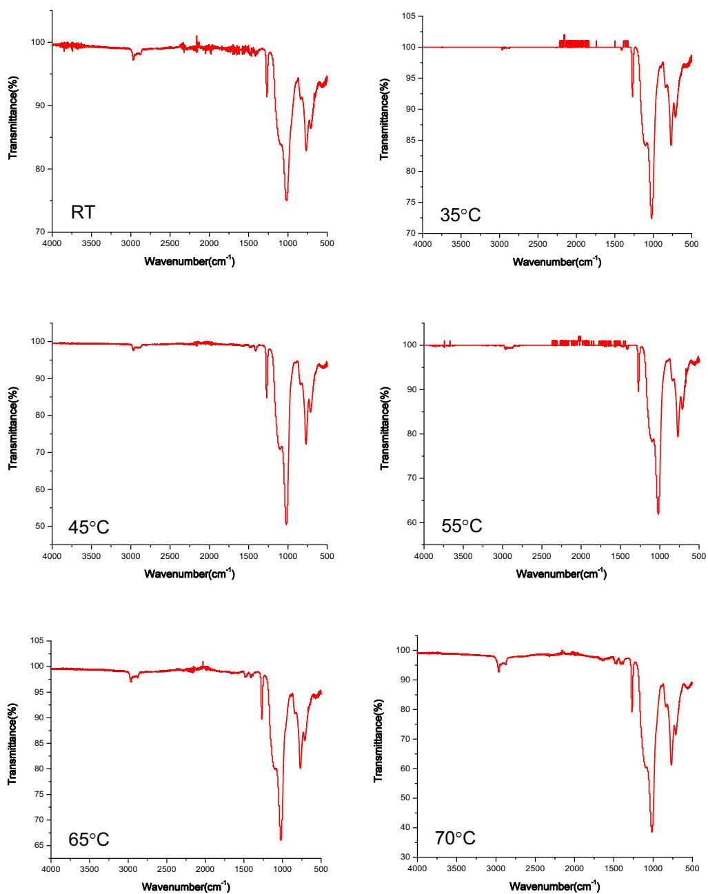
**Figure S37.** FTIR spectra of materials synthesized in acetonitrile at different temperatures.
