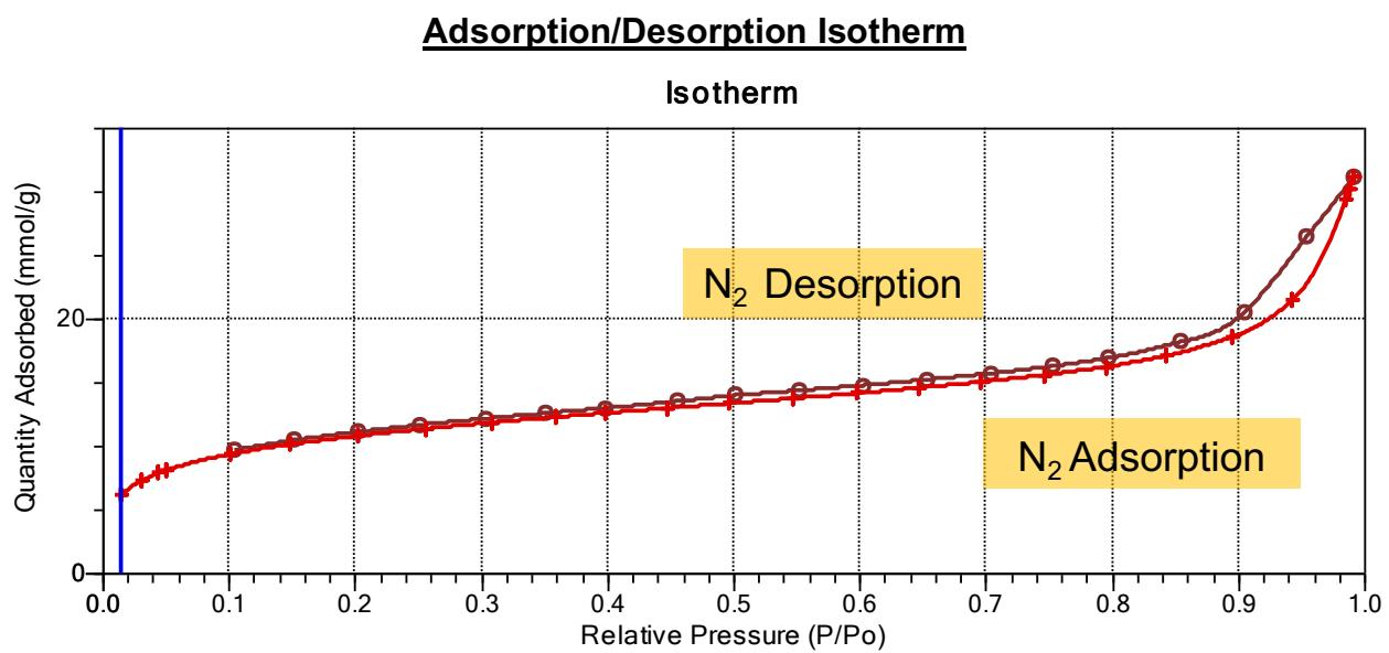
**Figure S29.** Representative example of nitrogen adsorption and desorption isotherm for the BET surface area analysis of material synthesized in dichloromethane under standard conditions.
