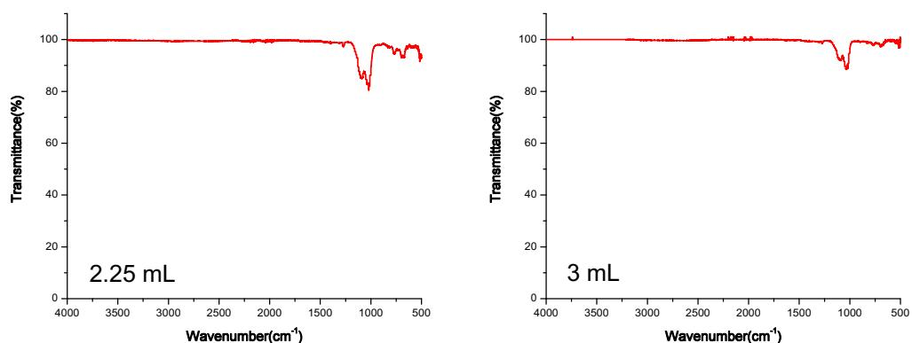
**Figure S34.** FTIR spectra of materials synthesized in dichloromethane with different amounts of water.
