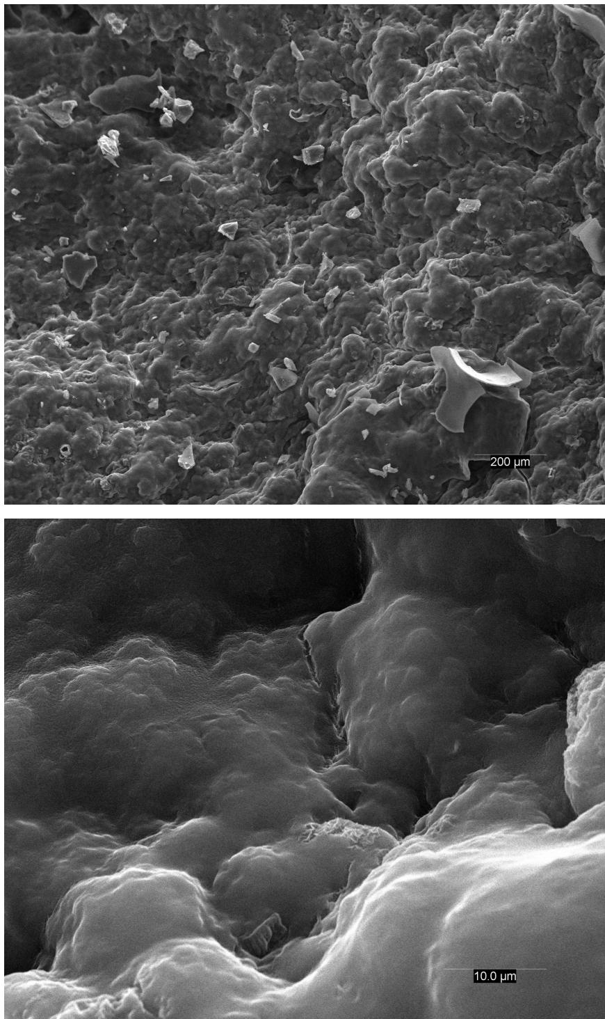
**Figure S21.** SEM images of particle gels synthesized in acetonitrile at room temperature (air dry method).
