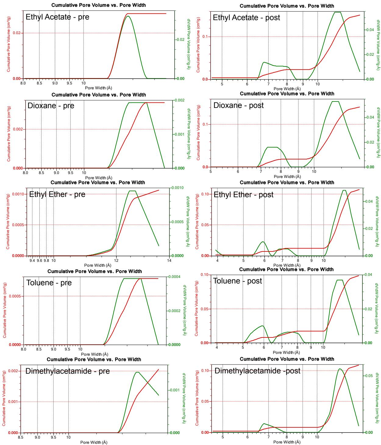
**Figure S3.** DFT pore size distribution graphs in micropore region of materials synthesized in different solvents (pre-curing and post-curing).
