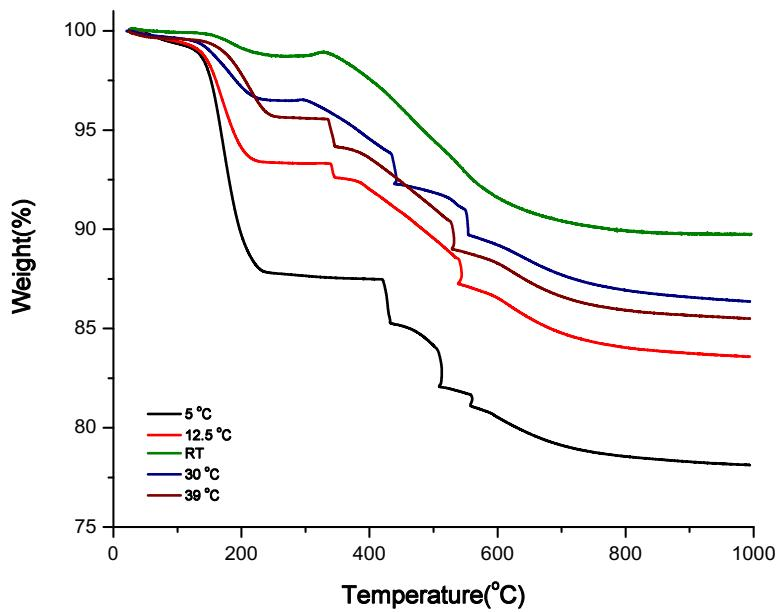
**Figure S13.** TGA graphs of materials synthesized in dichloromethane at different temperatures.
