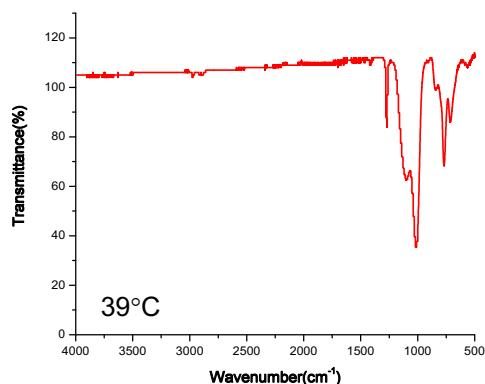
**Figure S36.** FTIR spectra of materials synthesized in dichloromethane at different temperatures.
