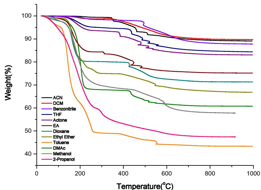
**Figure S1.** TGA graphs of materials from reactions synthesized in different solvents (pre-curing).
