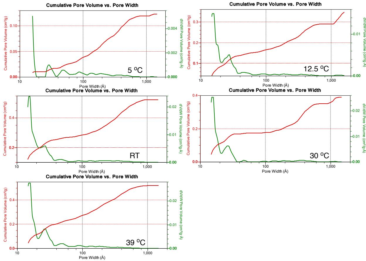
**Figure S14.** DFT pore size distribution graphs of materials synthesized in dichloromethane at different temperatures.
