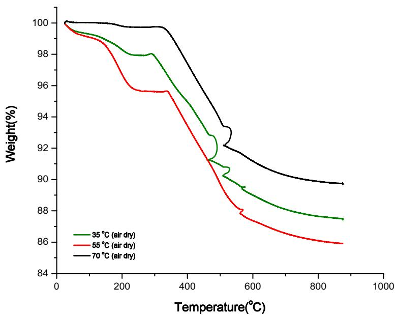
**Figure S16.** TGA graphs from materials synthesized in acetonitrile at different temperatures (gel washed by solvent).
