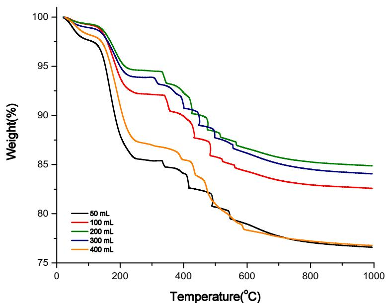
**Figure S7.** TGA graphs of samples from material synthesized in different amounts of acetonitrile.
