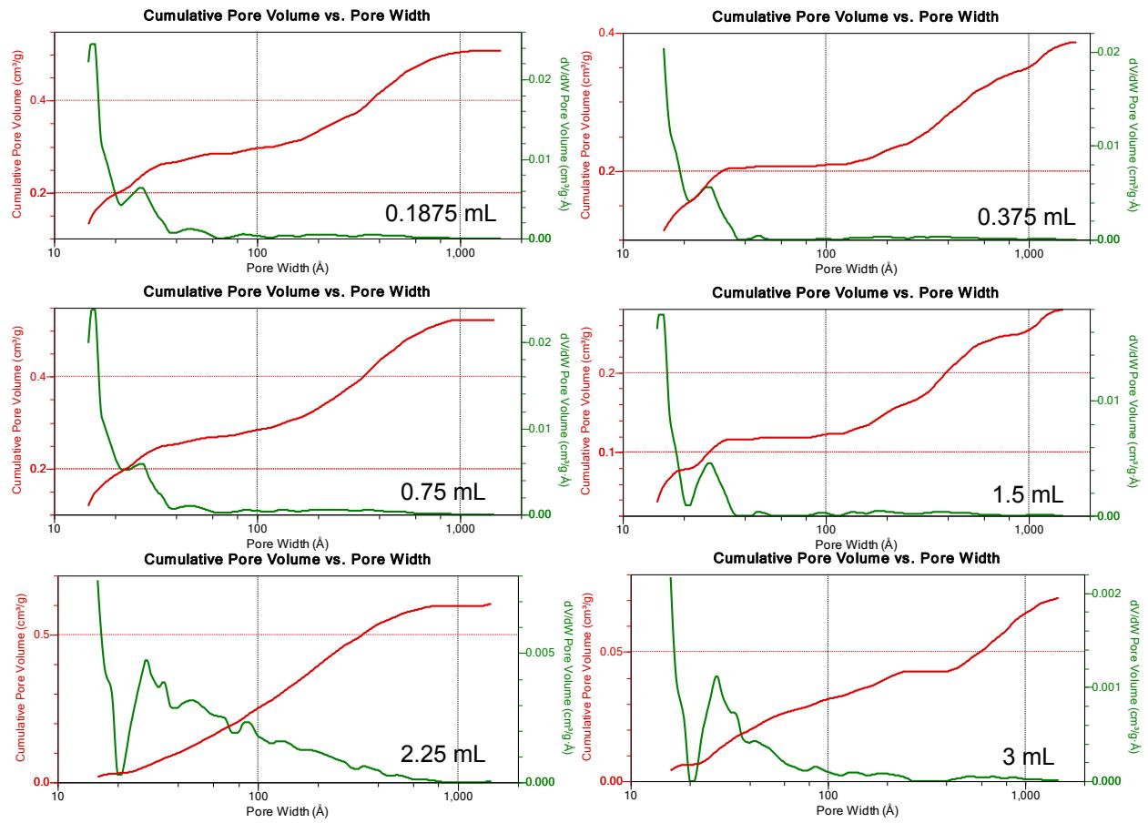
**Figure S10.** DFT pore size distribution graphs of material synthesized in dichloromethane with different amounts of water.
