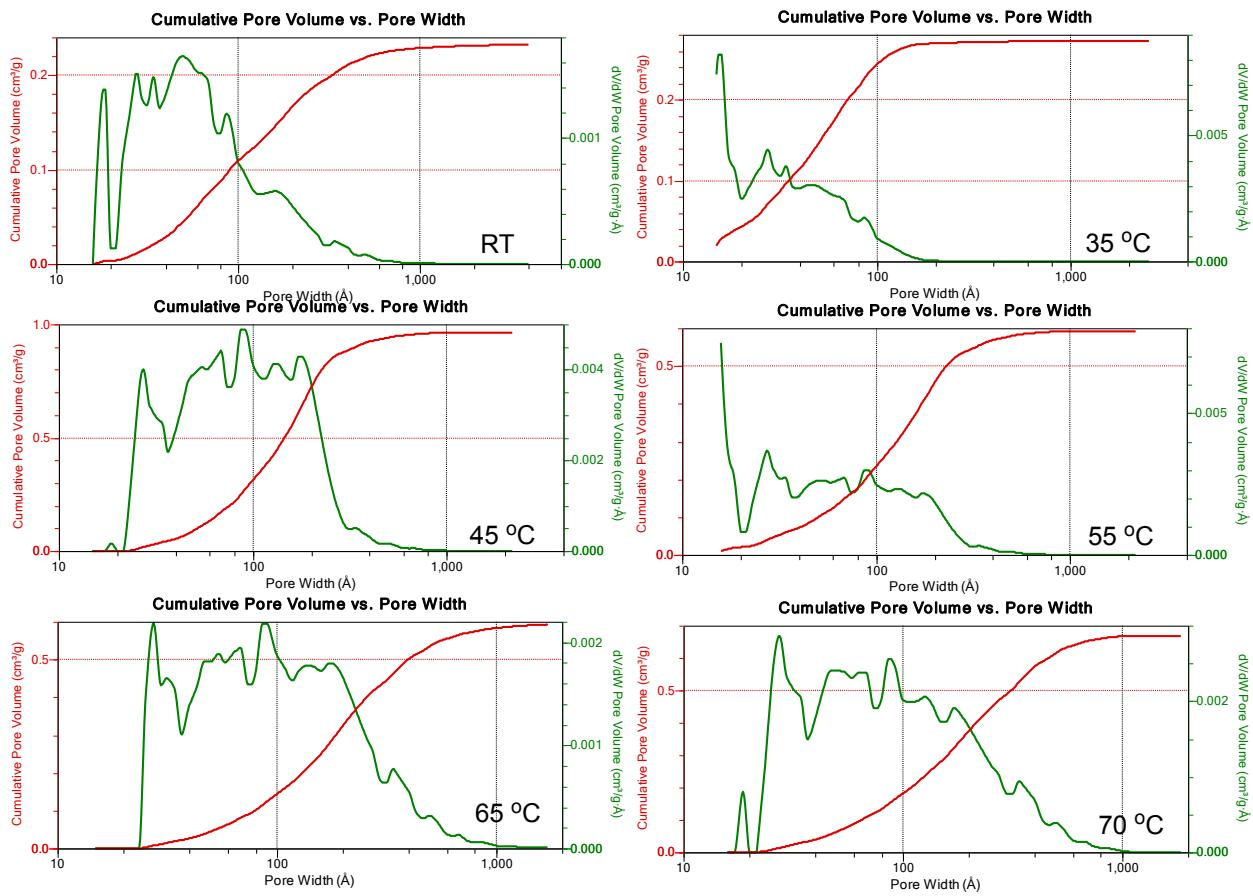
**Figure S18.** DFT pore size distribution graphs of materials synthesized in acetonitrile at different temperatures.
