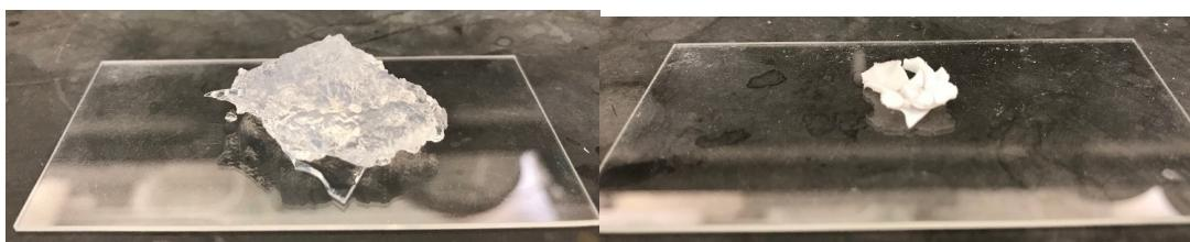
**Figure S26.** Before (left) and after (right) drying of material synthesized in acetonitrile at 70°C.
