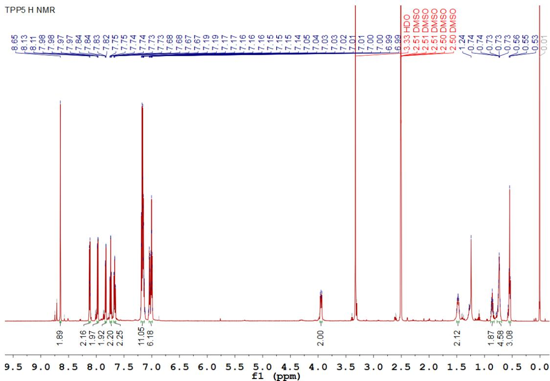
**Figure S41.** <sup>1</sup>H NMR spectrum of TPP5 in DMSO-*d*<sub>6</sub> at 298K.
