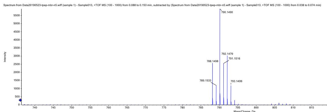
**Figure S4** ESI mass spectrum of cationic AIEgen TPP4.
