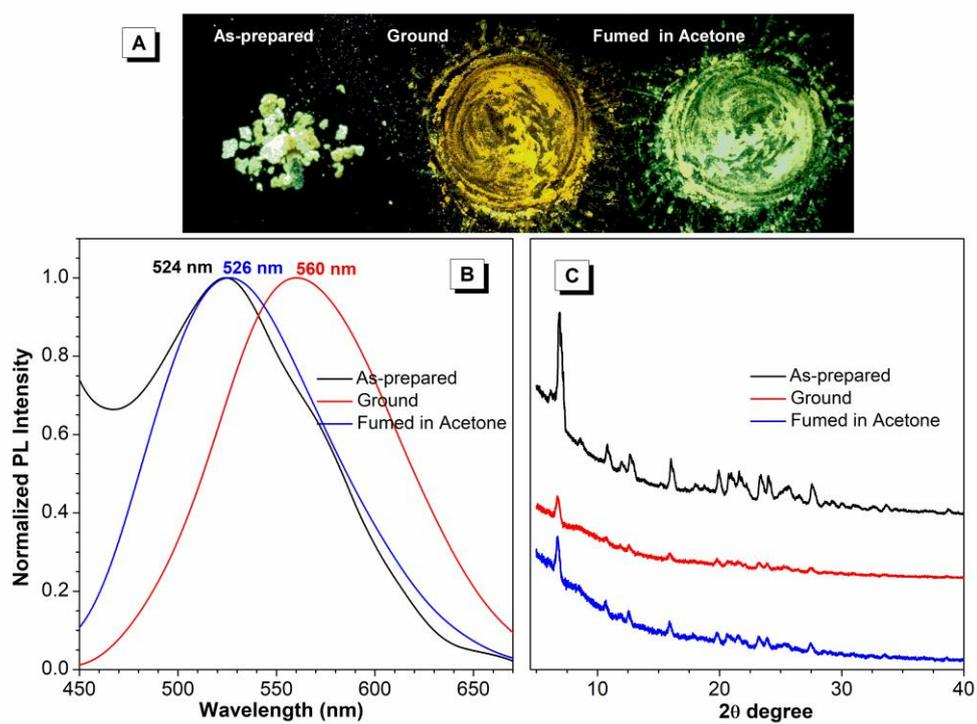
**Figure S20.** Fluorescent images (A), PL spectra (B), and powder XRD results (C) of as-prepared samples of cationic luminogen TPP5 after grinding and subsequent solvent fuming with acetone for 5 minutes.
