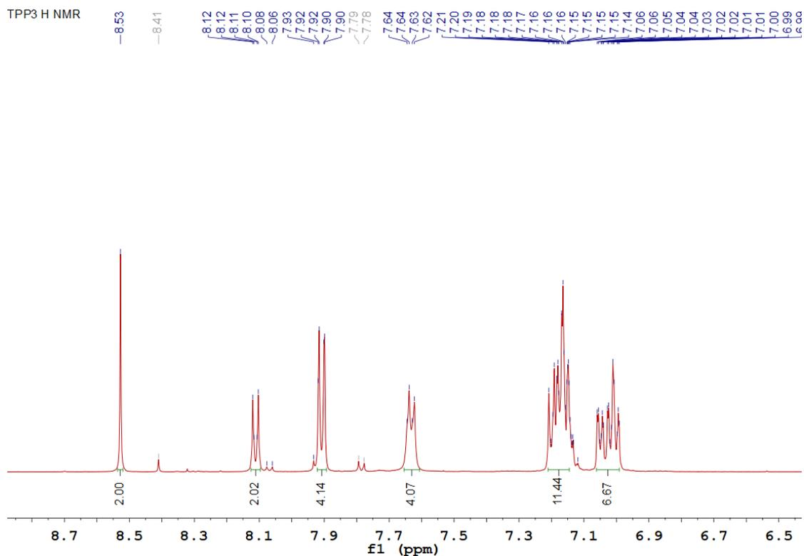
**Figure S36.** Enlarged aromatic region in the  $^1\text{H}$  NMR spectrum of TPP3 in  $\text{DMSO-}d_6$  at 298K.
