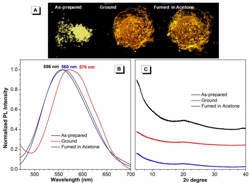
**Figure S19.** Fluorescent images (A), PL spectra (B), and powder XRD results (C) of as-prepared samples of cationic luminogen TPP4 after grinding and subsequent solvent fuming with acetone for 5 minutes.
