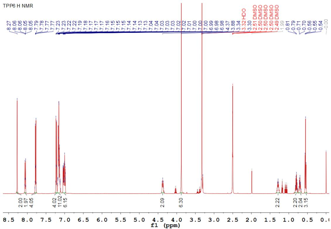
**Figure S44.**  $^1\text{H}$  NMR spectrum of TPP6 in  $\text{DMSO-}d_6$  at 298K.
