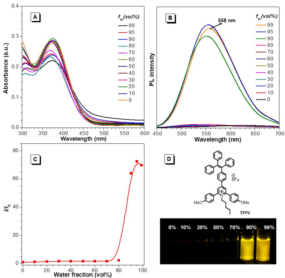
**Figure S17.** (A) UV-Vis absorption spectra and (B) photoluminescence spectra of TPP6 in DMSO and DMSO/water mixtures with different water fraction ( $f_w$ ). (C) Plots of the maximum emission intensities of TPP6 in DMSO and DMSO/water mixtures versus  $f_w$ . (D) Chemical structure and images of TPP6 under UV lamp in DMSO and DMSO/water mixtures with different  $f_w$ . Concentration = 10  $\mu\text{M}$ .
