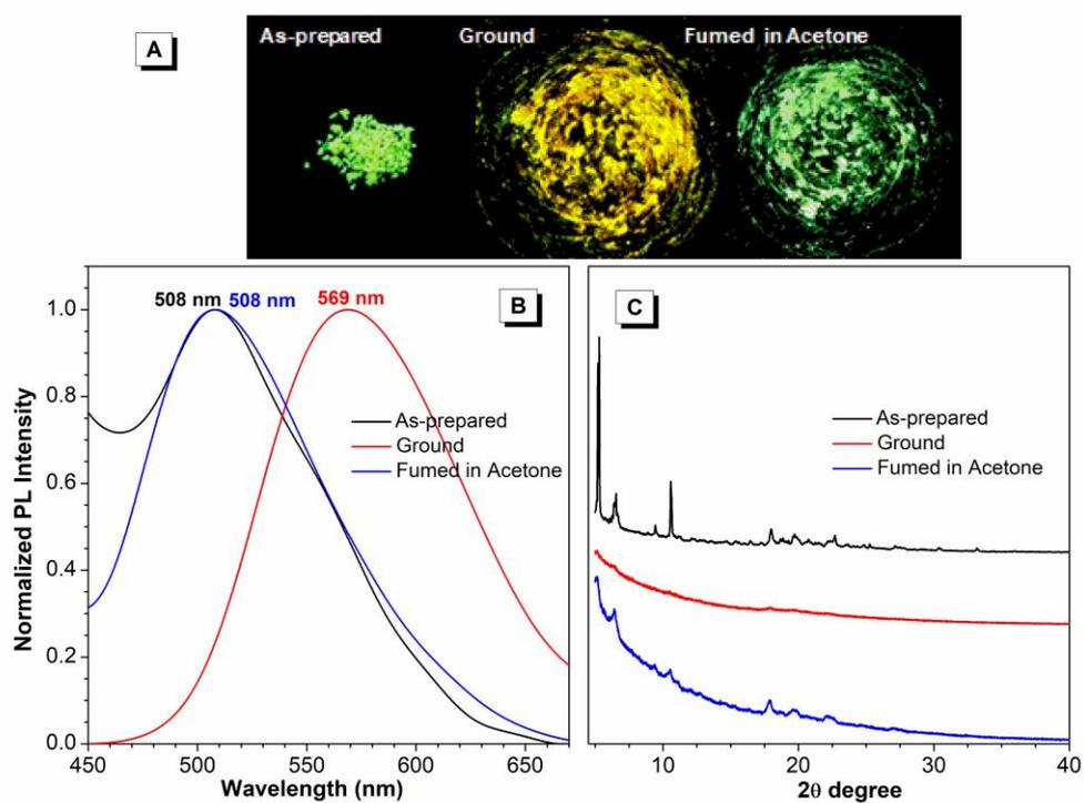
**Figure S21.** Fluorescent images (A), PL spectra (B), and powder XRD results (C) of as-prepared samples of cationic luminogen TPP6 after grinding and subsequent solvent fuming with acetone for 5 minute.
