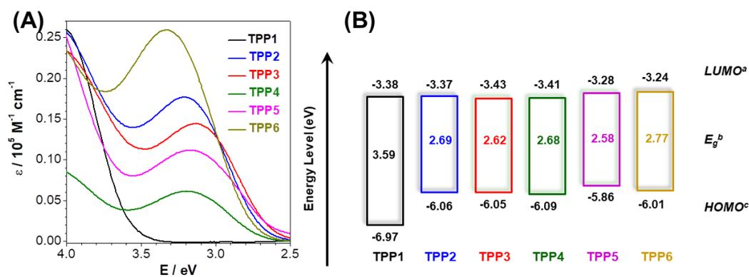
**Figure S12.** (A) UV-Vis absorption spectra of TPPs in DMSO (10  $\mu$ M). (B) Energy levels of molecular orbitals of TPPs. <sup>a</sup> LUMO levels were calculated by the first reduction peaks in the electrochemical measurement with respect to ferrocene. <sup>b</sup> Optical Band gap ( $E_g$ ) was estimated from the absorption edge wavelength, which was obtained from the offset wavelength derived from the low energy absorption band. <sup>c</sup> HOMO = LUMO -  $E_g$ .
