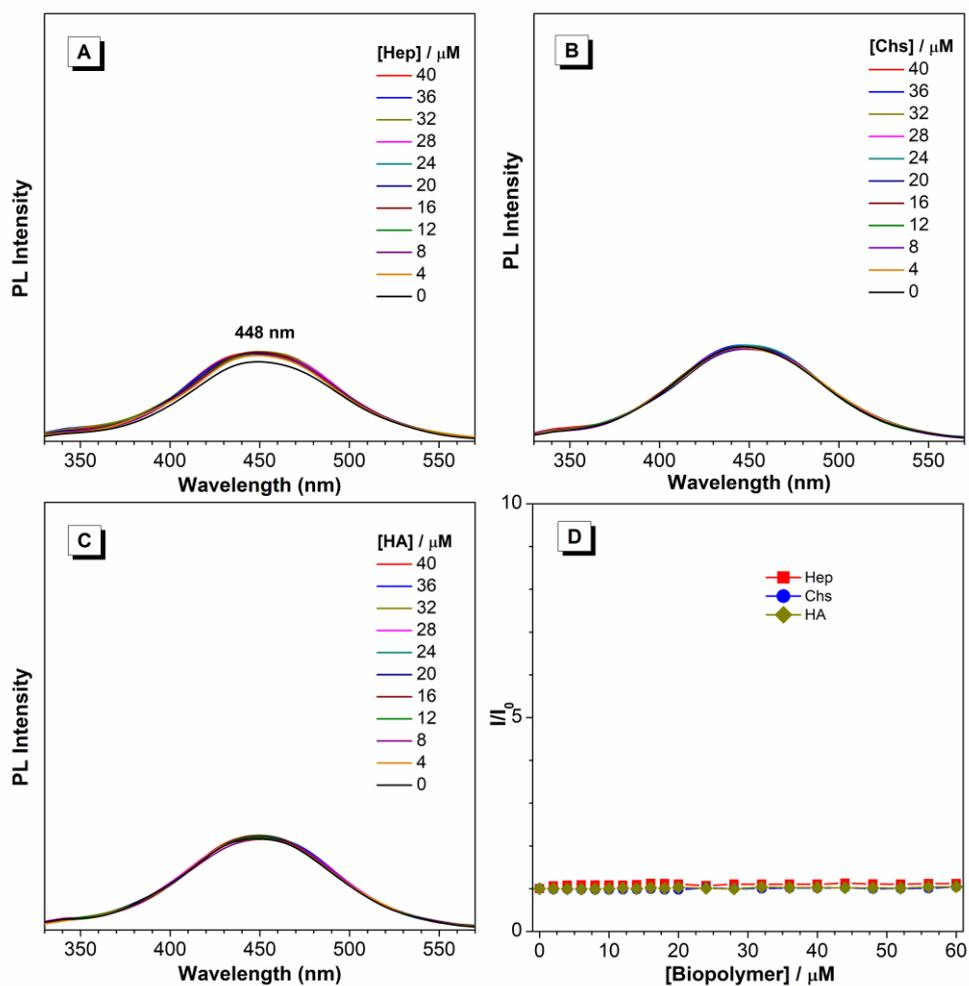
**Figure S22.** PL spectra of TPP1 with different concentration of (A) heparin (Hep), (B) chondroitin 4-sulfate (Chs), and (C) hyaluronic acid (HA) . (D) Curve of relative fluorescence intensity of TPP1 with biopolymer concentration. Solvent: DMSO/H<sub>2</sub>O = 50/50 by volume; concentration of cationic AIEgens: 10  $\mu\text{M}$ .
