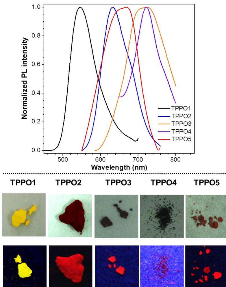
**Figure S7.** (Up) Photoluminescence spectra of as-prepared TPPOs samples in the solid state.
