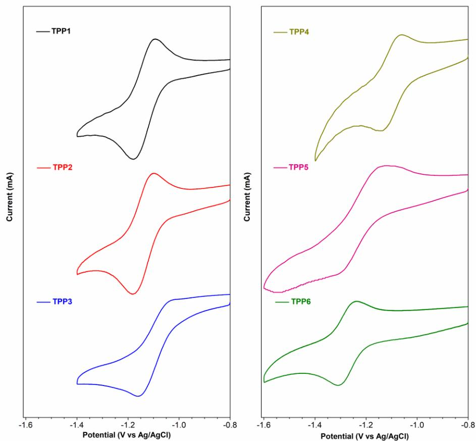
**Figure S11.** Cyclic voltametry spectra of TPPs in DCM (1 mM) measured with  $[n\text{-Bu}_4\text{N}][\text{PF}_6]$  (0.1 M) as a supporting electrolyte with ferrocene as reference.
