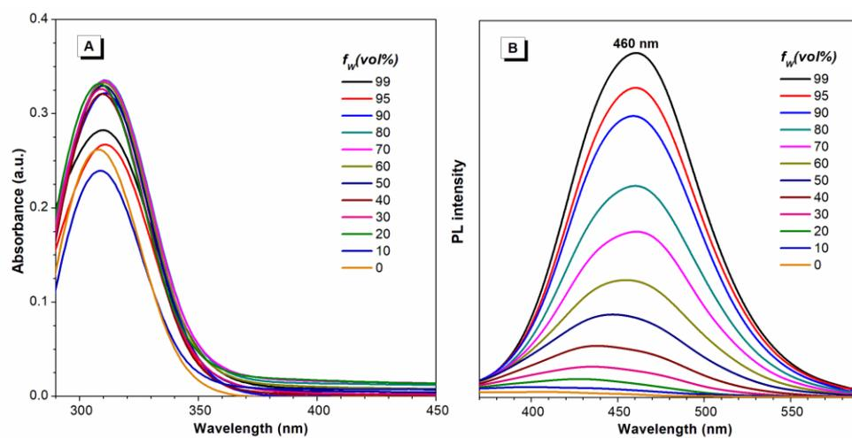
**Figure S9.** (A) UV-Vis absorption spectra and (B) photoluminescence spectra of TPP1 in DMSO and DMSO/water mixtures with different water fraction ( $f_w$ ). Concentration = 10  $\mu$ M.
