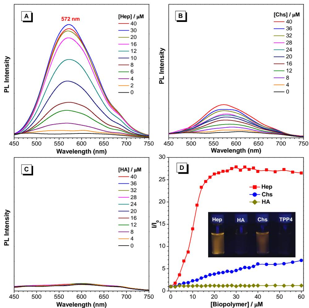
**Figure S25.** PL spectra of TPP4 with different concentration of (A) heparin (Hep), (B) chondroitin 4-sulfate (Chs), and (C) hyaluronic acid (HA) . (D) Curve of relative fluorescence intensity of TPP4 with biopolymer concentration. Solvent: DMSO/H<sub>2</sub>O = 50/50 by volume; concentration of cationic AIEgens: 10  $\mu\text{M}$ . Inset: fluorescent images for the mixture of TPP4 in absence or presence of biopolymer (40  $\mu\text{M}$ ) under UV lamp.
