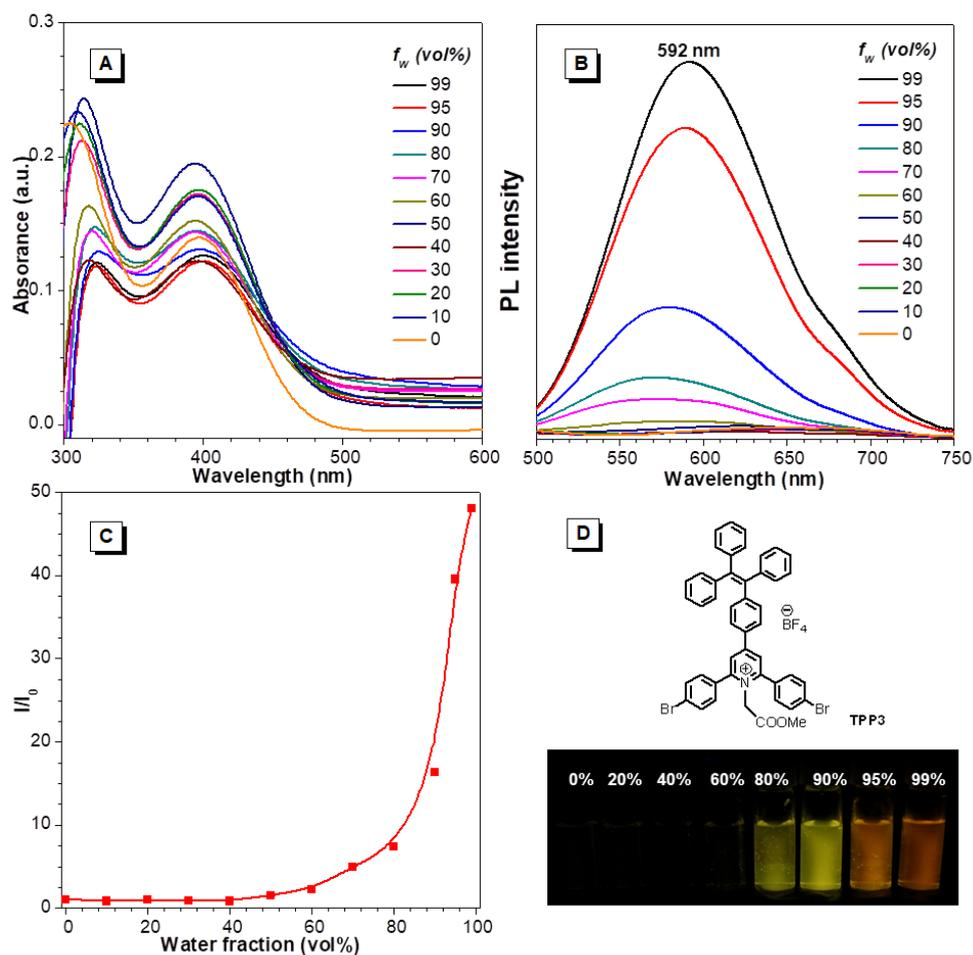
**Figure S14.** (A) UV-Vis absorption spectra and (B) photoluminescence spectra of TPP3 in DMSO and DMSO/water mixtures with different water fraction ( $f_w$ ). (C) Plots of the maximum emission intensities of TPP3 in DMSO and DMSO/water mixtures versus  $f_w$ . (D) Chemical structure and images of TPP3 under UV lamp in DMSO and DMSO/water mixtures with different  $f_w$ . Concentration = 10  $\mu\text{M}$ .
