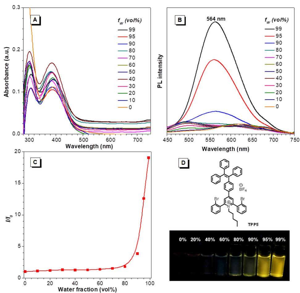
**Figure S16.** (A) UV-Vis absorption spectra and (B) photoluminescence spectra of TPP5 in DMSO and DMSO/water mixtures with different water fraction ( $f_w$ ). (C) Plots of the maximum emission intensities of TPP5 in DMSO and DMSO/water mixtures versus  $f_w$ . (D) Chemical structure and images of TPP5 under UV lamp in DMSO and DMSO/water mixtures with different  $f_w$ . Concentration = 10  $\mu\text{M}$ .
