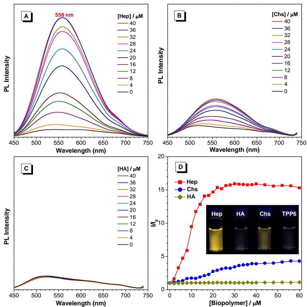
**Figure S27.** PL spectra of TPP6 with different concentration of (A) heparin (Hep), (B) chondroitin 4-sulfate (Chs), and (C) hyaluronic acid (HA) . (D) Curve of relative fluorescence intensity of TPP6 with biopolymer concentration. Solvent: DMSO/H<sub>2</sub>O = 50/50 by volume; concentration of cationic AIEgens: 10  $\mu\text{M}$ . Inset: fluorescent images for the mixture of TPP6 in absence or presence of biopolymer (40  $\mu\text{M}$ ) under UV lamp.
