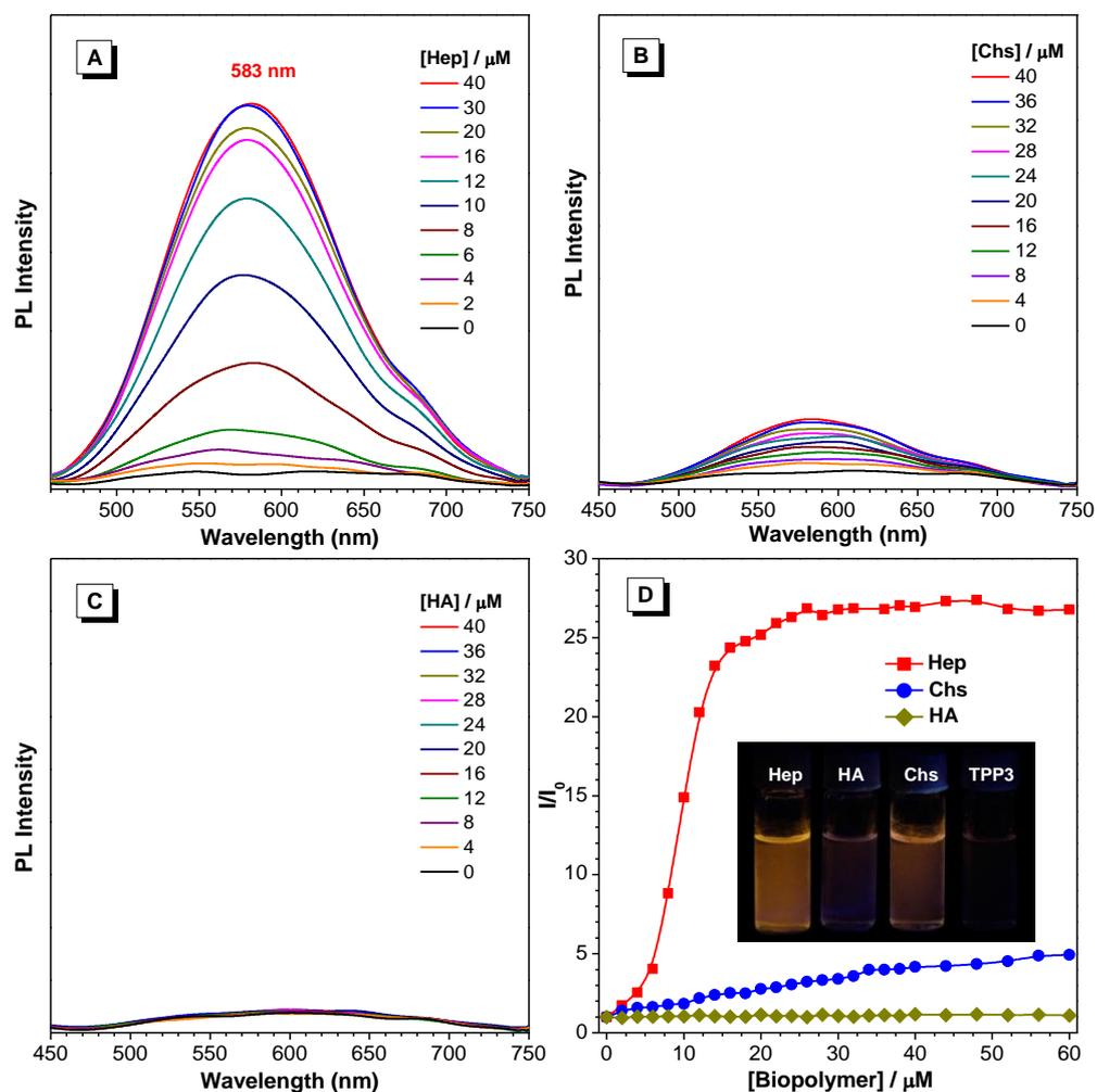
**Figure S24.** PL spectra of TPP3 with different concentration of (A) heparin (Hep), (B) chondroitin 4-sulfate (Chs), and (C) hyaluronic acid (HA) . (D) Curve of relative fluorescence intensity of TPP3 with biopolymer concentration. Solvent: DMSO/H<sub>2</sub>O = 50/50 by volume; concentration of cationic AIEgens: 10  $\mu\text{M}$ . Inset: fluorescent images for the mixture of TPP3 in absence or presence of biopolymer (40  $\mu\text{M}$ ) under UV lamp.
