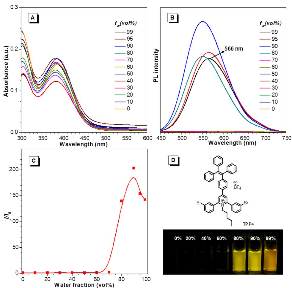
**Figure S15.** (A) UV-Vis absorption spectra and (B) photoluminescence spectra of TPP4 in DMSO and DMSO/water mixtures with different water fraction ( $f_w$ ). (C) Plots of the maximum emission intensities of TPP4 in DMSO and DMSO/water mixtures versus  $f_w$ . (D) Chemical structure and images of TPP4 under UV lamp in DMSO and DMSO/water mixtures with different  $f_w$ . Concentration = 10  $\mu$ M.
