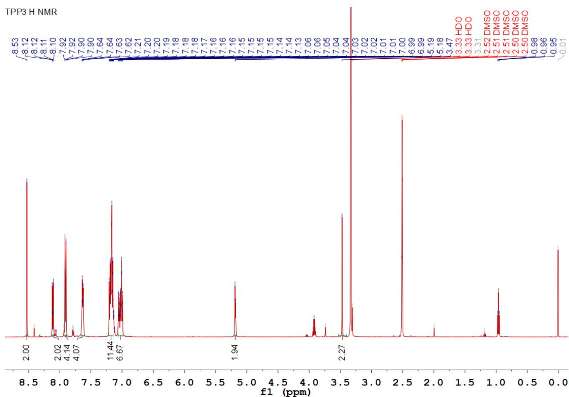
**Figure S35.**  $^1\text{H}$  NMR spectrum of TPP3 in  $\text{DMSO-}d_6$  at 298K.
