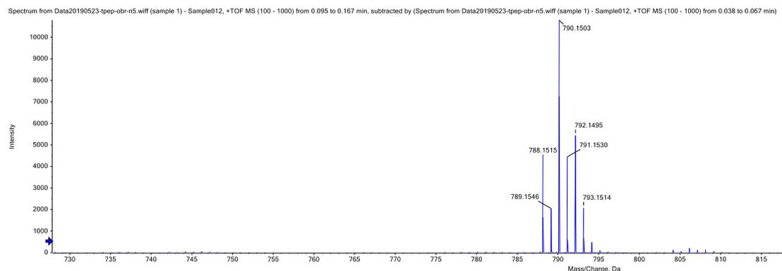
**Figure S5** ESI mass spectrum of cationic AIEgen TPP5.
