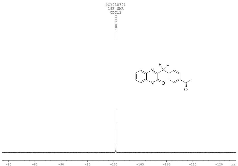
**Fig. S30** <sup>19</sup>F NMR spectrum of compound 3aj
