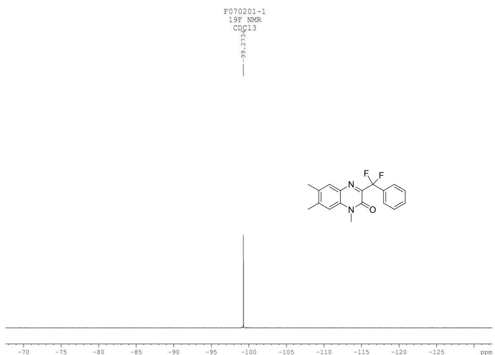
**Fig. S51**  $^{19}\text{F}$  NMR spectrum of compound **3ba**
