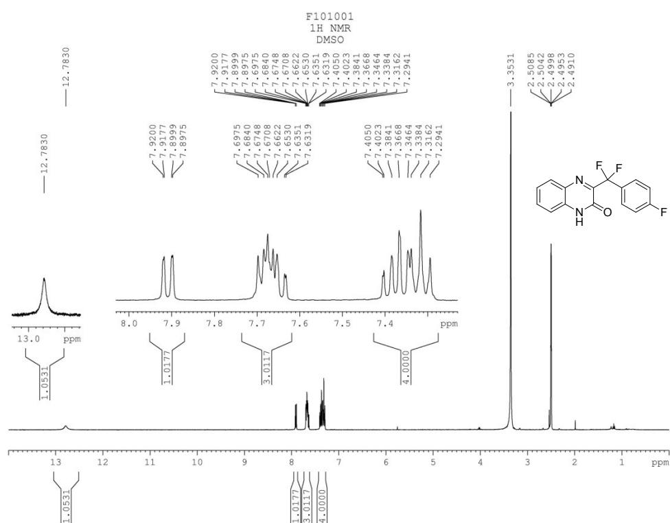
**Fig. S88**  $^1\text{H}$  NMR spectrum of compound **3nh**
