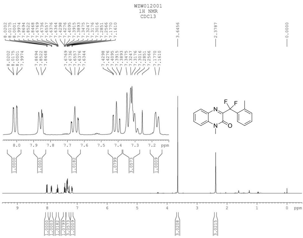
**Fig. S7**  $^1\text{H}$  NMR spectrum of compound **3ac**
