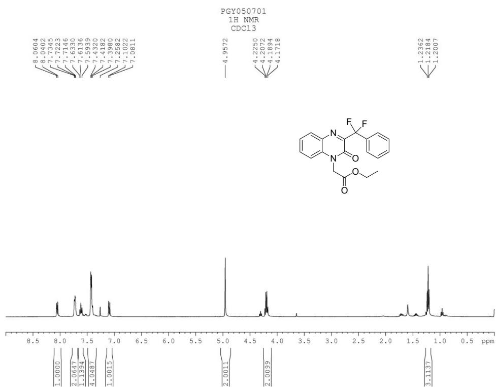
**Fig. S82** <sup>1</sup>H NMR spectrum of compound **3ma**
