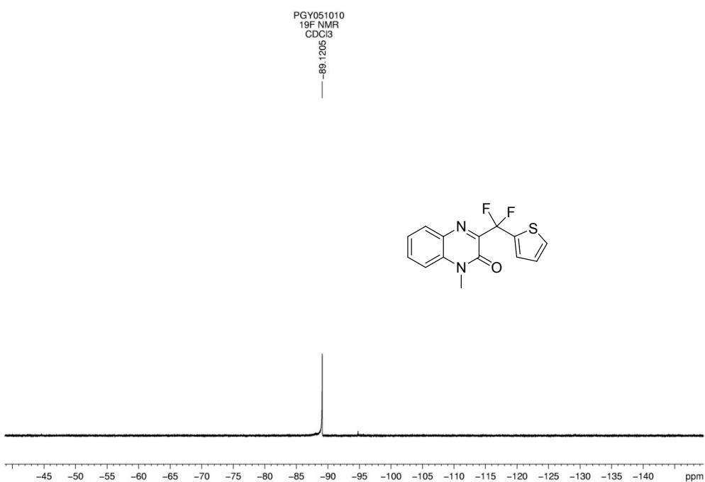
**Fig. S45** <sup>19</sup>F NMR spectrum of compound 3ao
