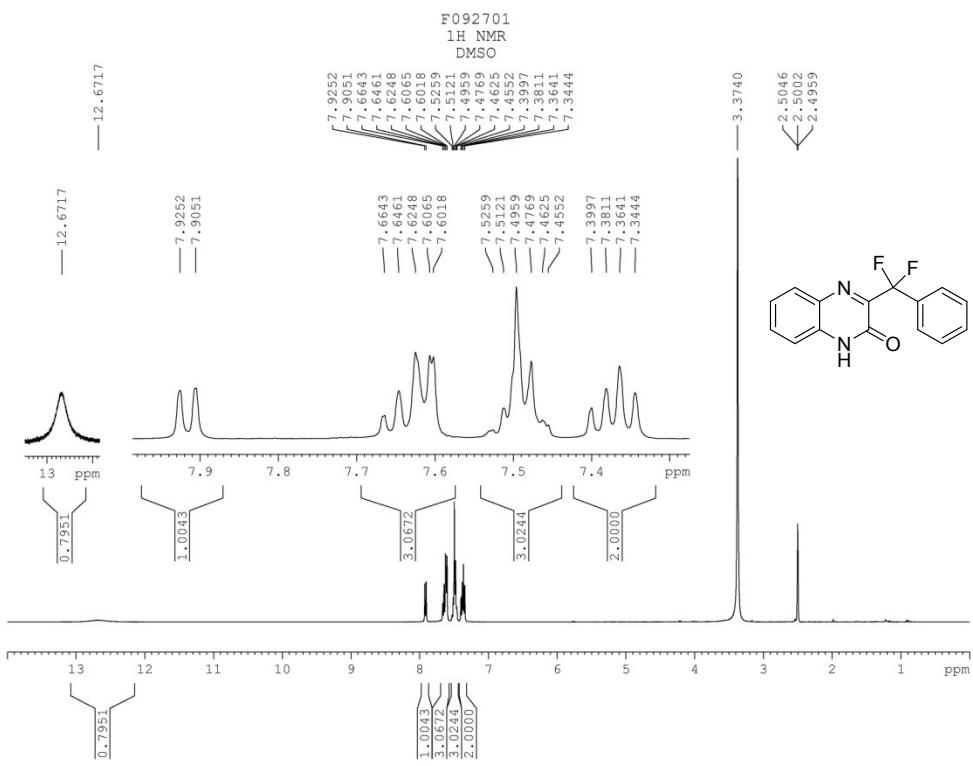
**Fig. S85**  $^1\text{H}$  NMR spectrum of compound **3na**
