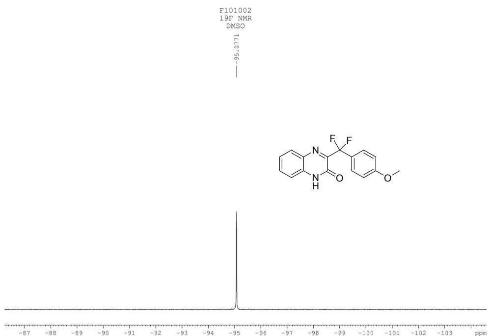
**Fig. S93** <sup>19</sup>F NMR spectrum of compound 3nf
