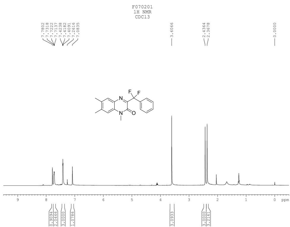
**Fig. S49** <sup>1</sup>H NMR spectrum of compound **3ba**
