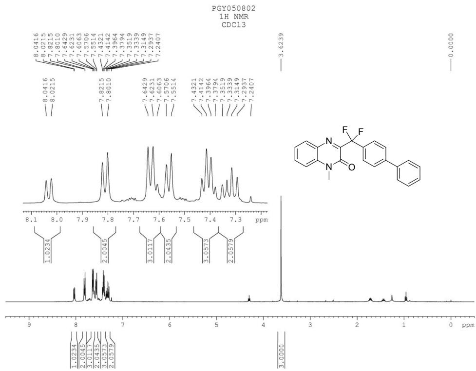
**Fig. S37**  $^1\text{H}$  NMR spectrum of compound **3am**
