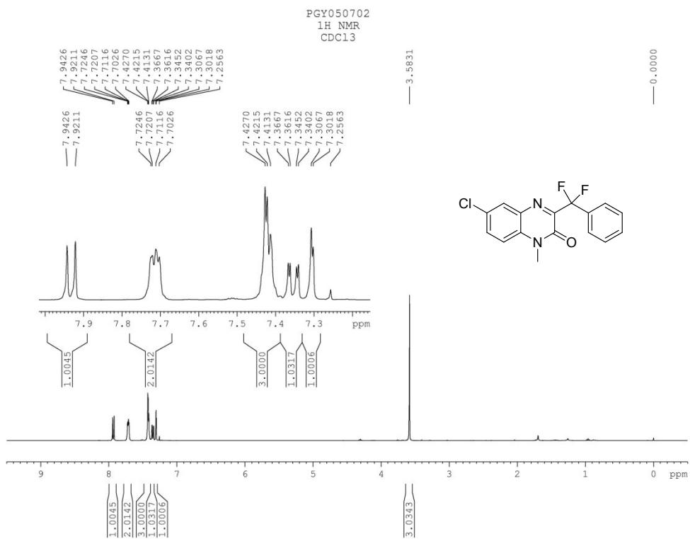
**Fig. S55**  $^1\text{H}$  NMR spectrum of compound **3da**
