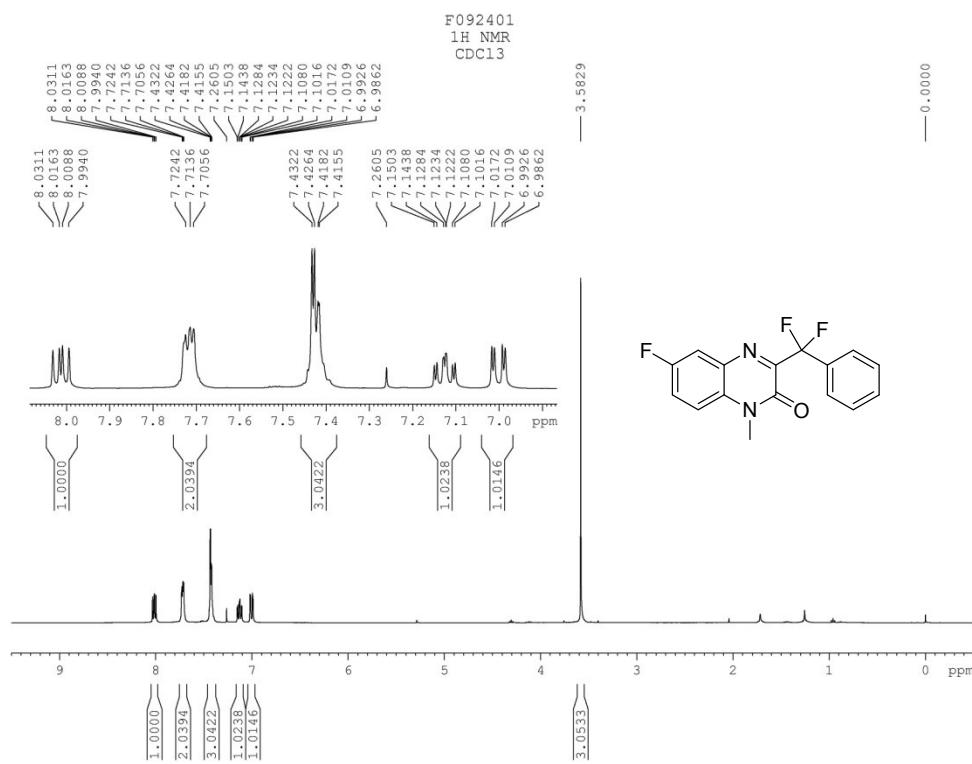
**Fig. S52**  $^1\text{H}$  NMR spectrum of compound **3ca**
