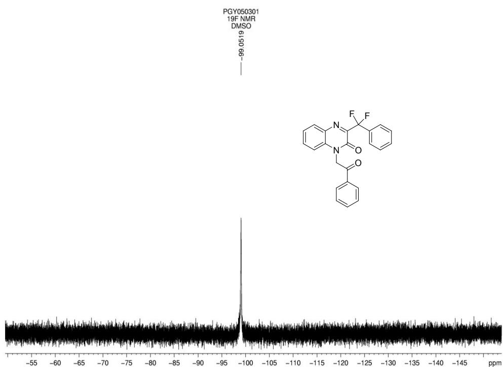
**Fig. S81** <sup>19</sup>F NMR spectrum of compound **3la**
