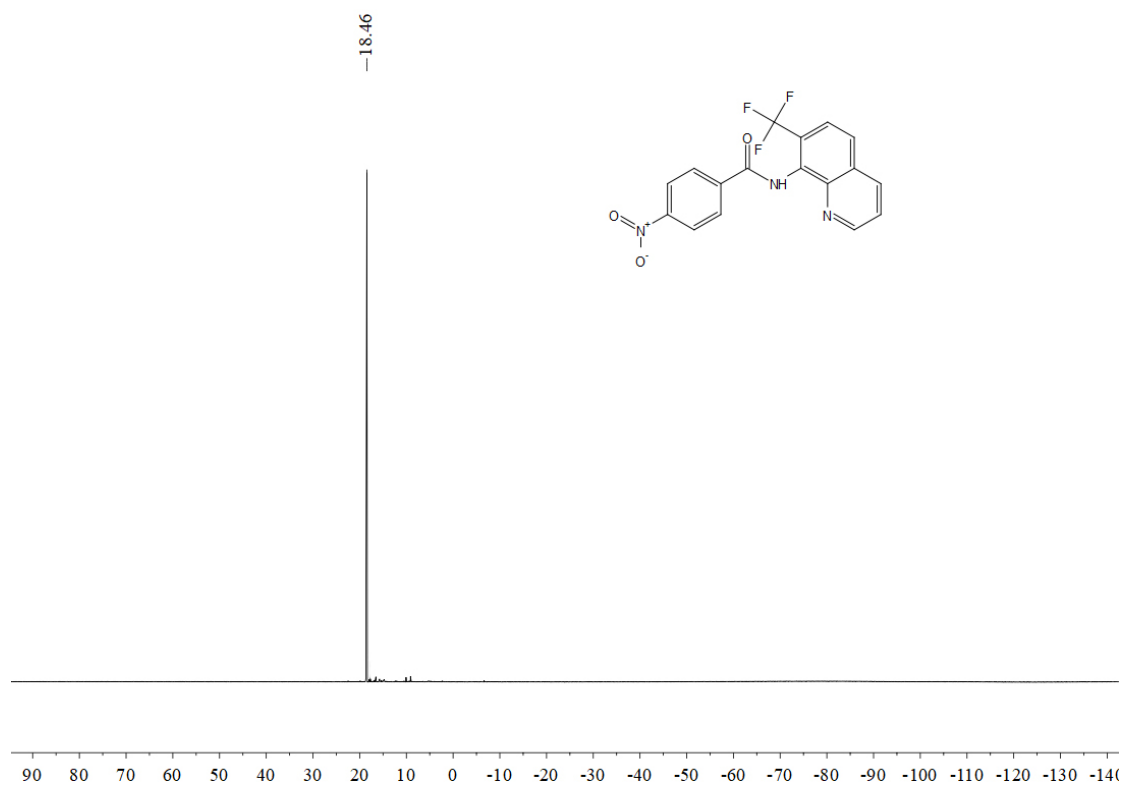
Figure S33. ^{19}\text{F} NMR of 4-nitro-N-(7-(trifluoromethyl)quinolin-8-yl)benzamide 2k .
