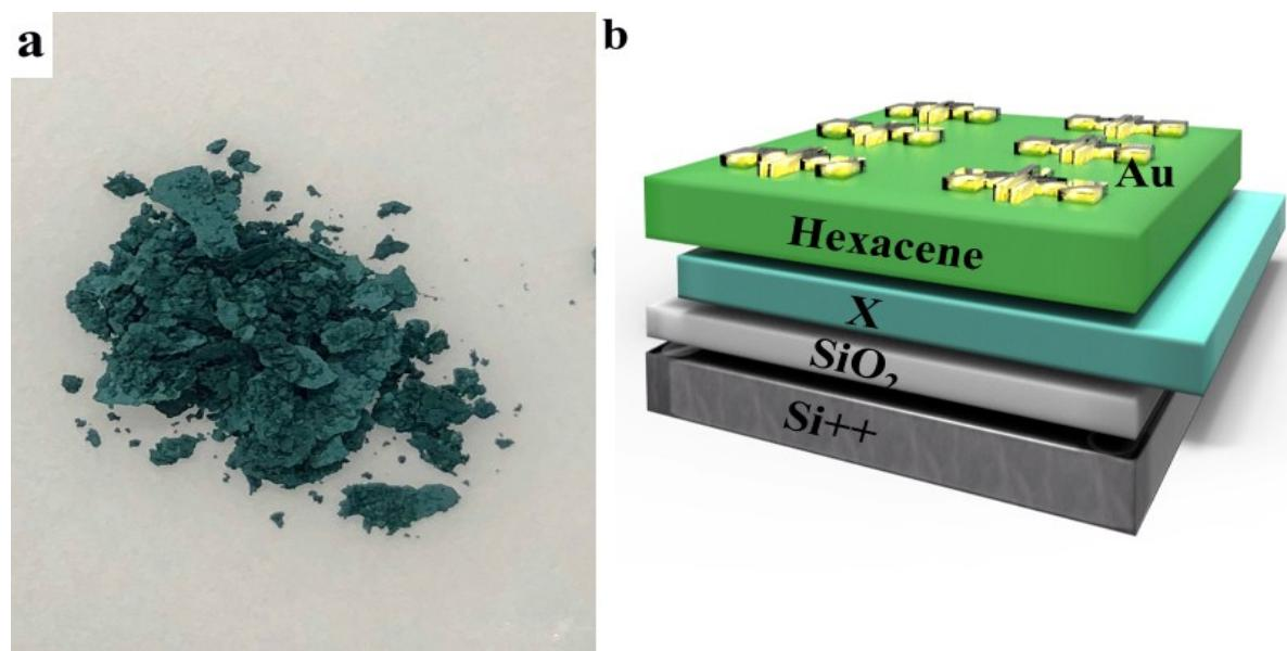
Figure S1 (a) Physical appearance of hexacene; (b) Schematic illustration of hexacene-based OFET device
