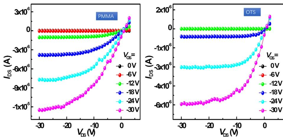
Figure S4 Output characteristics of the OFETs with different dielectric layers that measured in air at room temperature.
