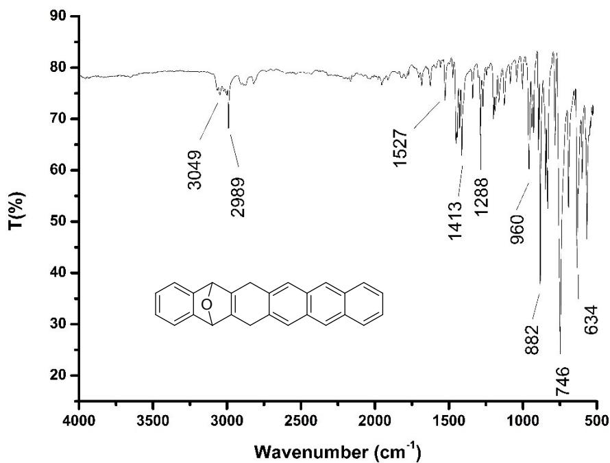
Figure S19 IR spectrum of compound 6
