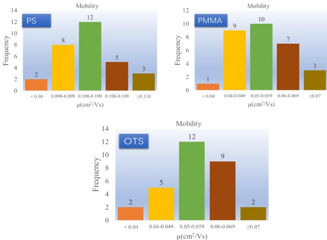
Figure S2 Statistic histograms for the field-effect hole mobilities of hexacene-based OFET devices
