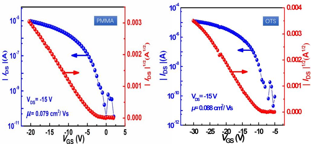
Figure S3 Transfer characteristics of the OFETs with different dielectric layers that exhibited the highest field effect mobility as measured in air at room temperature.
