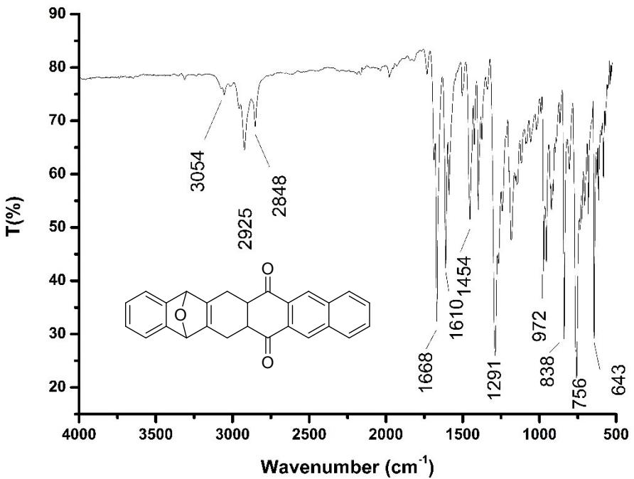
Figure S14 IR spectrum of compound 4
