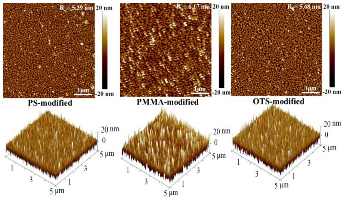
Figure S5 AFM images of hexacene deposited on PS, PMMA and OTS.
