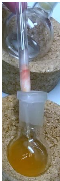
Figure SI- 18. Picture from the filtration with the 'mini column' based on a glass pipet filled with Celite® and silica.
