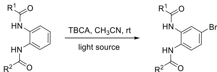
A 10 mL round-bottom flask equipped with a magnetic stir bar was charged with the unsymmetrical diamide (**1**, 0.40 mmol) and acetonitrile (3 mL) under open air conditions at room temperature, and two 100-watt household lights were arranged approximately 20 cm from the reaction. To the stirred solution was added
