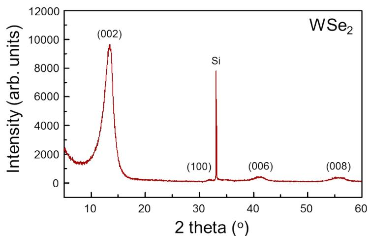
**Fig. S5** In-plane XRD pattern of the  $\text{WSe}_2$  crystal grown onto a  $\text{SiO}_2/\text{Si}$  substrate using a newly developed single source precursor.
