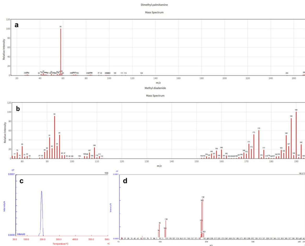
**Fig. S3** Mass spectra of  $(\text{CTA})_2[\text{WSe}_4]$  measured by TG-DTA-Mass. (a) Referred mass spectrum of dimethyl palmitamine (cetyl dimethyl amine). (b) Referred mass spectrum of dimethyl diselenide. (c) Graph of mass intensity with temperature change. The peak appeared at 183.8 to 196.0 °C when decomposed in TG-DTA. (d) Mass peak at the decomposition temperature.
