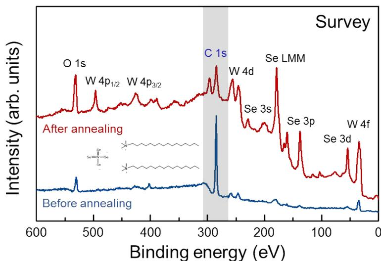
**Fig. S4** XPS survey spectra for  $(\text{CTA})_2[\text{WSe}_4]$  coated on  $\text{SiO}_2$  (300 nm)/ $\text{Si}(001)$  before and after annealing for the synthesis of  $\text{WSe}_2$  layers.
