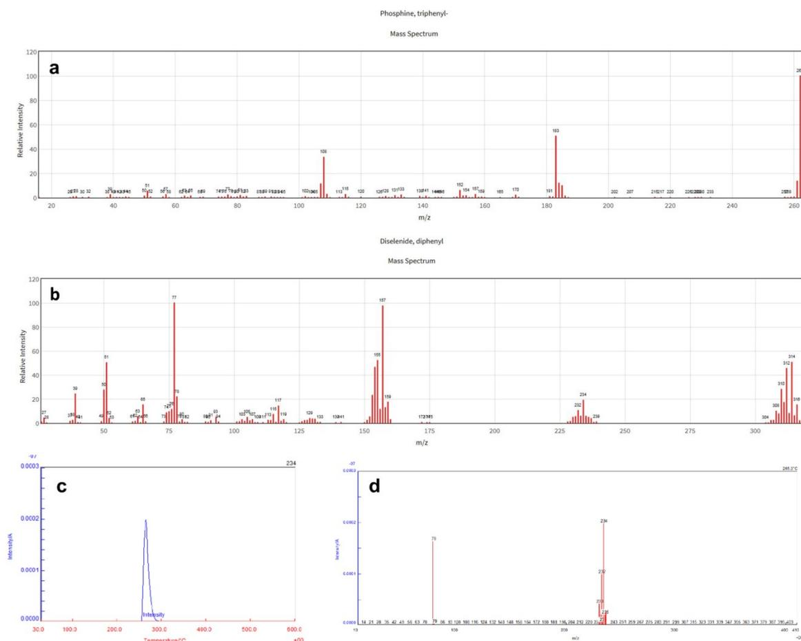
**Fig. S1** Mass spectra of  $(\text{Ph}_4\text{P})_2[\text{WSe}_4]$  measured by TG-DTA-Mass. (a) Referred mass spectrum of triphenyl phosphine. (b) Referred mass spectrum of diphenyl diselenide. (c) Graph of mass intensity with temperature change. The peak appeared at 260.4 to 270.6 °C when decomposed in TG-DTA. (d) Mass peaks at the decomposition temperature.
