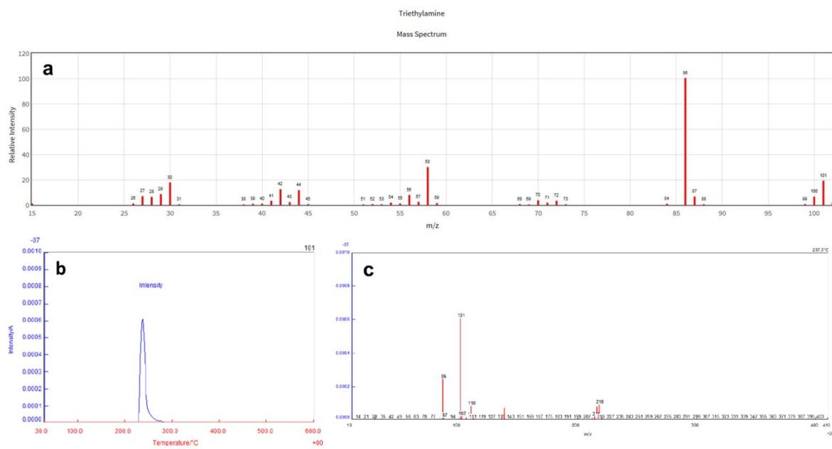
**Fig. S2** Mass spectra of  $(\text{Et}_4\text{N})_2[\text{WSe}_4]$  measured by TG-DTA-Mass. (a) Referred mass spectrum of triethylamine. (b) Graph of mass intensity with temperature change. The peak appeared at 234.8 to 239.5 °C when decomposed in TG-DTA. (c) Mass peaks at the decomposition temperature.
