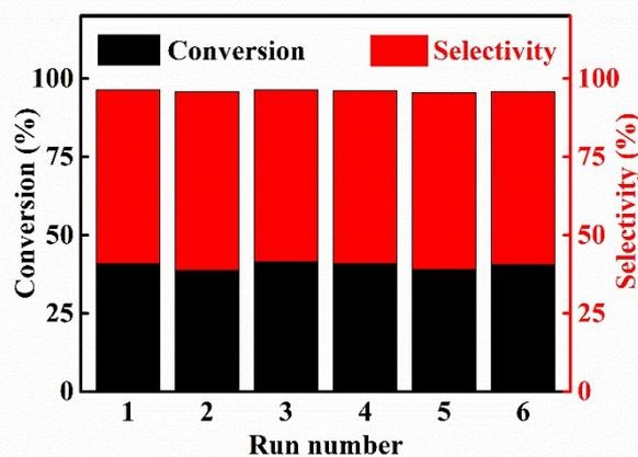
Fig. S5 Recyclable test of *nanoTS-1\_D* in the epoxidation of 1-hexene. (Even after 6 cycles, we can hardly see obvious loss in conversion or selectivity.)
