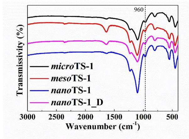
Fig. S3 FT-IR spectra of synthesized TS-1 zeolites.
