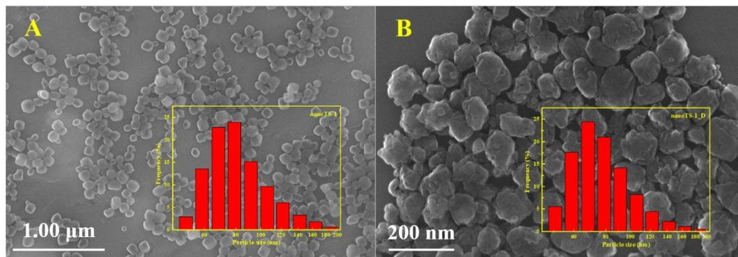
**Fig. S1** SEM images of synthesized *nano*TS-1 (A) and *nano*TS-1\_D (B). The insets in (A, B) are the Dynamic Light Scattering(DLS) particle size distributions.
