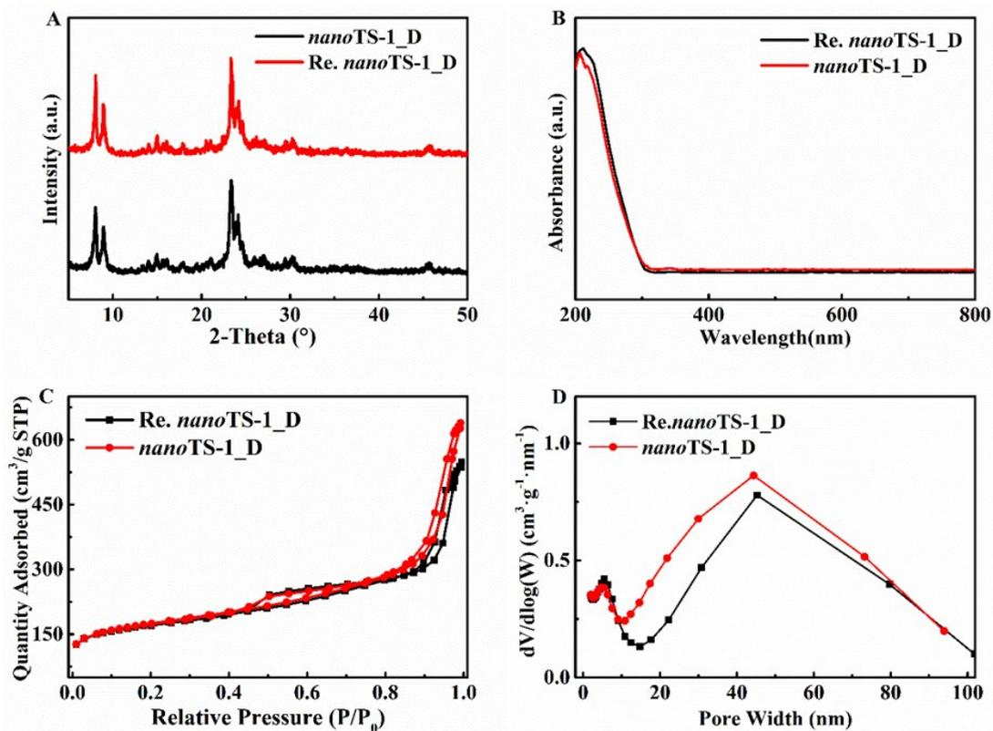
Fig. S4 (A) Powder XRD patterns, (B) UV-vis spectra, (C) N<sub>2</sub> sorption isotherms and (D) pore size distribution (PSD) of synthesized *nanoTS-1\_D* and *Re. nanoTS-1\_D*
