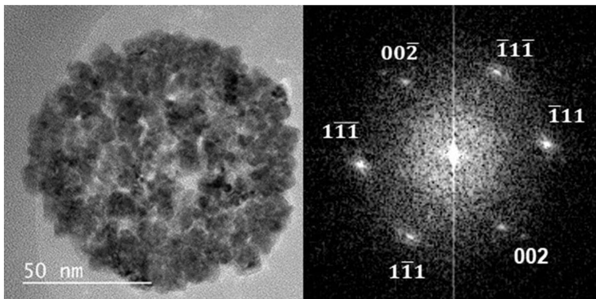
**Figure S2.** HR-TEM and FFT image of RhNP. RhNP exhibited highly crystalline fcc structure.
