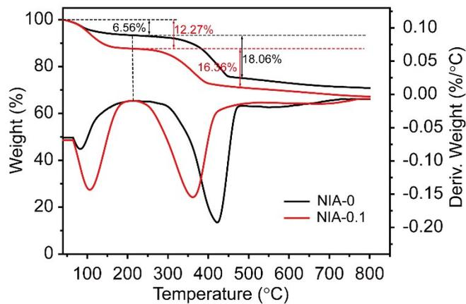
Figure. S2 TGA and DTG of NIA-0 and NIA-0.1 tested in air.
