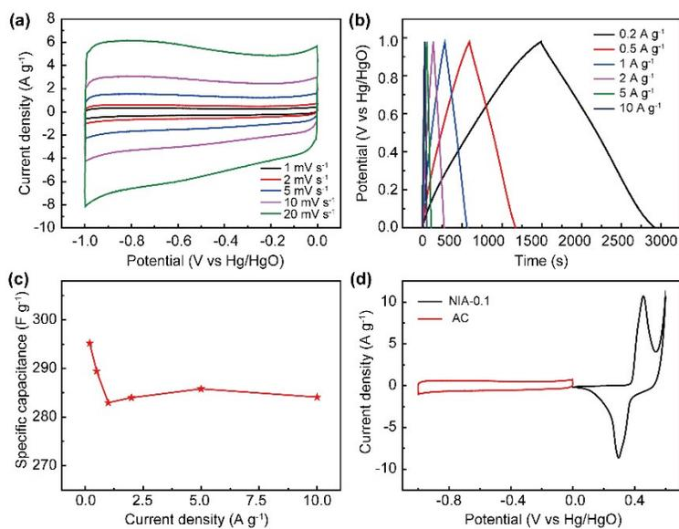
Figure. S5 (a) CV curves of HCP at scan rates from 1 to 20  $\text{mV s}^{-1}$ . (b) GCD curves of HCP at different current densities. (c) Specific capacitance values of HCP at different current densities. (d) Potential windows of NIA-0.1 and HCP at a scan rate of 2  $\text{mV s}^{-1}$ .
