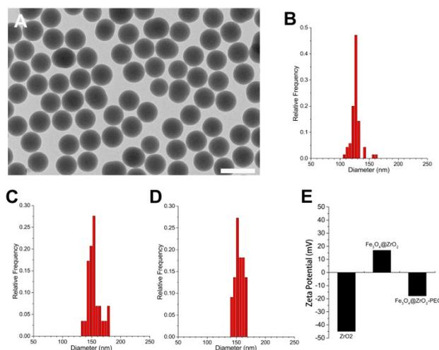
**Figure S1.** The structural characterization of samples. (A) TEM images of SiO<sub>2</sub> nanoparticles, scale bar represent 200 nm. Histogram of size distribution for the (B) SiO<sub>2</sub>, (C) ZrO<sub>2</sub> and (D) M-MZNs nanoparticles. (E) Zeta potentials of ZrO<sub>2</sub>, M-MZNs and M-MZNs-PEG.
