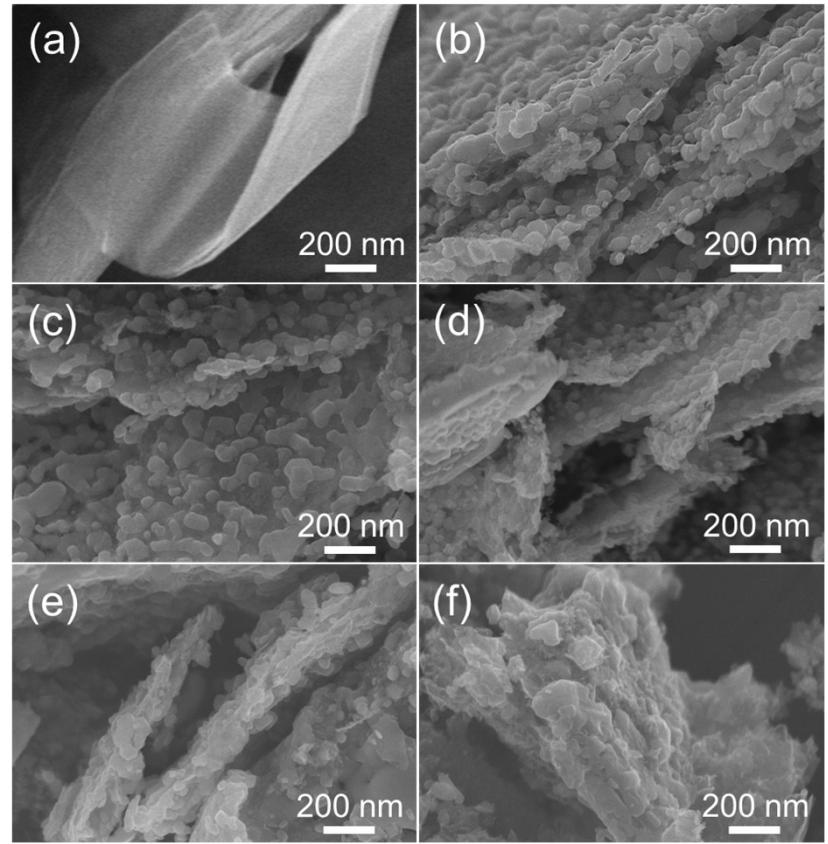
Fig. S3 SEM images of the pritine  $\text{Ti}_3\text{C}_2\text{T}_x$  MXene (a), FeNC/MXene-0.25 (b), FeNC/MXene-0.5 (c), FeNC/MXene-1 (d), FeNC/MXene-2.5 (e), and FeNC/MXene-5 (f) at high magnification.
