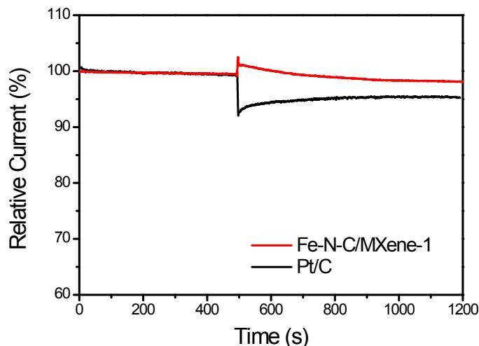
Fig. S9 Chronoamperometric responses of FeNC/MXene-1 and the Pt/C catalyst at 0.275 V in O<sub>2</sub><sup>-</sup>
