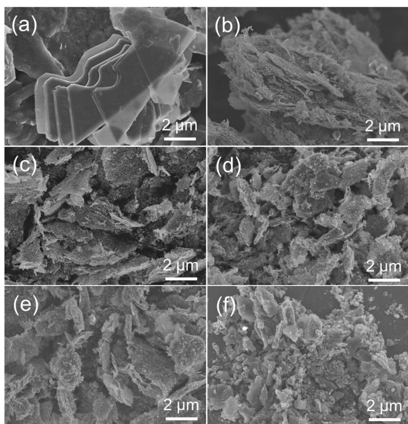
Fig. S2 SEM images of the pristine Ti<sub>3</sub>C<sub>2</sub>T<sub>x</sub> MXene (a), FeNC/MXene-0.25 (b), FeNC/MXene-0.5 (c), FeNC/MXene-1 (d), FeNC/MXene-2.5 (e), and FeNC/MXene-5 (f) at low magnification.
