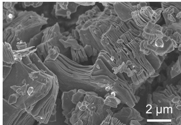
Fig. S1 SEM image of the multilayered Ti<sub>3</sub>C<sub>2</sub>T<sub>x</sub> powder.
