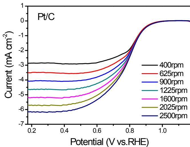
Fig. S7 LSV curves of the Pt/C catalyst in O<sub>2</sub>-saturated 0.1 M KOH solution at 50 mV·s<sup>-1</sup> with different rotating rates.
