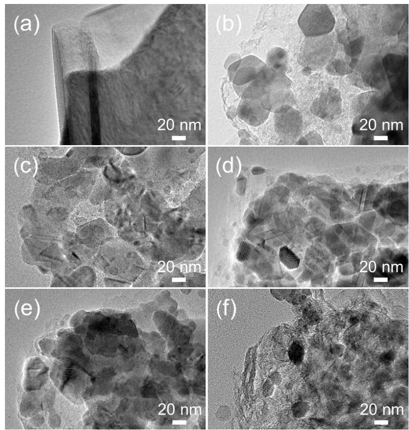
Fig. S4 TEM images of the pristine  $\text{Ti}_3\text{C}_2\text{T}_x$  MXene (a), FeNC/MXene-0.25 (b), FeNC/MXene-0.5 (c), FeNC/MXene-1 (d), FeNC/MXene-2.5 (e), and FeNC/MXene-5 (f).
