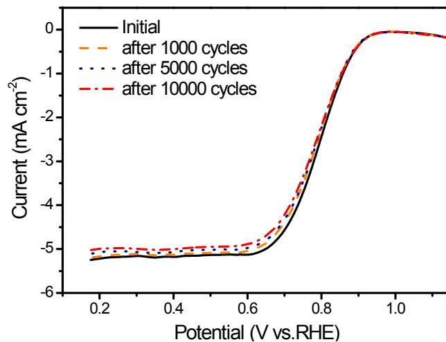
Fig. S8 LSV plots of FeNC/MXene-1 catalyst before and after the durability test over 10000 cycles at 1600 rpm.
