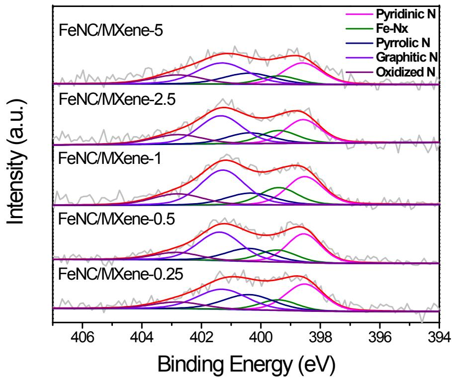
Fig. S5 XPS N1s binding energy regions of FeNC/MXene-x.
