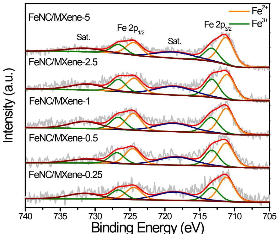
Fig. S6 XPS Fe2p binding energy regions of FeNC/MXene-x.
