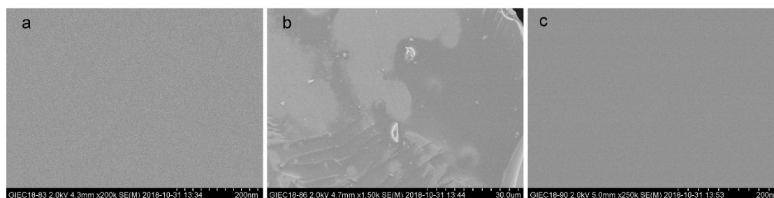
Fig. S9. The SEM images of UV-curable waterborne EPD films with different molar content of PA. (a) MWPA-PA66, scale:200 nm; (b) MWPA-PA39, scale:30 \mu\text{m} ; (c) MWPA-PA93, scale:200 nm.
