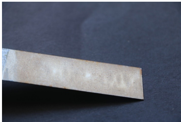
Fig. S13. Appearance of the corroded UV-curable EPD specimen surface with pure acrylic coatings (WPA).
