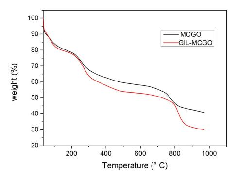
The curves for MCGO and GIL-MCGO at heating rate of 10°C per min in nitrogen.
