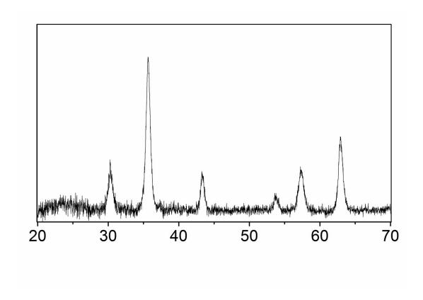
In the 20 range of 20°-70°, the six characteristic X-ray diffraction peaks for  $Fe_3O_4$  (20= 30.1°, 35.5°, 43.3°, 53.4°, 57.0°, and 62.6°), marked by their indices (2 2 0), (311), (4 0 0), (4 2 2), (511) and (4 4 0) are observed. The XRD patterns revealed that the synthesized process did not change the crystalline phase of  $Fe_3O_4$ .
