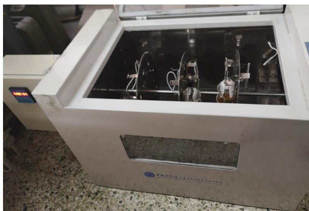
Figure S1. The self-made incubator with vertical rotary disc for enzymatic hydrolysis at high solid loading.
