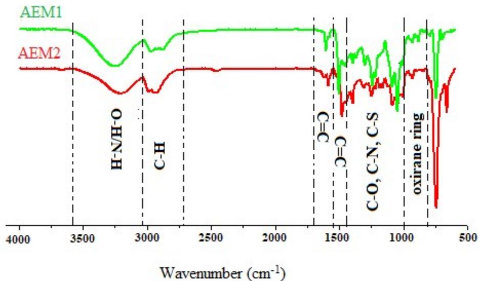
**Fig. SI 1.** ATR-FTIR spectra of AEM1 and AEM2
