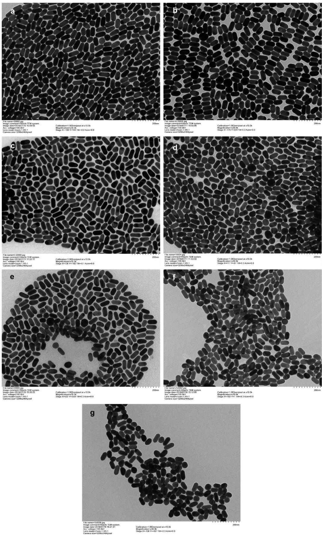
**Figure S1 (a-g)** TEM images of AuNRs after overgrowth at BSA concentrations of 0, 0.2, 0.5, 1, 2, 5, and 15 mM, respectively.
