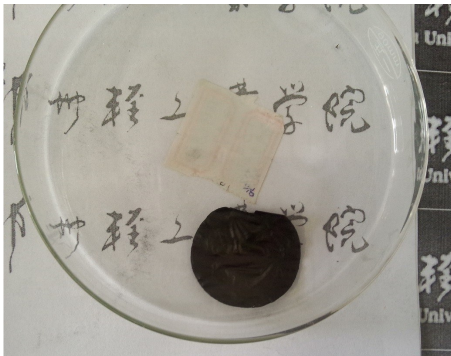
Fig. S2 The image of the generated highly wrinkled graphene film (HWGF)
