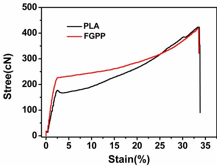
**Figure S7.** Tensile properties of the PLA and FGPP
