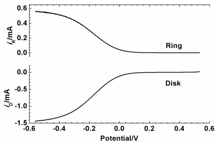
**Figure S1.** Ring ( $\text{Fe}^{2+} \rightarrow \text{Fe}^{3+} + \text{e}^-$ ) and disk ( $\text{Fe}^{3+} + \text{e}^- \rightarrow \text{Fe}^{2+}$ ) currents for the determination of collection efficiency of RRDE loaded with N-GC/Co@CoO/rGO catalyst. The electrolyte is degassed 0.1 M NaOH with 0.01 M  $\text{K}_3\text{Fe}(\text{CN})_6$ . The rotation speed of RRDE is 1,600 rpm. The collection efficiency is calculated to be  $(35.2 \pm 0.2)\%$ , which is close to the manufacturer's data 37%.
