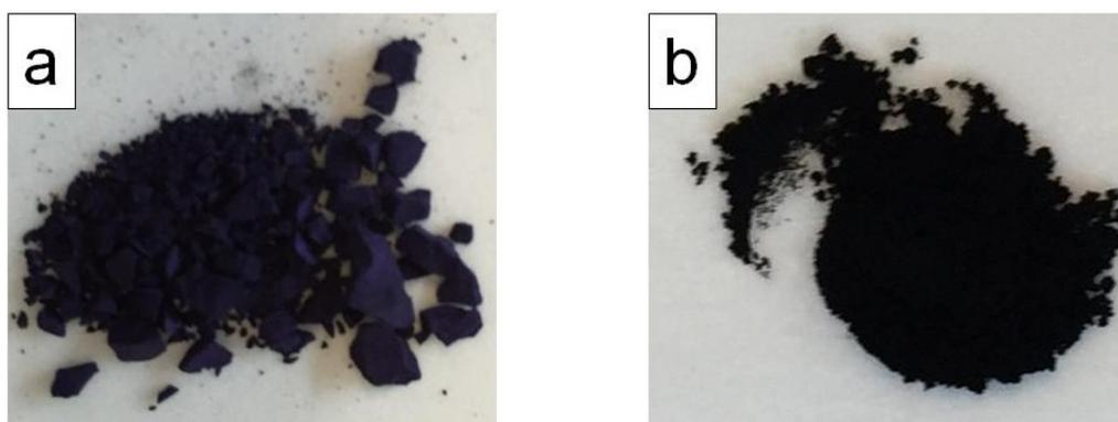
**Figure S2.** Digital pictures of (a) rGO-ZIF-67 and (b) N-GC/Co@CoO/rGO.
