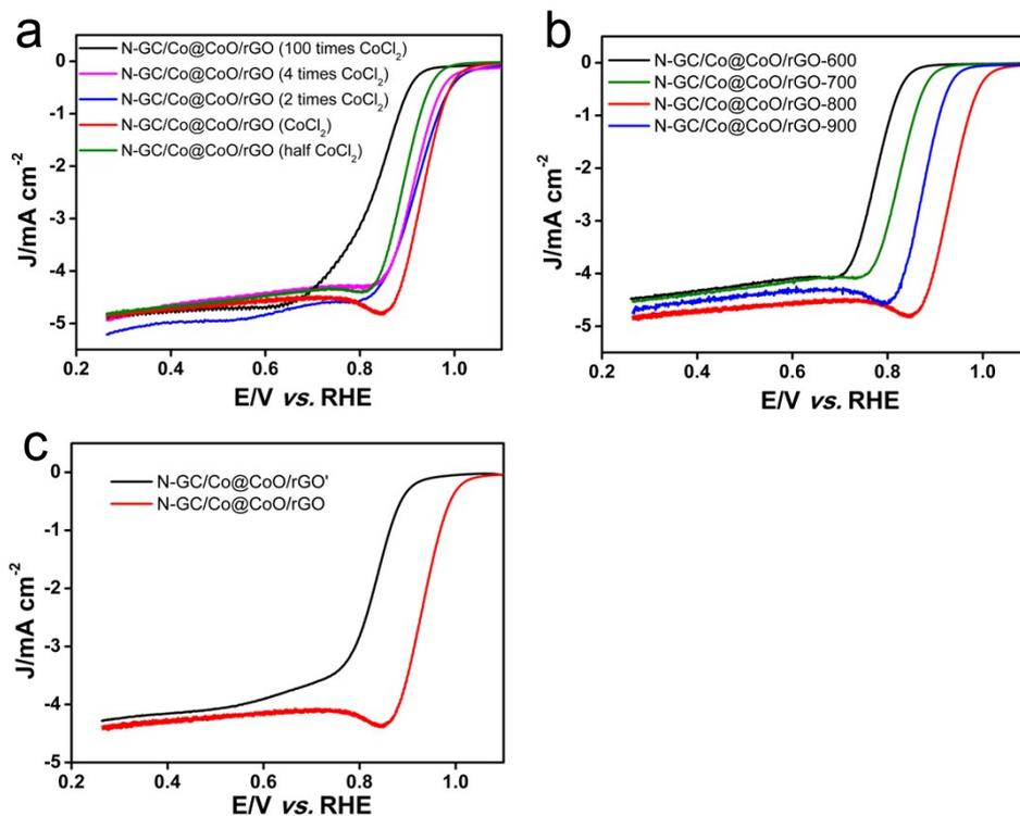
**Figure S5.** LSV curves of (a) N-GC/Co@CoO/rGO nanocomposite prepared with different molar ratios between GO and CoCl<sub>2</sub> precursors, (b) N-GC/Co@CoO/rGO nanocomposite carbonized under different temperature and (c) N-GC/Co@CoO/rGO nanocomposite prepared in our method and N-GC/Co@CoO/rGO' synthesized according to a previous report.<sup>[1]</sup> All of the curves were obtained at a rotation speed of 1,600 rpm in 0.1 M KOH.
