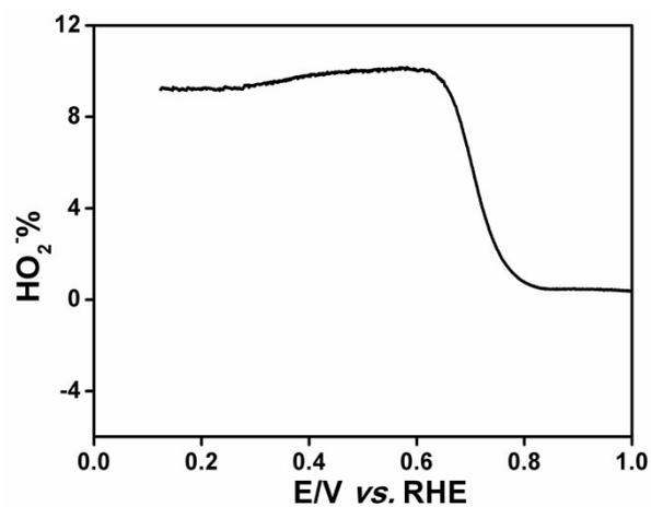
**Figure S7.** Calculation result of measured yield of HO<sub>2</sub><sup>-</sup> using K-L equation (see Experimental Section in detail) based on RRDE result (**Figure 4d**).
