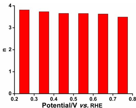
**Figure S6.** The number ( $n$ ) of electrons transferred per oxygen molecule (O<sub>2</sub>) during ORR for N-GC/Co@CoO/rGO obtained from its Koutecky-Levich plots shown in Figure 4c.
