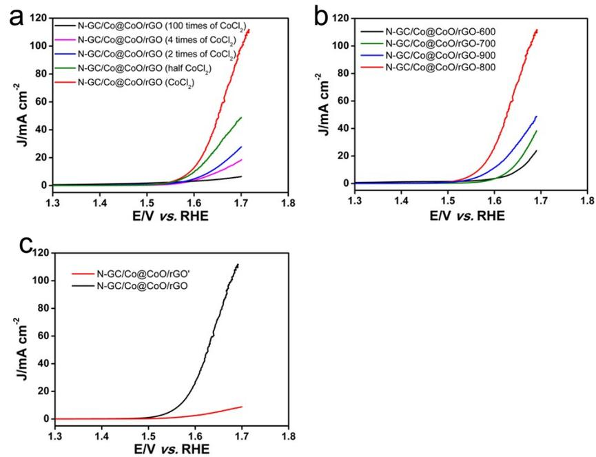
**Figure S9.** LSV curves of (a) N-GC/Co@CoO/rGO prepared with different molar ratios between GO and  $\text{CoCl}_2$  precursors, (b) N-GC/Co@CoO/rGO carbonized under different temperature and (c) N-GC/Co@CoO/rGO prepared in our method and N-GC/Co@CoO/rGO' synthesized according to a previous report<sup>1</sup> at a rotation speed of 1,600 rpm in 0.1 M KOH.
