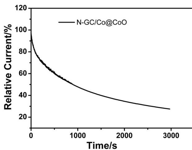
**Figure S8.** Chronoamperometric response of N-GC/Co@CoO at 0.7 V in O<sub>2</sub>-saturated 0.1 M KOH aqueous solution.
