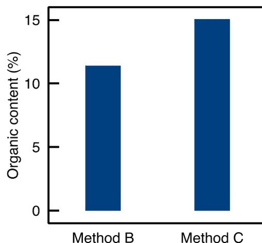
**Figure S3** – TGA analyses of A500<sub>B</sub> and A500<sub>C</sub> samples. More organic functions were detected on the rehydroxylated samples. This suggested that the rehydroxylation process allowed featuring more silanols at the surface.
