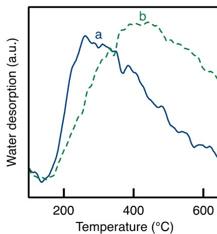
**Figure S2** – Thermo programmed water desorption of (a) Si(HIPE) and (b) rehydroxylated Si(HIPE).
