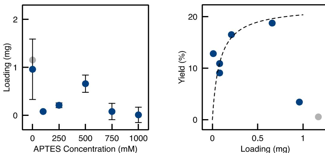
**Figure S4** – (Left) Enzyme loading as a function of the APTES concentration used for functionalization in Method D. (Right) BAP yield as a function of the enzyme loading for the samples prepared by Method D. Dotted curve is only a guide to the eye. Shaded dots (●) represents the yield and loading for TA-Si(HIPE) sample
