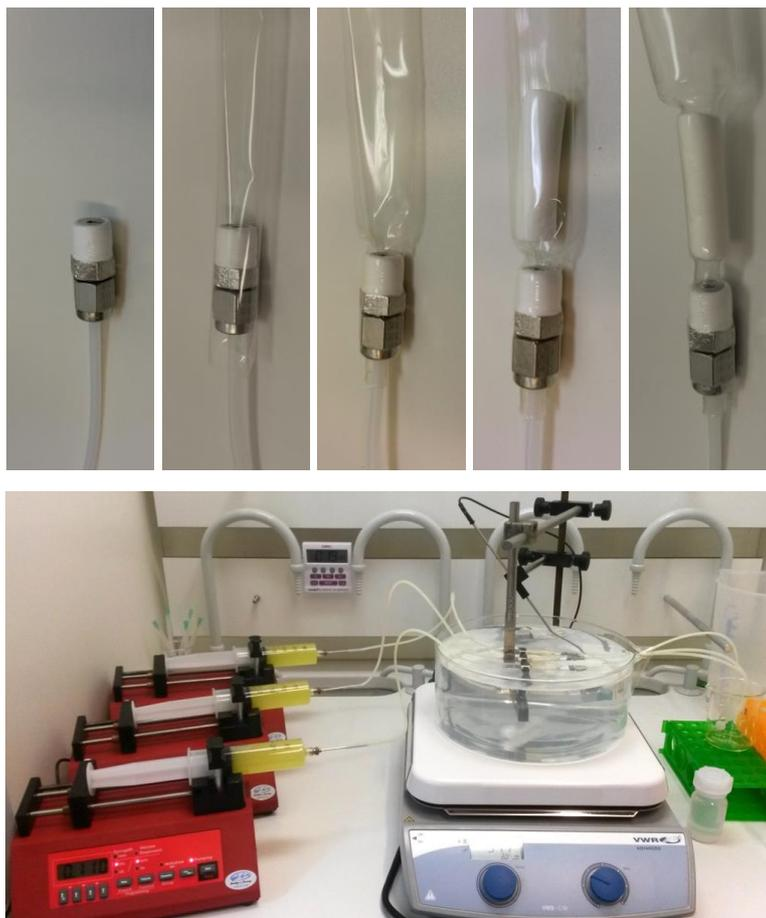
**Figure S1** – (top) Picture depicting the casting of the monolith into the heat-shrinkable Teflon tube and connexion wit the PTFE tubing. (bottom) Picture of the experimental set-up for flow reaction. Monolithic reactors are connected to syringe-pumps and outflow collectors via PTFE tubes. Monoliths are and immersed in a temperature-controlled water bath.
