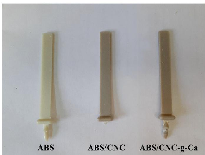
**Figure S7.** Injecton molded ABS samples with and without loading of cellulose nanocrystals
