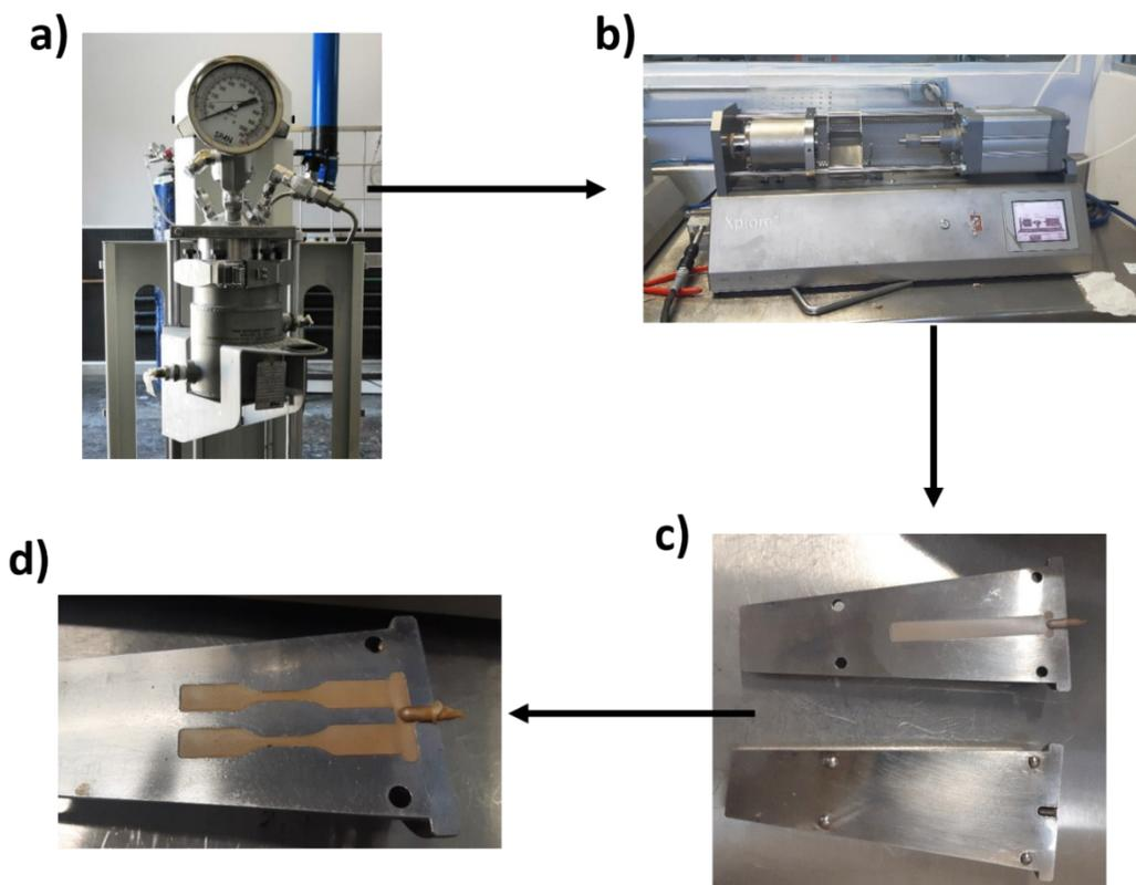
**Figure S6.** Schematic diagram of production of ABS/Nanocomposites: a) Stainless steel reactor (1 L capacity), equipped with an anchor-turbine stirrer used for the polymerization of ABS Nanocomposites; b) Xplore micro-injection moulder; c) Moulded sample of ABS/CNC; d) Moulded sample of ABS/CNC-g-Ca
