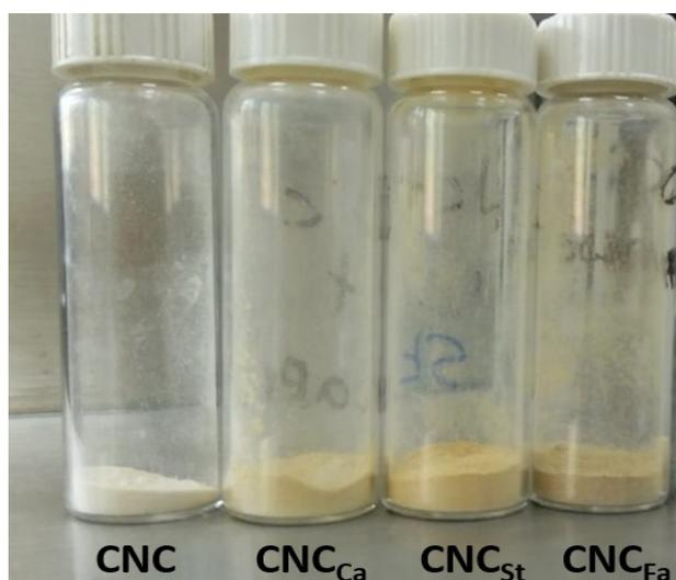
**Figure S2.** Photograph of cellulose nanocrystals before and after modification
