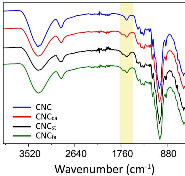
**Figure S3.** FTIR spectra of cellulose nanocrystals before and after plasma modification
