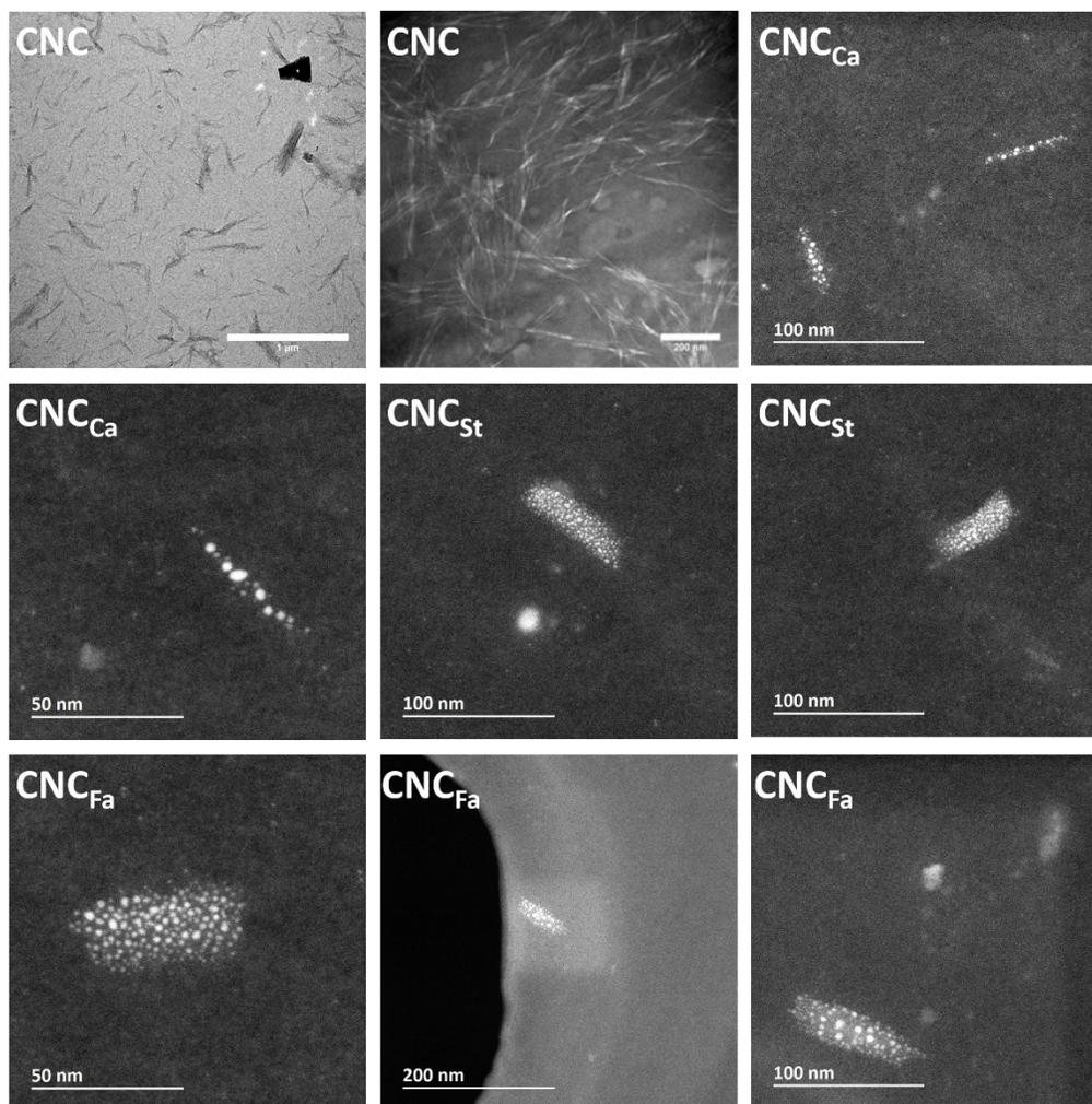
**Figure S4.** STEM micrographs of the cellulose nanocrystals before and after plasma modification
