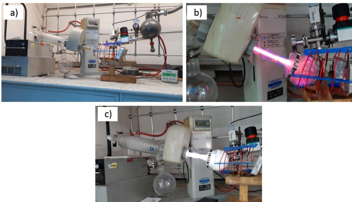
**Figure S1.** Photograph of the plasma reactor employed for the modification of the nanocrystals. A) Reactor before modification, B) Reaction test using an empty flask and air, C) Modification of CNC's using Caprolactone.
