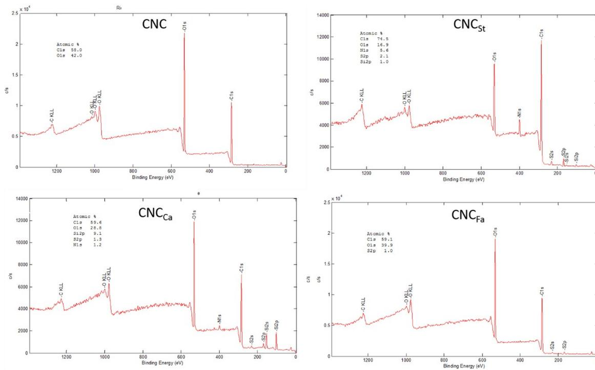
**Figure S5.** XPS survey of cellulose nanocrystals before and after modification
