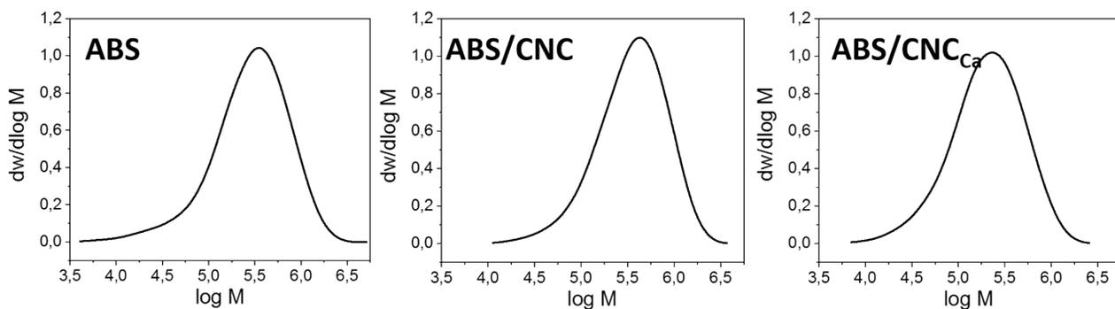
**Figure S8.** Size distribution of the different SAN copolymers in the synthesis of ABS/CNC nanocomposites
