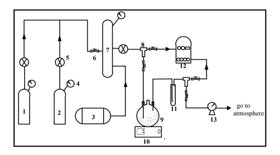
**Fig. S1.** Schematic diagram of the experimental apparatus of NO removal:(1) NO cylinder, (2)  $N_2$  cylinder, (3) air compressor, (4) piezometer, (5) rotameter, (6) valve, (7) buffer tank, (8) three-way pipe, (9) bubbling reactor, (10) electric heating-jacket, (11) drying tube, (12) flue gas analyzer, (13) wet gas meter.
