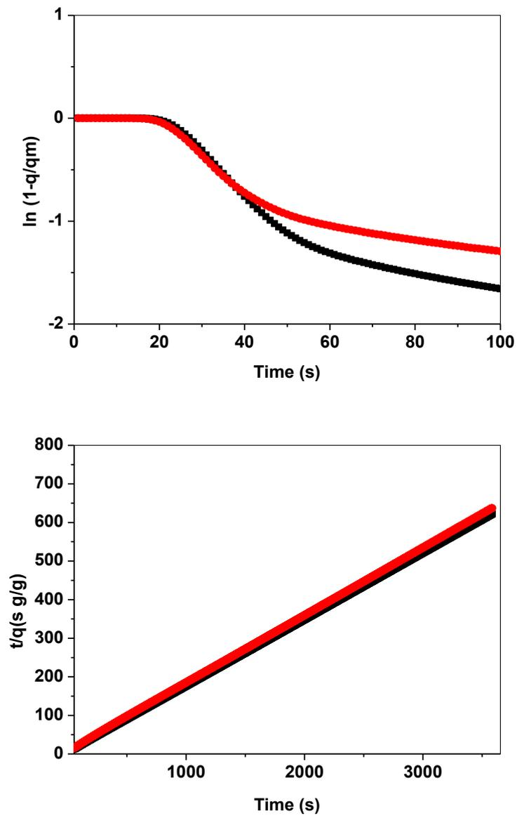
Figure S21. First (upper) and second (lower) order kinetic plot of CO<sub>2</sub> uptake on ACMO-4 during the first (black) and 23<sup>rd</sup> cycle (red)
