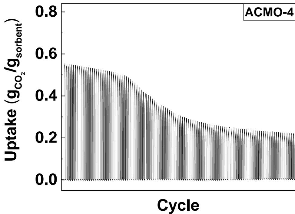
Figure S24. The CO<sub>2</sub> sorption cycles of ACMO-4, from 1 to 100<sup>th</sup> cycle
