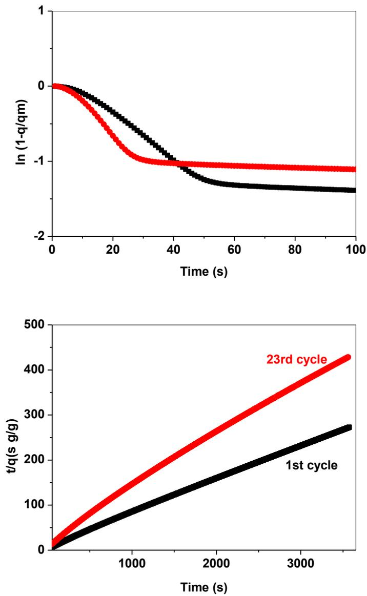
Figure S9. First (upper) and second (lower) order kinetic plot of CO<sub>2</sub> uptake on CMO-3 during the first (black) and 23<sup>rd</sup> cycle (red)
