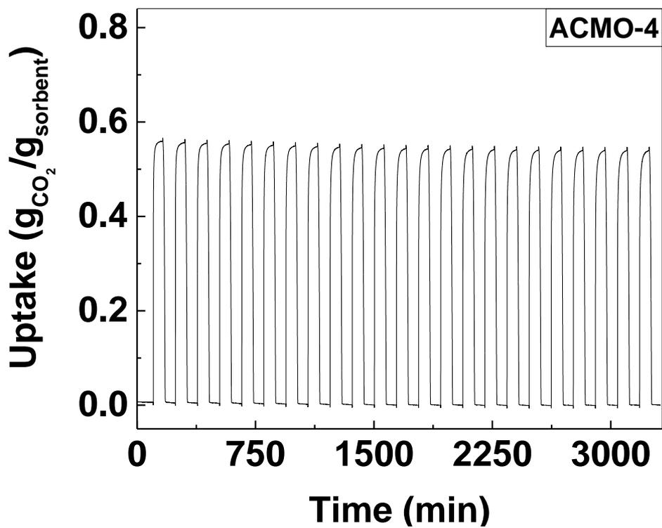
Figure S16. The CO<sub>2</sub> sorption cycles of ACMO-4, from 1 to 23<sup>rd</sup> cycle
