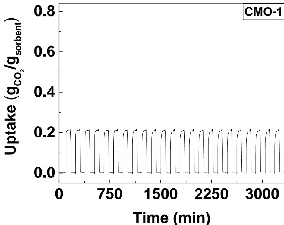
Figure S2. The CO<sub>2</sub> sorption cycles of CMO-1, from 1-23<sup>rd</sup> cycle
