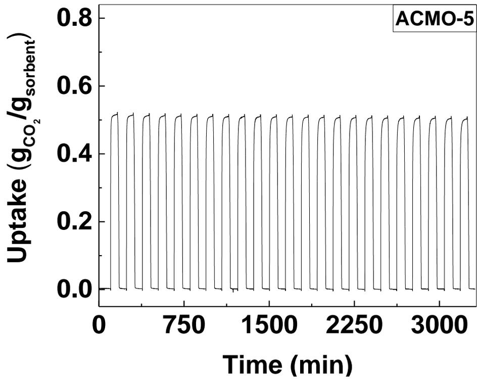
Figure S17. The CO<sub>2</sub> sorption cycles of ACMO-5, from 1 to 23<sup>rd</sup> cycle
