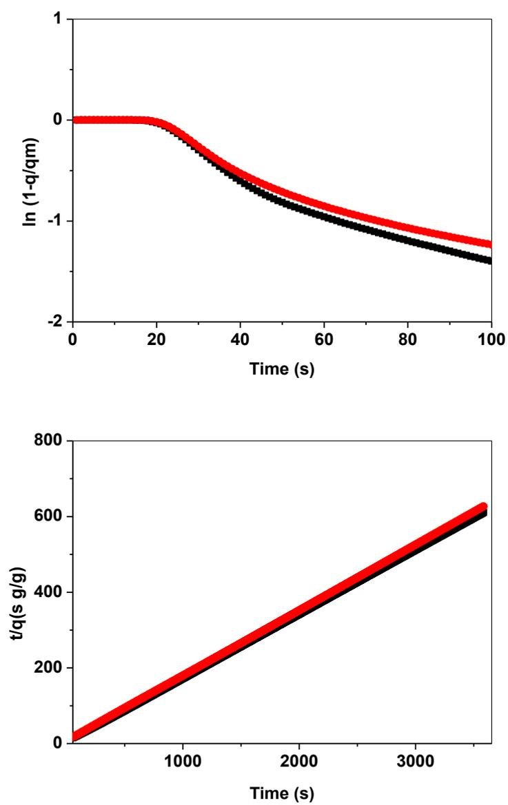
Figure S22. First (upper) and second (lower) order kinetic plot of CO<sub>2</sub> uptake on ACMO-5 during the first (black) and 23<sup>rd</sup> cycle (red)
