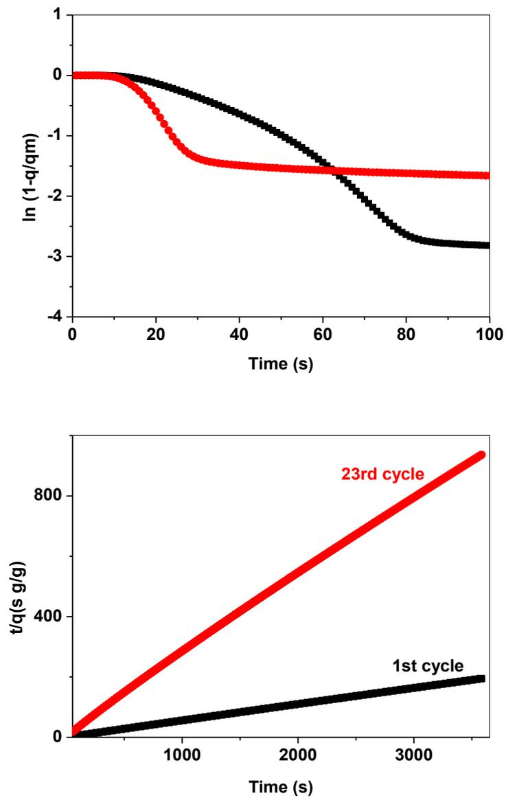
Figure S10. First (upper) and second (lower) order kinetic plot of CO<sub>2</sub> uptake on CaO-CaCO<sub>3</sub> during the first (black) and 23<sup>rd</sup> cycle (red)
