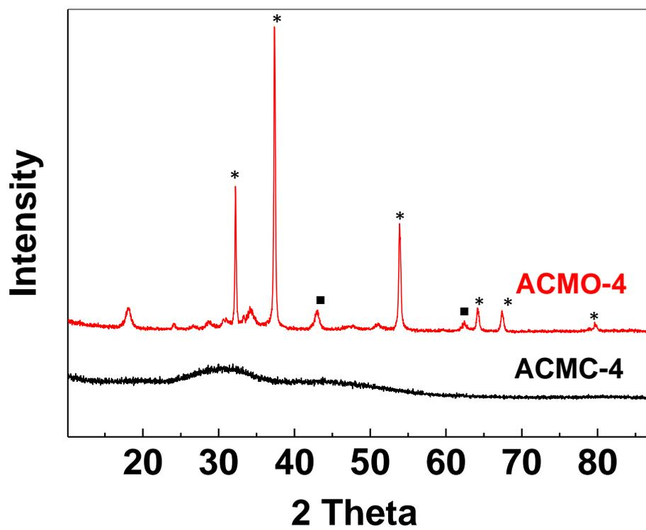
Figure S26. XRD before and after 100 adsorption cycles MgO (■), CaO (\*)
