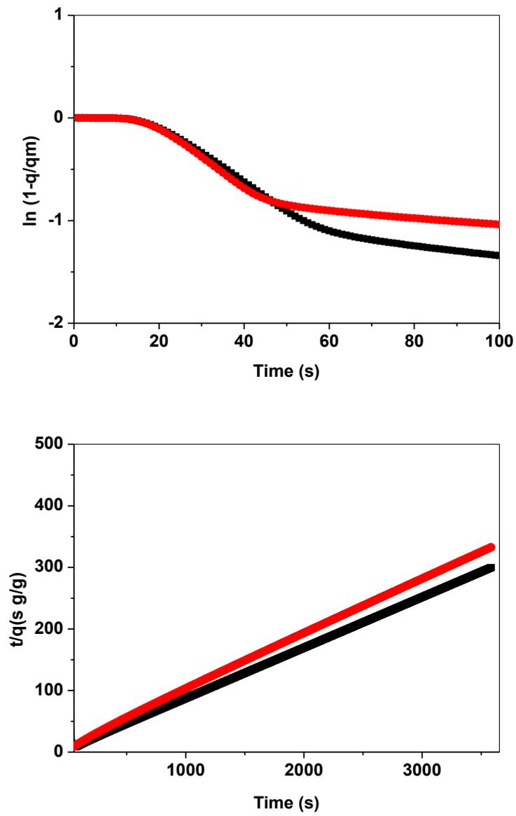
Figure S20. First (upper) and second (lower) order kinetic plot of CO<sub>2</sub> uptake on ACMO-3 during the first (black) and 23<sup>rd</sup> cycle (red)
