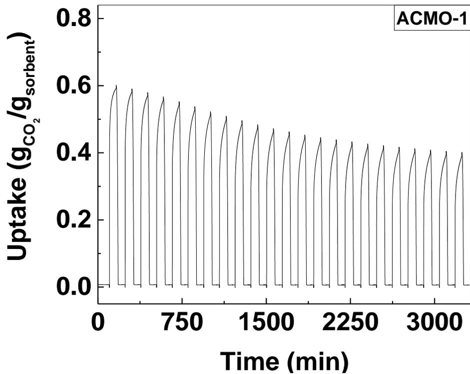
Figure S13. The CO<sub>2</sub> sorption cycles of ACMO-1, from 1 to 23<sup>rd</sup> cycle
