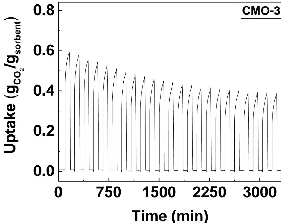
Figure S4. The CO<sub>2</sub> sorption cycles of CMO-3, from 1-23<sup>rd</sup> cycle
