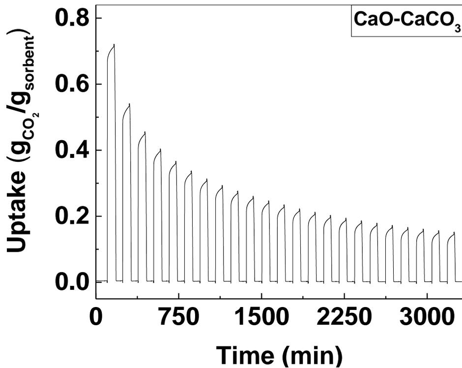
Figure S5. The CO<sub>2</sub> sorption cycles of CaO-CaCO<sub>3</sub>, from 1-23<sup>rd</sup> cycle
