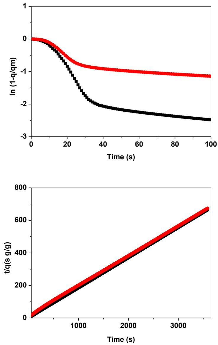
Figure S7. First (upper) and second (lower) order kinetic plot of CO<sub>2</sub> uptake on CMO-1 during the first (black) and 23<sup>rd</sup> cycle (red)
