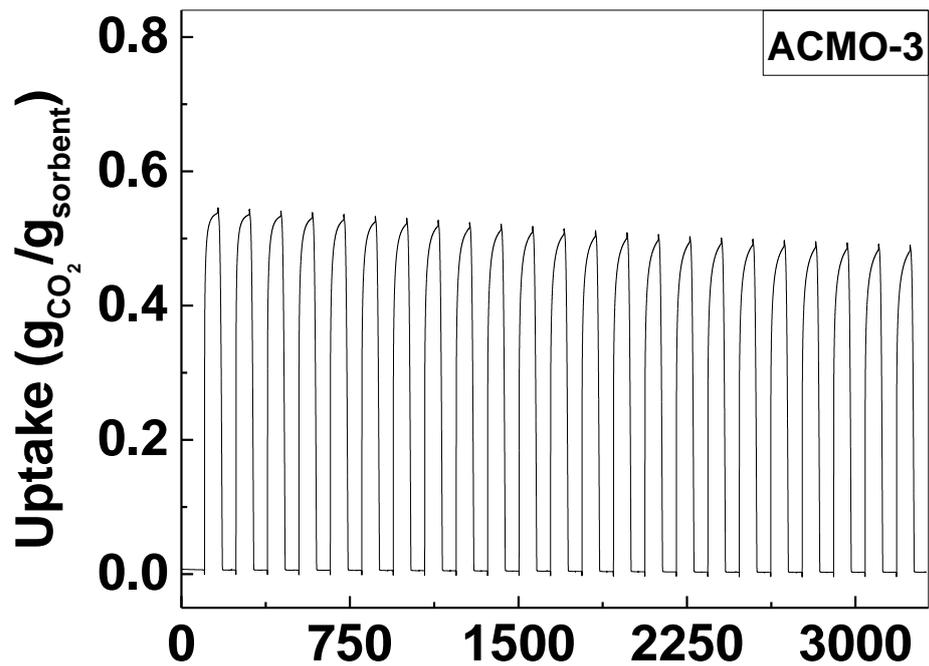
Figure S15. The CO<sub>2</sub> sorption cycles of ACMO-3, from 1 to 23<sup>rd</sup> cycle
