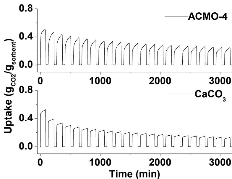
Figure S28. The CO<sub>2</sub> sorption cycles from a gas mixture (20% CO<sub>2</sub>, 80% N<sub>2</sub>) of ACMO-4 (top) and CaCO<sub>3</sub> (bottom), from 1 to 23<sup>rd</sup> cycle, the same gas mixture was used during CO<sub>2</sub> uptake at 650 °C and desorption at 850 °C
