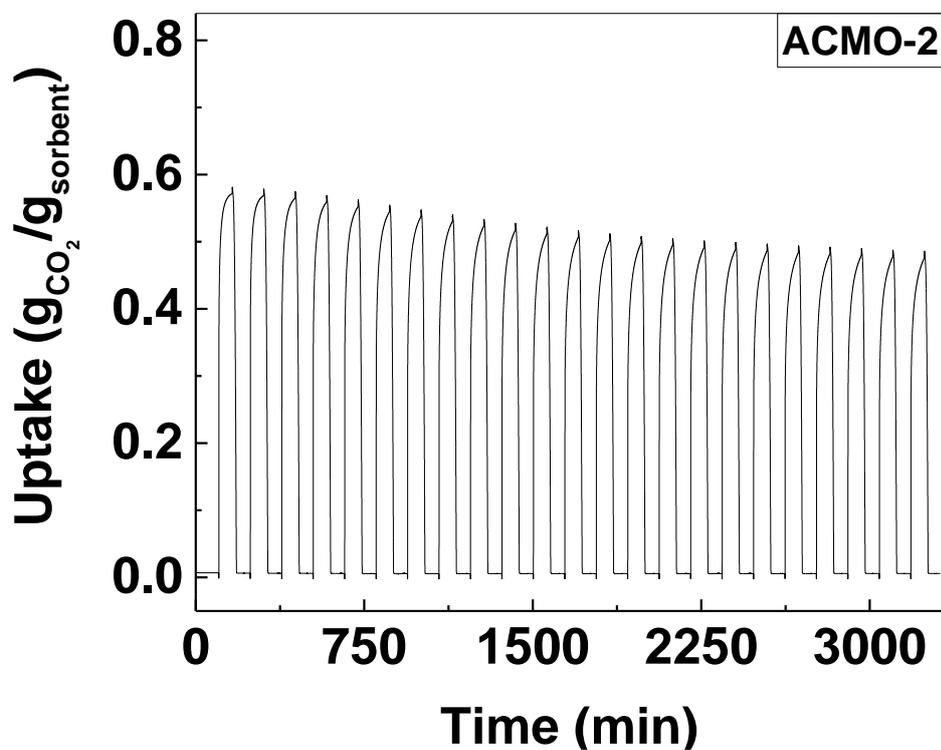
Figure S14. The CO<sub>2</sub> sorption cycles of ACMO-2, from 1 to 23<sup>rd</sup> cycle
