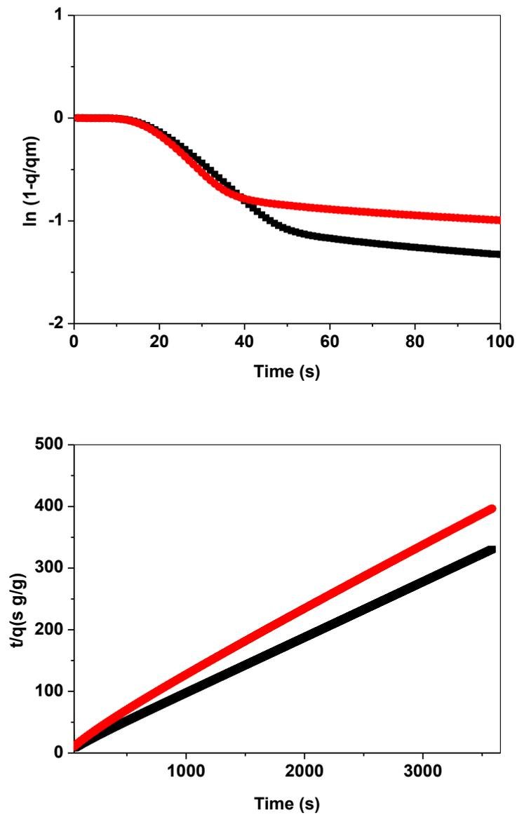
Figure S19. First (upper) and second (lower) order kinetic plot of CO<sub>2</sub> uptake on ACMO-1 during the first (black) and 23<sup>rd</sup> cycle (red)
