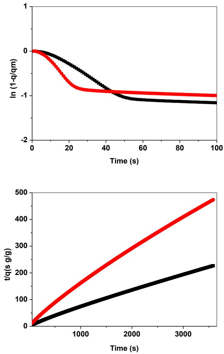
Figure S11. First (upper) and second (lower) order kinetic plot of CO<sub>2</sub> uptake on CaO-HPACC during the first (black) and 23<sup>rd</sup> cycle (red)
