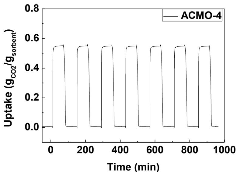
Figure S29. The CO<sub>2</sub> sorption cycles of ACMO-4, from 1 to 7<sup>th</sup> cycle where the CO<sub>2</sub> gas was mildly hydrated by bubbling through 5 water traps before being exposed to the ACMO-4 sorbent
