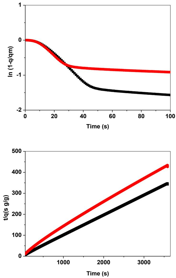
Figure S8. First (upper) and second (lower) order kinetic plot of CO<sub>2</sub> uptake on CMO-2 during the first (black) and 23<sup>rd</sup> cycle (red)
