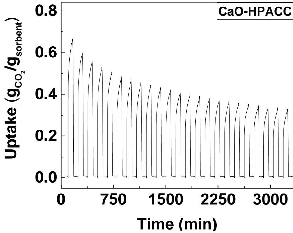
Figure S6. The CO<sub>2</sub> sorption cycles of CaO-HPACC, from 1-23<sup>rd</sup> cycle
