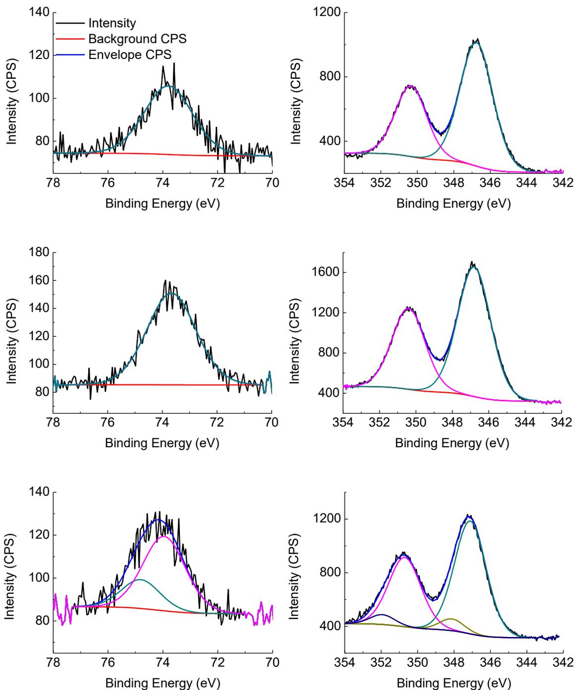
Figure S27. X-ray photoelectron spectra of a, b) ACMO-4 before CO<sub>2</sub> uptake experiments c,d) ACMO-4 after 23 cycles and e,f) ACMO-4 after 39 cycles, the Al 2p peak is shown in A,C and E, the Ca 2p peak is shown in B,D and F
