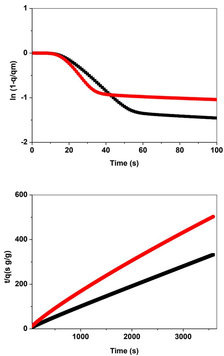
Figure S18. First (upper) and second (lower) order kinetic plot of CO<sub>2</sub> uptake on ACMO-1 during the first (black) and 23<sup>rd</sup> cycle (red)
