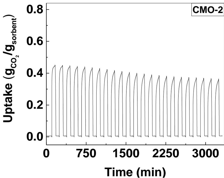
Figure S3. The CO<sub>2</sub> sorption cycles of CMO-2, from 1-23<sup>rd</sup> cycle
