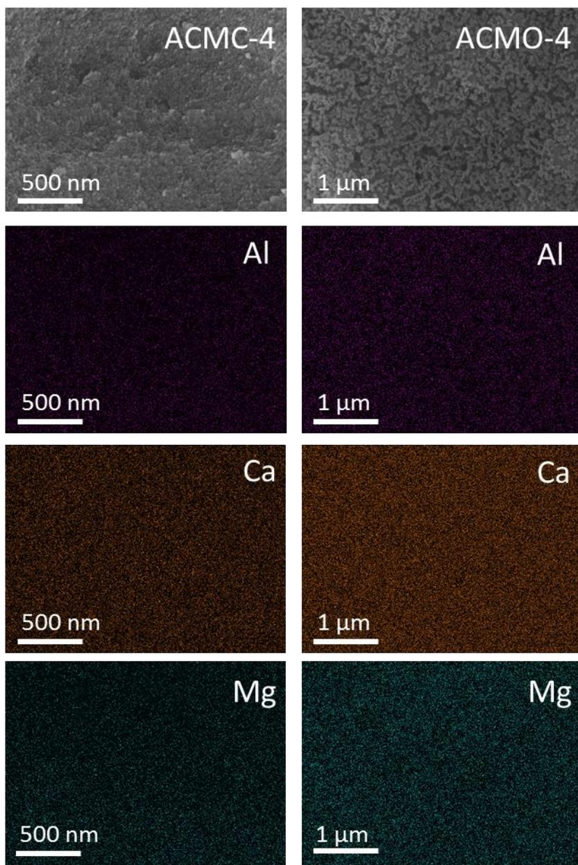
Figure S23. EDX mapping of the Al, Ca and Mg on ACMC-4 and ACMO-4
