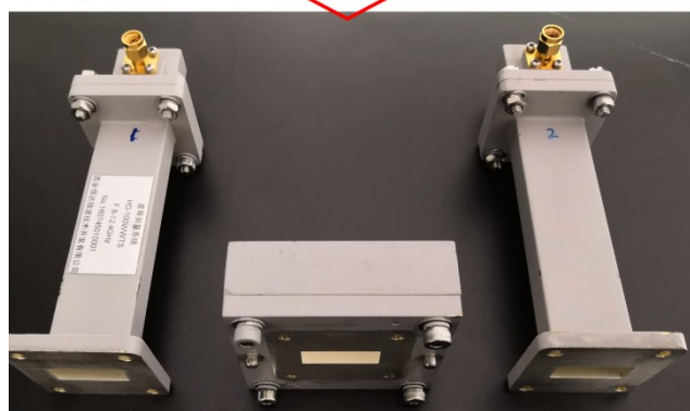
Fig. S1 Digital pictures of experimental setup and the sample holder for testing of shielding property.
