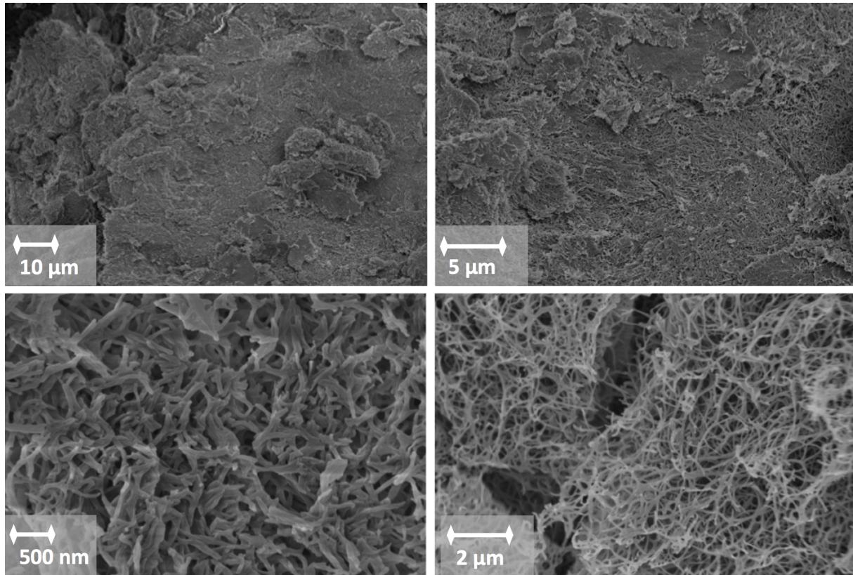
**Fig. S9** Additional FESEM pictures of a xerogel prepared from **C<sub>12</sub>-Cyc** ( $c = 20 \text{ g L}^{-1}$ ) in cyclohexane.
