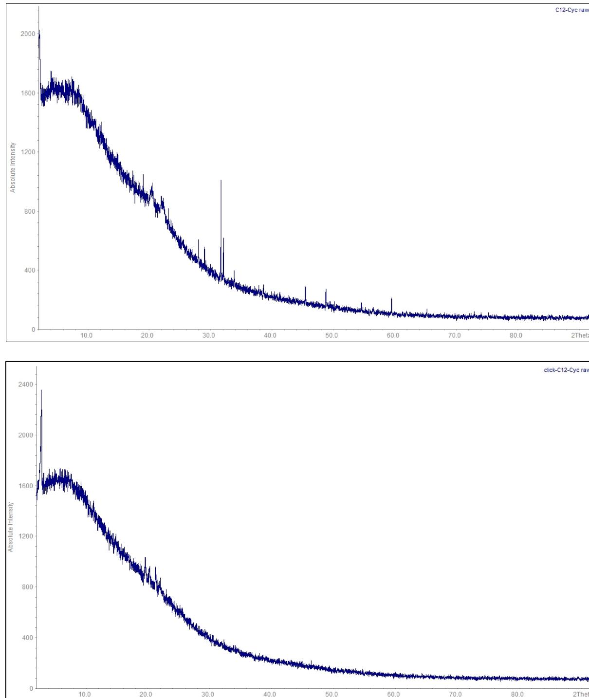
**Fig. S19** XRD spectra of raw **C<sub>12</sub>-Cyc** (*top*) and raw **click-C<sub>12</sub>-Cyc** (*bottom*) as the compounds were recrystallized from acetone during the synthesis.
