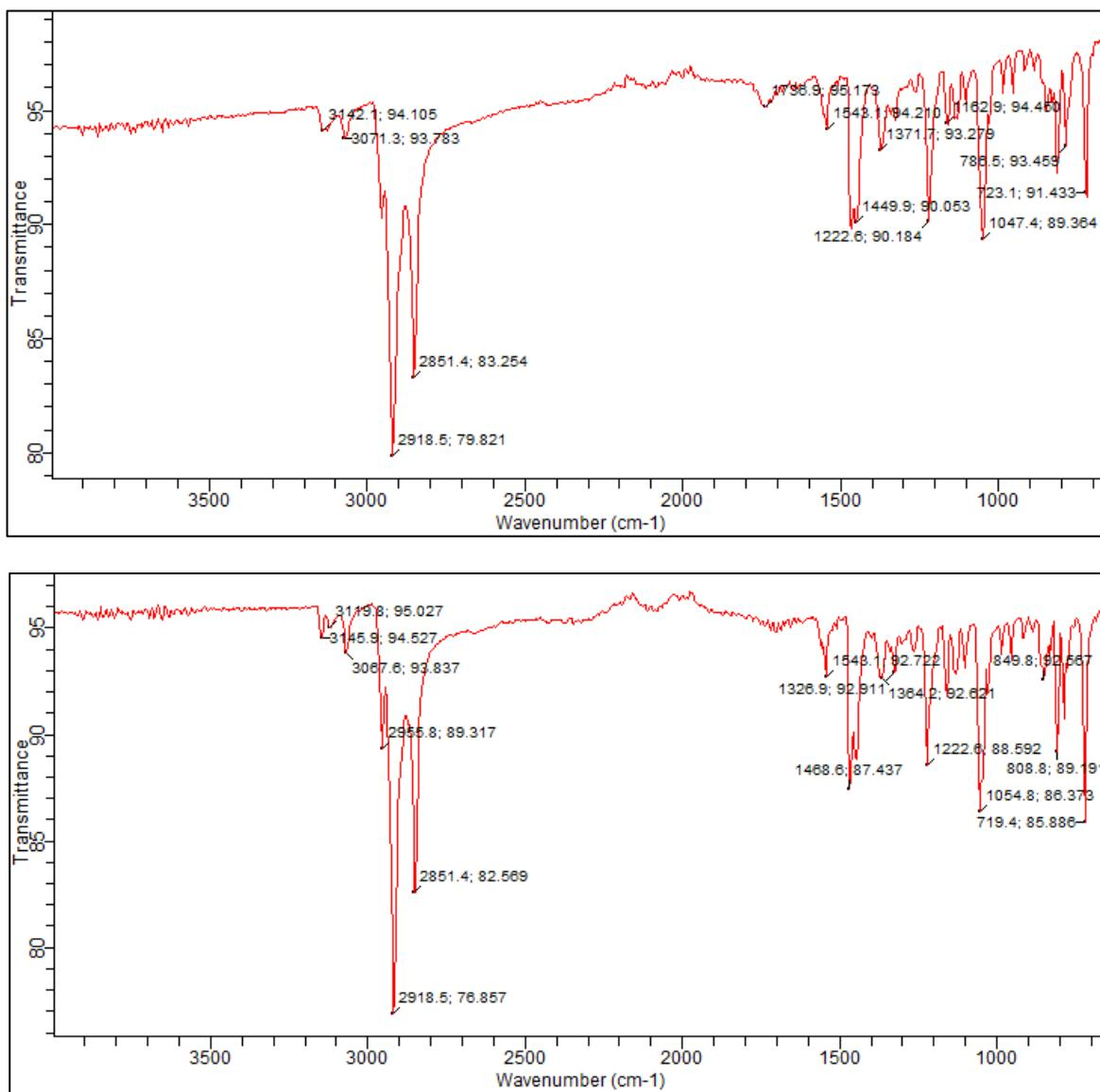
**Fig. S18** FT-IR spectra of **click-C<sub>12</sub>-Cyc** xerogel in cyclohexane ( $c = 15 \text{ g L}^{-1}$ ) (top) and **click-C<sub>12</sub>-Cyc** xerogel in nitromethane ( $c = 20 \text{ g L}^{-1}$ ) (bottom).
