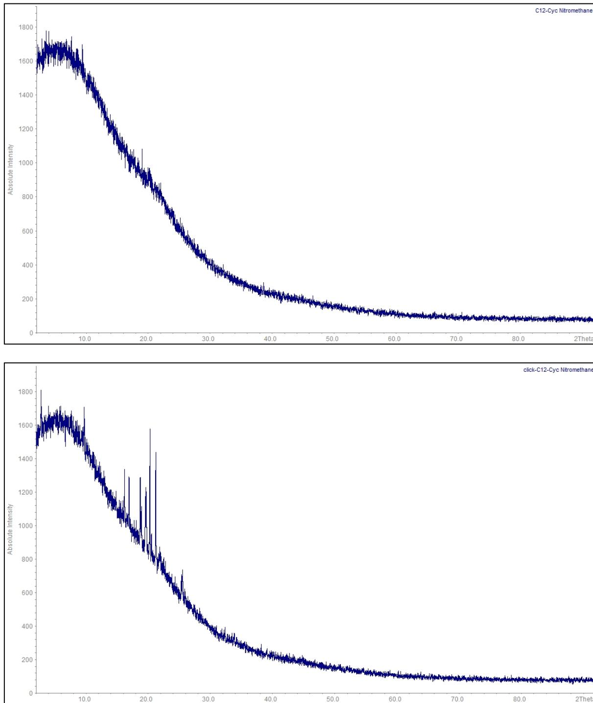
**Fig. S21** XRD spectra of **C<sub>12</sub>-Cyc** ( $c = 20 \text{ g L}^{-1}$ ) (top) and **click-C<sub>12</sub>-Cyc** ( $c = 20 \text{ g L}^{-1}$ ) (bottom) xerogels in nitromethane.
