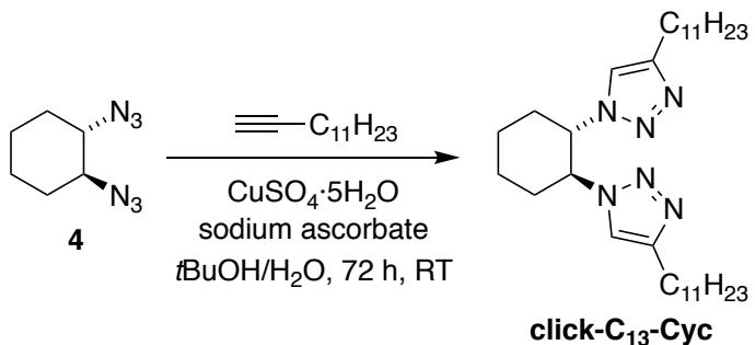
**Scheme 2.** Synthetic scheme for the preparation of (1*S,2S*)-1,2-bis(4-undecyl-1*H*-1,2,3-triazol-1-yl)cyclohexane (**click-C<sub>13</sub>-Cyc**).
