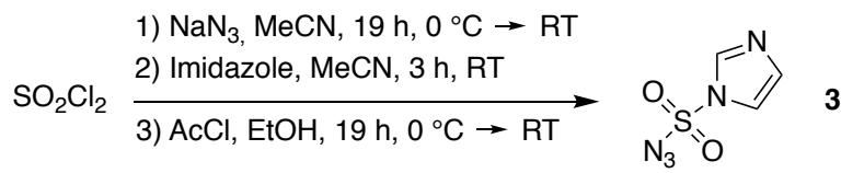
**Scheme 1.** Synthetic scheme for the preparation of 1*H*-imidazole-4-sulfonyl azide (**3**).
