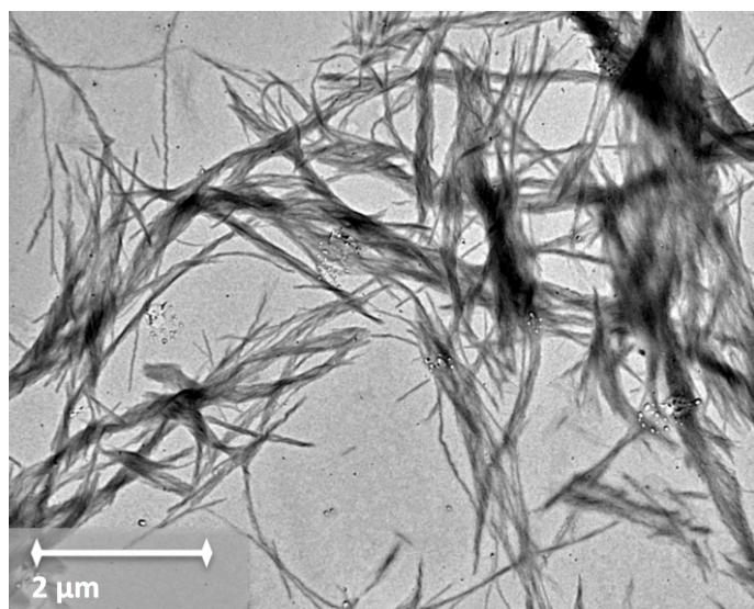
**Fig. S10** Representative TEM image of the gel made of **C<sub>12</sub>-Cyc** ( $c = 20 \text{ g L}^{-1}$ ) in cyclohexane.
