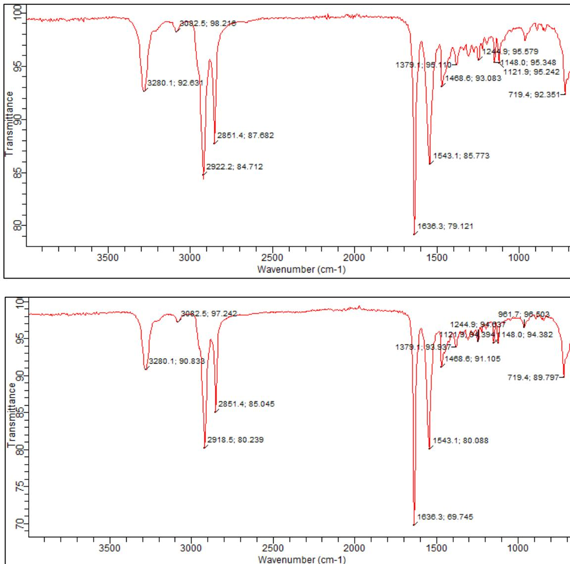
**Fig. S17** FT-IR spectra of **C<sub>12</sub>-Cyc** xerogel in cyclohexane ( $c = 15 \text{ g L}^{-1}$ ) (top) and **C<sub>12</sub>-Cyc** xerogel in nitromethane ( $c = 20 \text{ g L}^{-1}$ ) (bottom).
