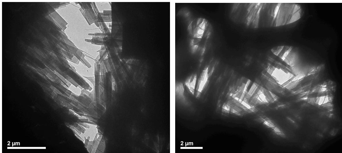
**Fig. S14** Representative TEM images of gels made of **click-C<sub>12</sub>-Cyc** ( $c = 30 \text{ g L}^{-1}$ ) in nitromethane.
