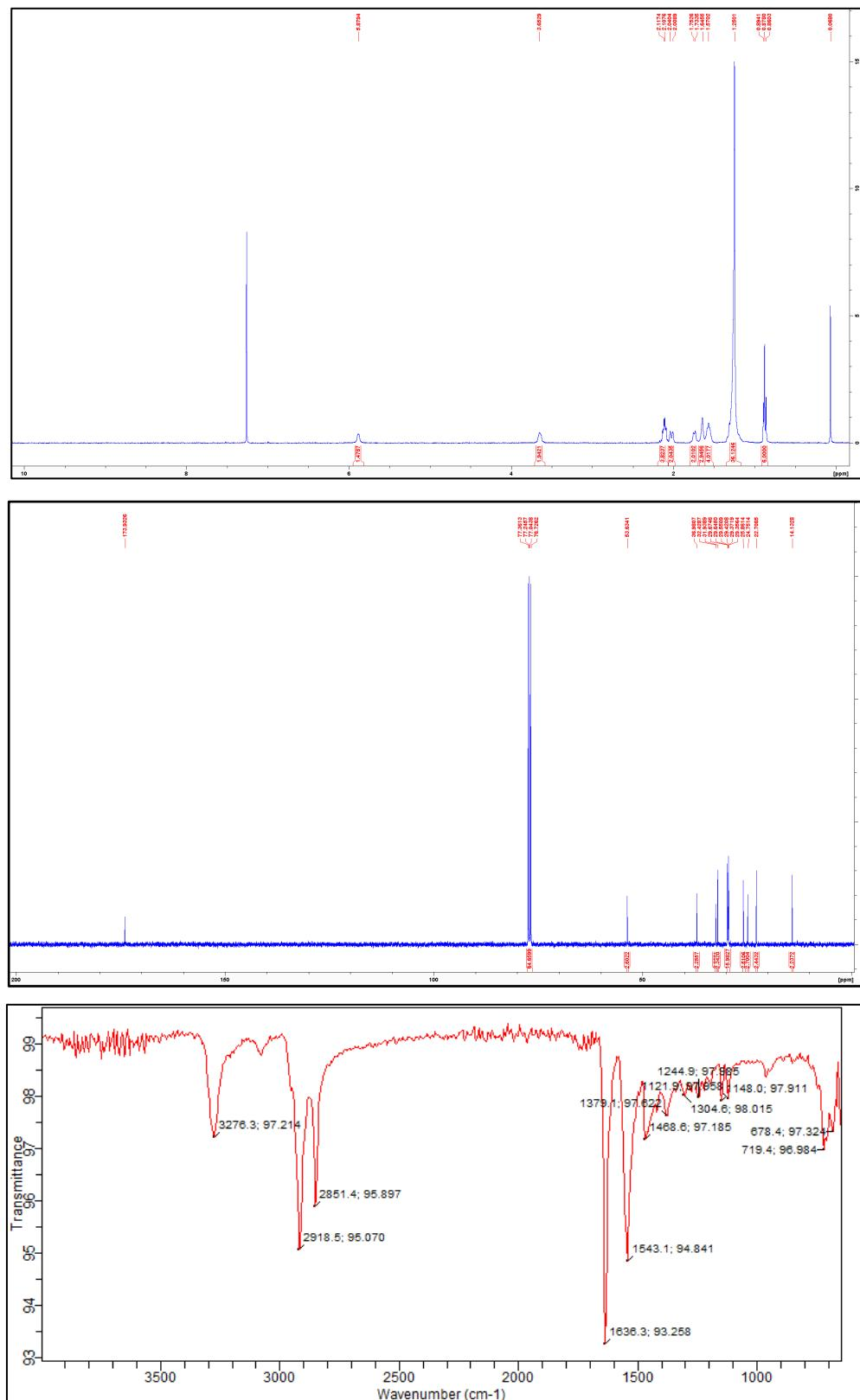
**Fig. S2**  $^1\text{H}$  NMR (top),  $^{13}\text{C}$  NMR (middle), FT-IR (bottom) spectra of C<sub>12</sub>-Cyc. NMR spectra were made in CDCl<sub>3</sub>.
