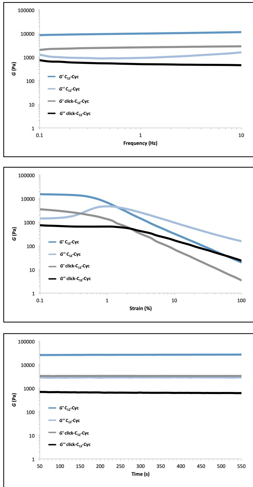
**Fig. S16** Oscillatory rheological experiments of gels prepared from **C<sub>12</sub>-Cyc** and **click-C<sub>12</sub>-Cyc** in cyclohexane ( $c = 20 \text{ g L}^{-1}$ ). *Top:* DFS-plots. *Middle:* DSS-plots. *Bottom:* DTS-Plots.
