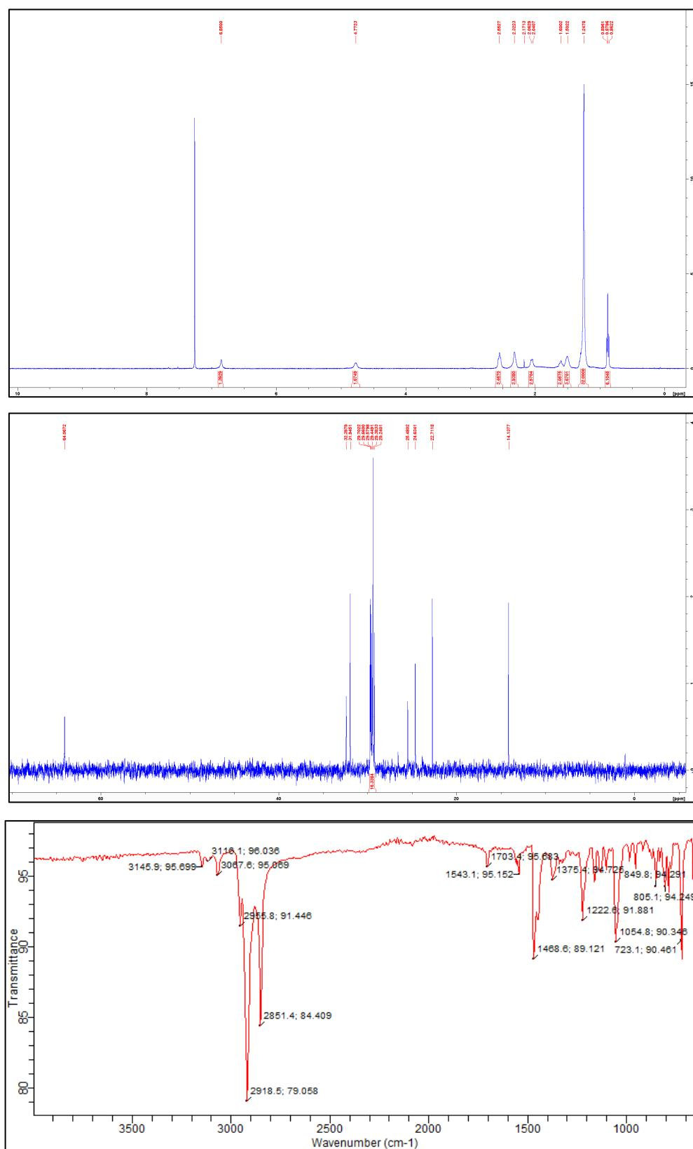
**Fig. S6** <sup>1</sup>H NMR (*top*), <sup>13</sup>C NMR (*middle*) and FT-IR (*bottom*) spectra of **click-C<sub>13</sub>-Cyc**. NMR spectra were made in CDCl<sub>3</sub>.
