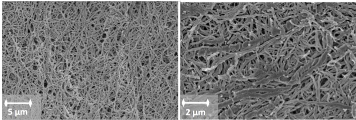
**Fig. S12** Additional FESEM pictures of a xerogel prepared from **C<sub>12</sub>-Cyc** ( $c = 30 \text{ g L}^{-1}$ ) in nitromethane.
