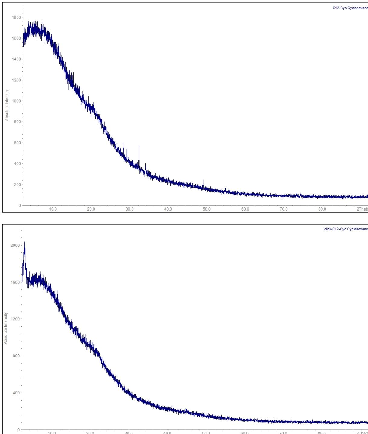
**Fig. S20** XRD spectra of **C<sub>12</sub>-Cyc** ( $c = 15 \text{ g L}^{-1}$ ) (top) and **click-C<sub>12</sub>-Cyc** ( $c = 15 \text{ g L}^{-1}$ ) (bottom) xerogels in cyclohexane.
