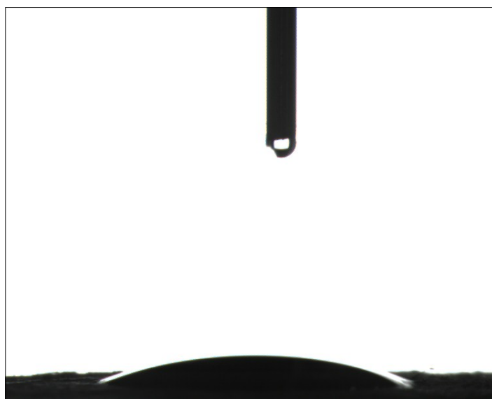
Figure S4. Water contact angle of DND at 500ms.
