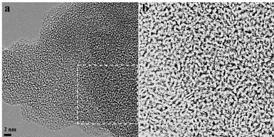
**Fig. S1.** (a) Low- and (b) high-magnification HRTEM images of prepared FeP/C catalysts.
