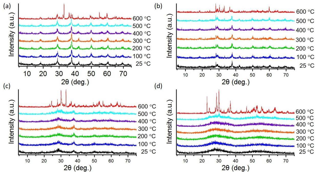
**Figure 1S:** *In situ* XRD of Nb-OMS-2 heated on an environmental cell under air: (a) 15% Nb-OMS-2 (b) 21% Nb-OMS-2 (c) 31% Nb-OMS-2 (d) 68% Nb-OMS-2
