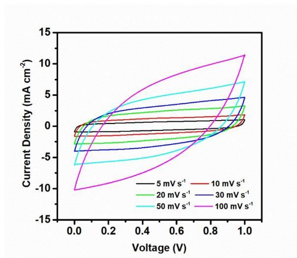
**Fig. S3.** CV curves at scan rates of 5, 10, 20, 30, 50 and 100  $\text{mV s}^{-1}$ .
