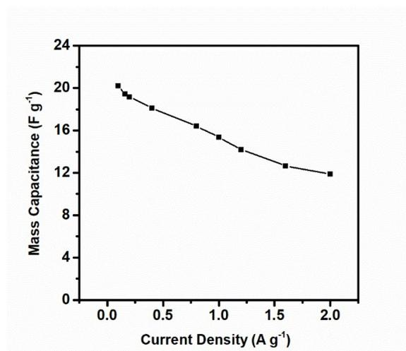
**Fig. S5.** Mass specific capacitances from GCD curves as a function of the current density.
