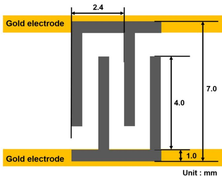
**Fig. S1.** Dimensional drawing of a single layer of the printed 3D structure (top-view).
