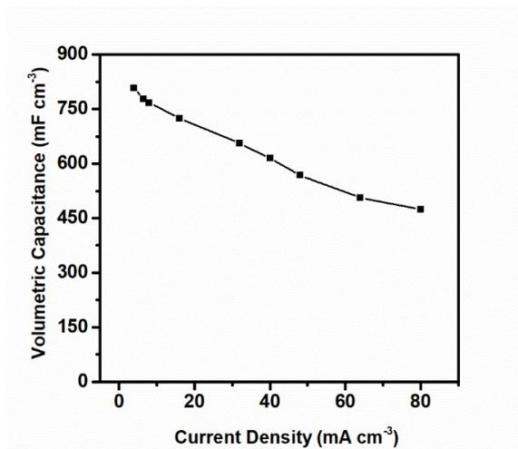
**Fig. S6.** Volumetric specific capacitances calculated from GCD curves as a function of the current density.
