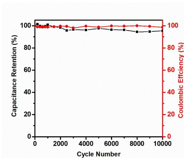
**Fig. S7.** Cycling performance and coulombic efficiency of the 3DHG-MSC at the current density of 8 mA cm<sup>-2</sup> for 10000 cycles.
