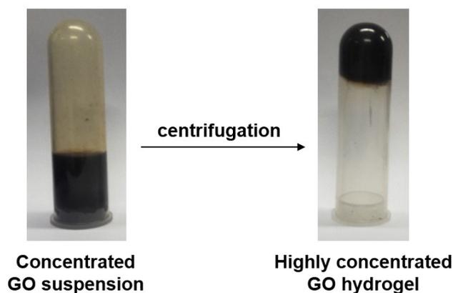
**Fig. S2.** Test tube inversion experiment of the highly concentrated GO suspension ( $17.5 \text{ mg mL}^{-1}$ ).
