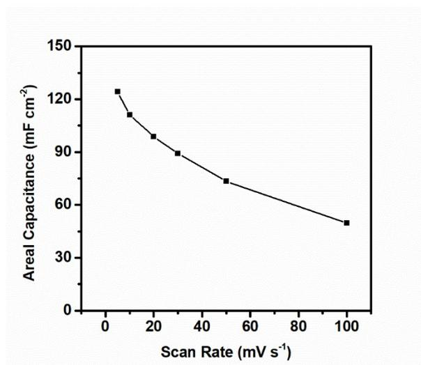
**Fig. S4.** Areal specific capacitances calculated from CV curves as a function of the scan rate.
