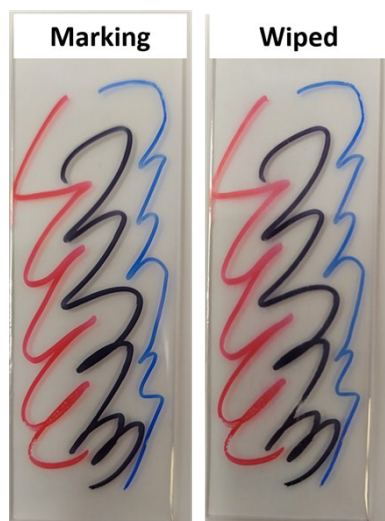
Figure S5 Anti Ink property for fully-cured PU sample treated with PDMS-NH 2 solution (PDMS in hexanes solution (5mg/mL) for 20 seconds. No anti-graffiti properties were witnessed.
