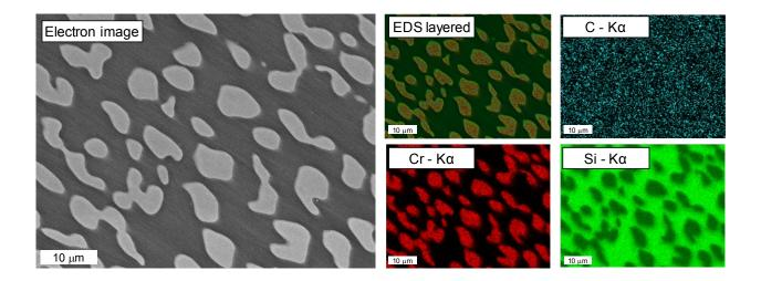
**Figure SI1.** FE–SEM image and EDS element mappings of a cross-sectioned solidified melt of 90% Si – 10% Cr. In the FE–SEM image, the bright region and dark region were found to be Cr-rich phase and Si-rich phase with EDS mapping, respectively. The distinguished Cr-rich phase enables the investigation of the melt fluid flow.
