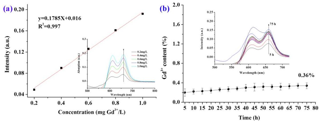
Fig. S8 The calibration curve (a) and the release of Gd<sup>3+</sup> from PVA-DPTA-Gd conjugate at different time interval (b).
