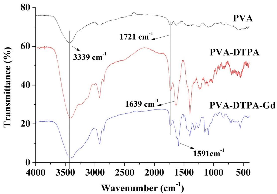
Fig. S1 FTIR spectra of PVA, PVA-DTPA and PVA-DTPA-Gd.
