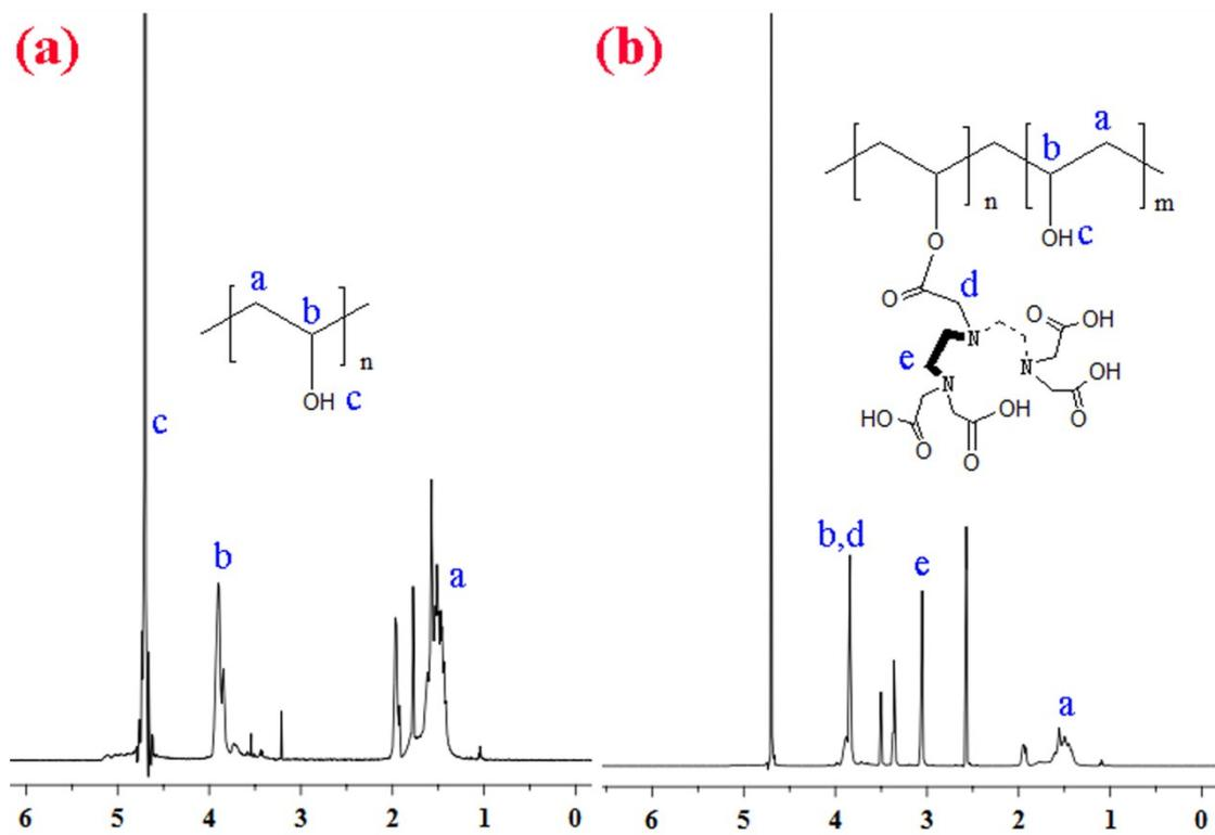
Fig. S2 NMR spectra of PVA(a) and PVA-DTPA(b).
