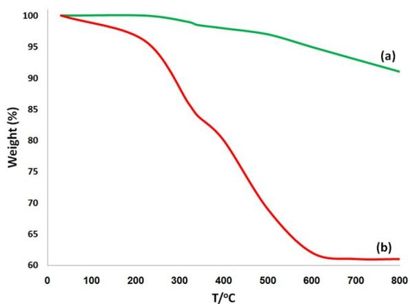
Figure S10 TGA curve of (a) raw CNTs, and (b) CNT-FeNi<sub>3</sub>/DFNS/Cu MNPs.
