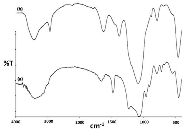
**Figure S2** FTIR spectra of (a) FeNi<sub>3</sub>/DFNS MNPs, and (b) FeNi<sub>3</sub>/DFNS/PEI MNPs.
