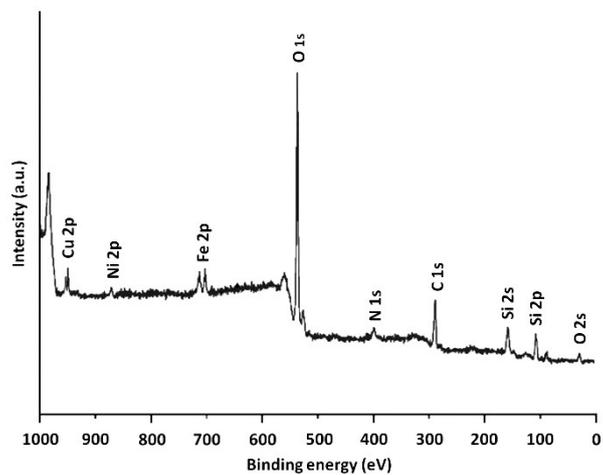
Figure S8 XPS spectra of CNT-FeNi<sub>3</sub>/DFNS/Cu MNPs.
