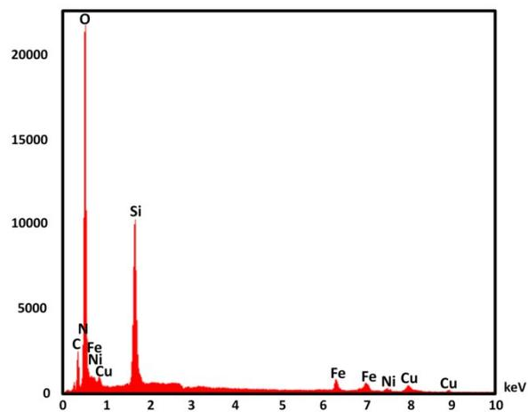
Figure S9 The EDX spectra of CNT-FeNi<sub>3</sub>/DFNS/Cu MNPs.
