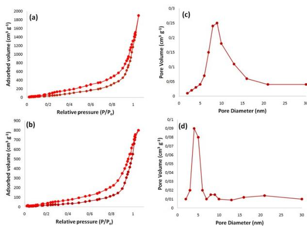
**Figure S3** adsorption-desorption isotherms of the FeNi<sub>3</sub>/DFNS NPs (a); FeNi<sub>3</sub>/DFNS/Cu (II) complexes MNPs (b); and BJH pore size distributions of the FeNi<sub>3</sub>/DFNS NPs (c); FeNi<sub>3</sub>/DFNS/Cu (II) complexes MNPs (d).
