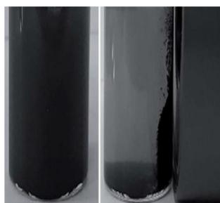
Figure S13 Catalytic separations by magnetic attraction.
