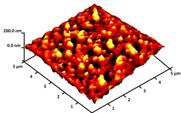
**Figure S4** Three-dimensional of AFM images of FeNi<sub>3</sub>/DFNS/Cu (II) complexes MNPs.
