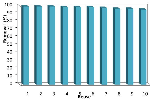
Figure S14 The reusability of catalysts for degradation of TC.
