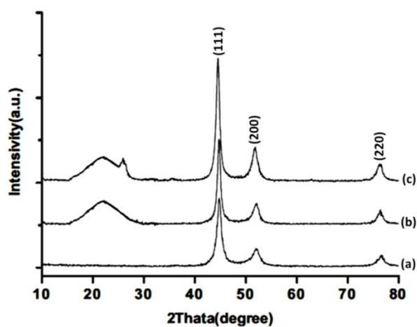
Figure S7 XRD analysis of (a) FeNi<sub>3</sub>, (b) FeNi<sub>3</sub>/DFNS/Cu (II), and (c) CNT-FeNi<sub>3</sub>/DFNS/Cu (II) complexes MNPs.
