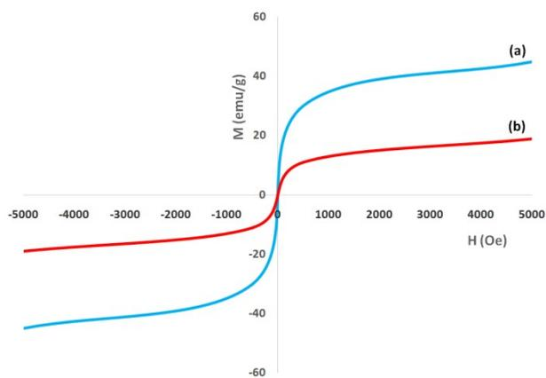
Figure S11 Room-temperature magnetization curves of (a) FeNi<sub>3</sub>/DFNS/Cu (II), and (b) CNT-FeNi<sub>3</sub>/DFNS/Cu (II) complexes MNPs.
