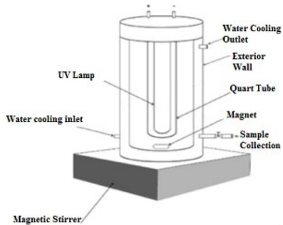
Figure S12 Schematic of the photocatalytic reactor.
