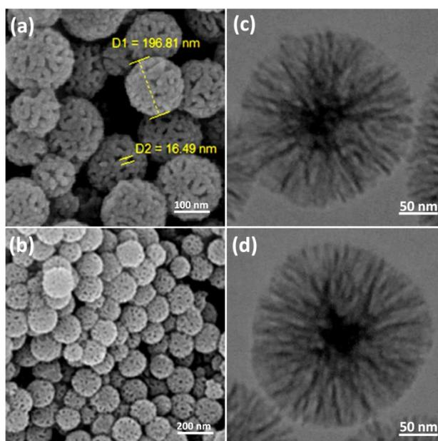
**Figure S1** TEM images of FeNi<sub>3</sub>/DFNS MNPs (a); FeNi<sub>3</sub>/DFNS/Cu (II) complexes MNPs (b); FE-SEM images of FeNi<sub>3</sub>/DFNS MNPs (c); FeNi<sub>3</sub>/DFNS/Cu (II) complexes MNPs (d).
