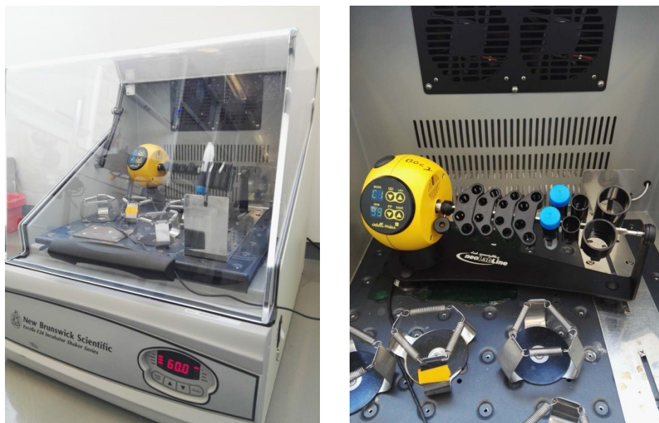
Figure S1. Picture of the reaction setup for rotating mode. Left: Whole reaction setup including the rotating machine. Right: Close-up of the rotating machine.
