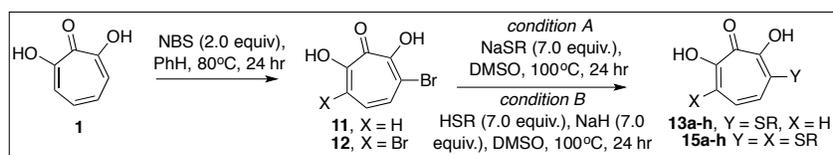
**General Procedure:** Recrystallized *N*-Bromosuccinimide (2 equiv, 1.24 mmol, 221.4 mg) was added to a solution of **1** (1 equiv, 0.62 mmol, 86.0 mg) in benzene (0.2 M, 3 mL) and stirred at 80 °C for 24 hours. After cooling the reaction mixture to room temperature, the mixture was concentrated *en vacuo* to remove benzene, which gave crude solid compounds **11** and **12** as a mixture. Without purification *condition A* or *B* was applied to obtain compounds **13a-h** and **15a-h**.
