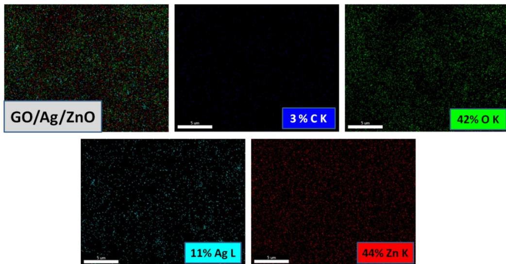
Fig S5: Elemental mapping of sample ZA-1/GO
