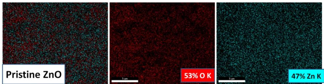
Fig S4: Elemental mapping of pristine ZnO.
