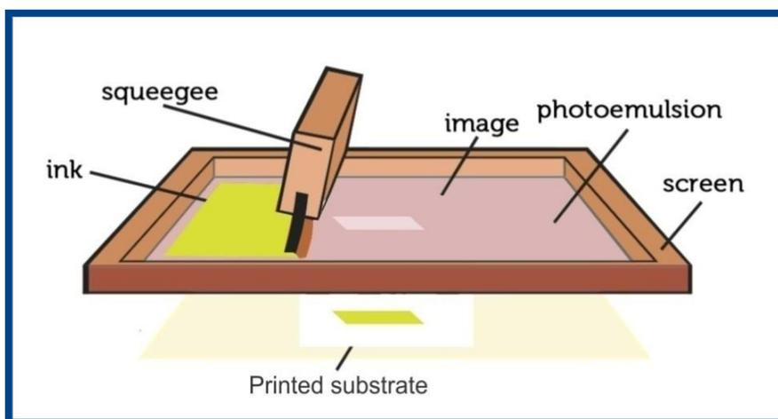
Fig S1: Schematic of screen printing technique
