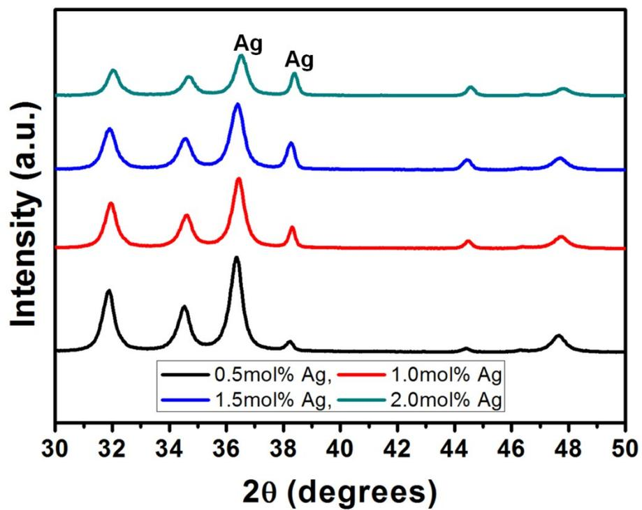
Fig S2: XRD reflections of the samples at various Ag doping
