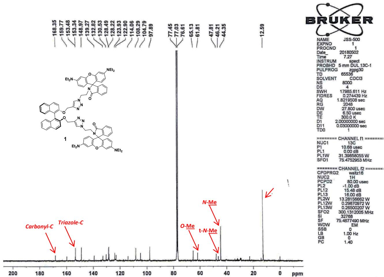
**<sup>13</sup>C NMR spectrum (75MHz, CDCl<sub>3</sub>) of dendrimer 1**
