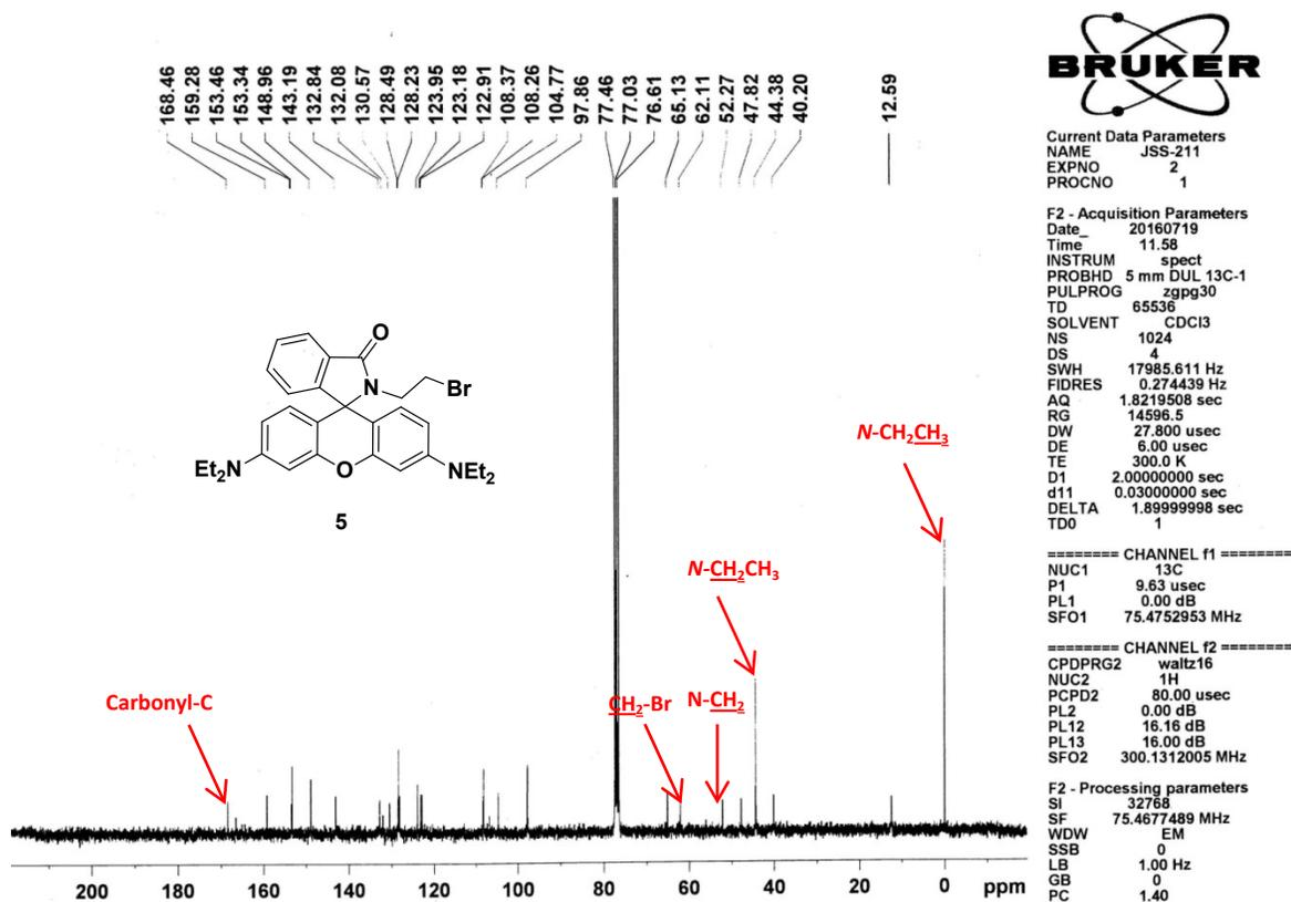
**<sup>13</sup>C NMR spectrum (75MHz, CDCl<sub>3</sub>) of rhodamine b bromo dendron 5<sup>19</sup>**
