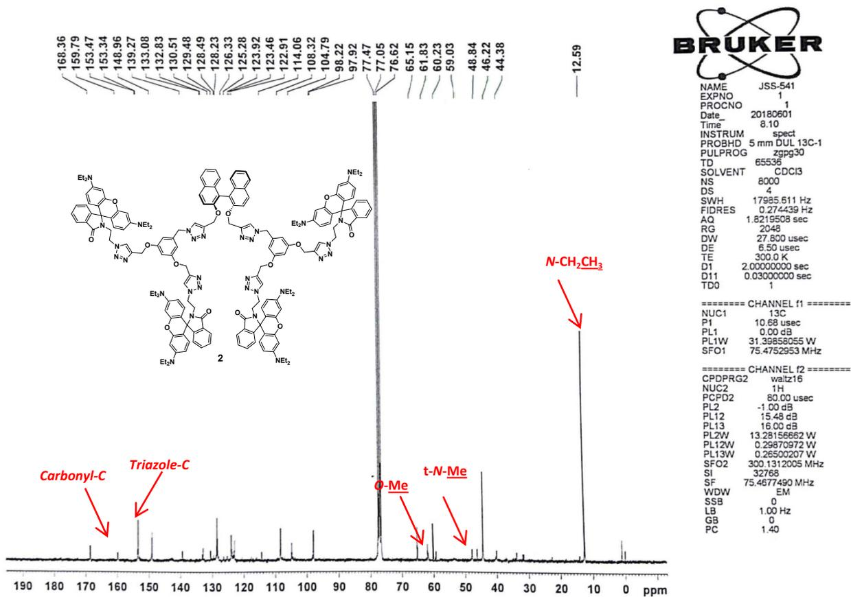
$^{13}\text{C}$  NMR spectrum (75MHz,  $\text{CDCl}_3$ ) of dendrimer 2
