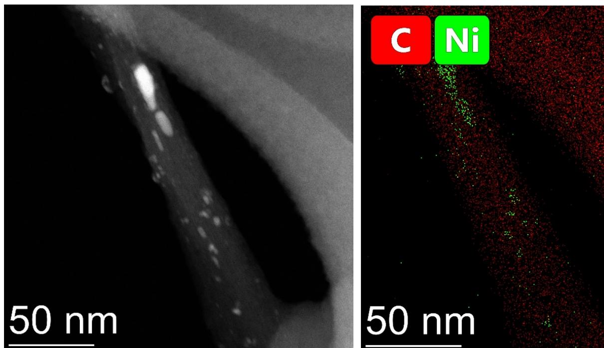
Figure S2: STEM-HAADF (High-angle annular dark-field) [Left] and EDS (energy dispersive X-ray spectroscopy) [Right] image of carbon nanotube bundles after high temperature annealing. The nickel clusters grown inside the nanotubes can be seen as bright spots on the HAADF image. The EDS map also verifies that those clusters contain Ni.
