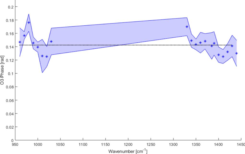
Figure S4 : O<sub>3</sub> near-field phase spectrum of a nickel cluster formed inside a single-walled carbon nanotube. The black dotted line represents the phase calculated via EFDM. The blue stars show the measured phase at different wavenumbers in our tuning range. The blue area represents the measurement error range.
