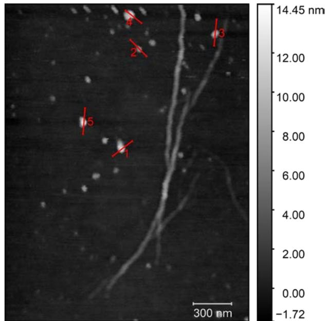
Figure S5 : AFM topography of Fig. 6 of the main text. Additional spots which appear also in contrast are measurement artifacts from dirt on the substrate.
