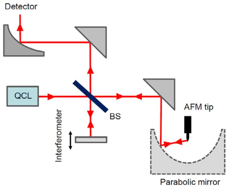
Figure S3 : Schematic presentation of the s-SNOM setup.
