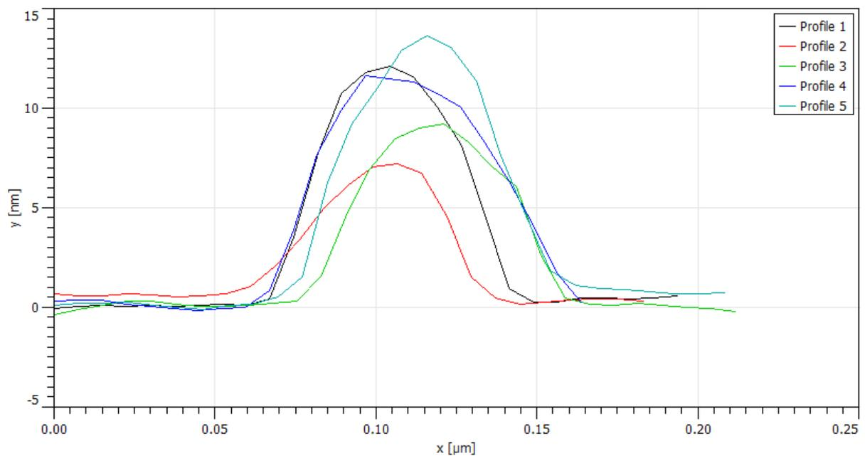
Figure S6: AFM topography profile of the spots mentioned in Fig. S5. These objects are high and provide low signal level which results in elevated noise in those areas and looks like signal contrast in low resolution images.
