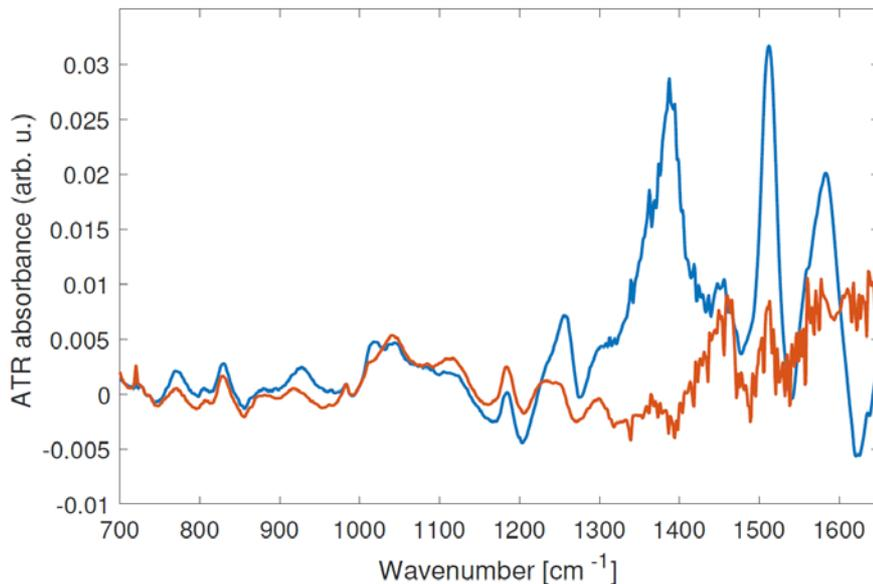
Figure S1: ATR-IR spectra of Ni-acetylacetonate-filled carbon nanotube acquired from the buckypaper sample, before (blue curve) and after (red curve) annealing. The absorption peaks of the molecules disappear as they dissociate and the remaining nickel forms clusters.
